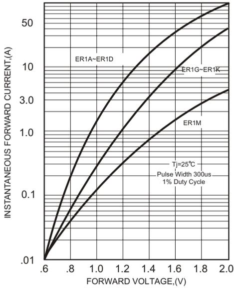
Instantaneous Forward Current - Amperes versus
