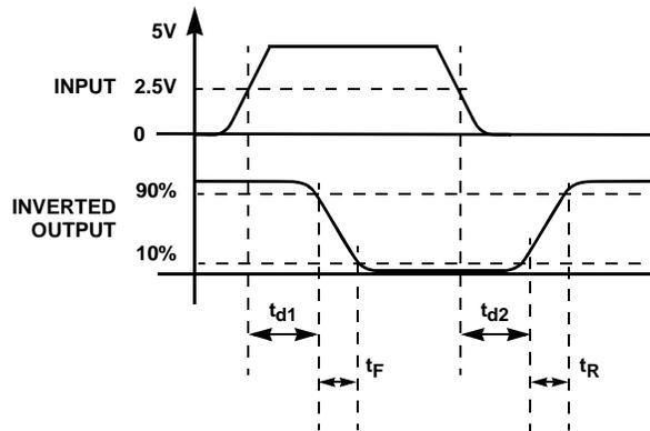
FIGURE 13. TIMING DIAGRAM
