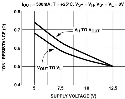
FIGURE 3. "ON"-RESISTANCE vs SUPPLY VOLTAGE ( $V_{S+}$ )
