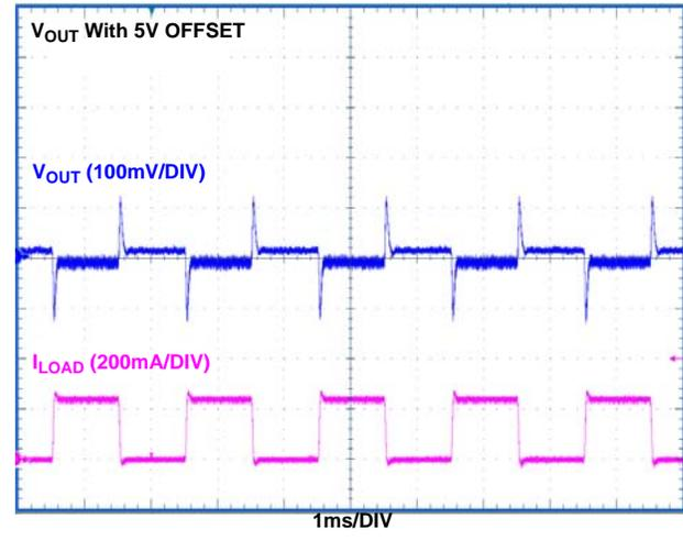
FIGURE 14. LOAD TRANSIENT RESPONSE (20mA TO 250mA)
