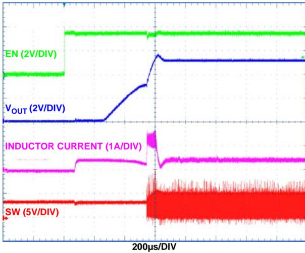
FIGURE 11. START-UP AFTER ENABLE ( $I_{LOAD} = 250mA$ )
