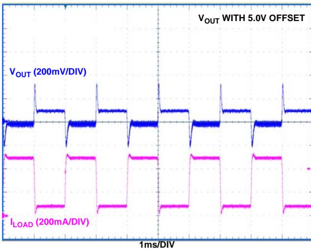
FIGURE 15. LOAD TRANSIENT RESPONSE (100mA TO 500mA)
