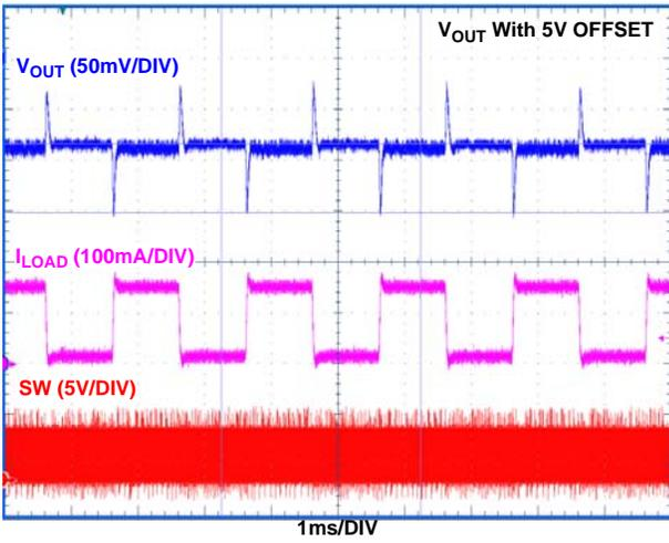
FIGURE 13. LOAD TRANSIENT RESPONSE (20mA TO 150mA)
