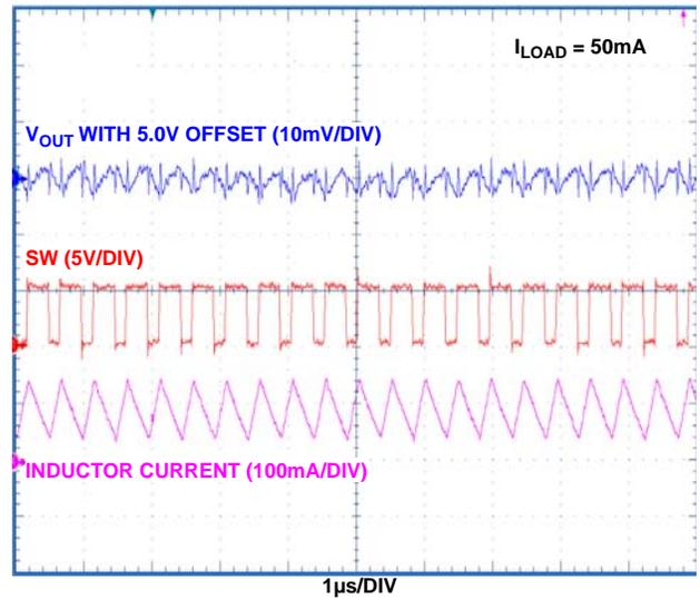
FIGURE 8. OUTPUT RIPPLE VOLTAGE ( $I_{LOAD} = 50mA$ )
