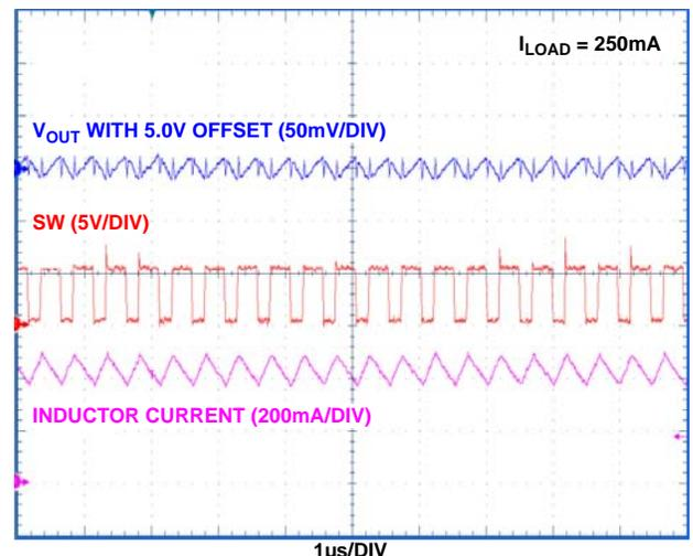
FIGURE 10. OUTPUT RIPPLE VOLTAGE ( $I_{LOAD} = 250mA$ )
