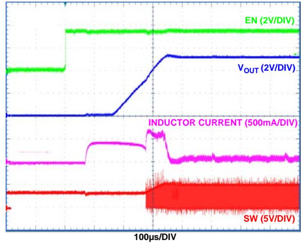
FIGURE 12. START-UP AFTER ENABLE ( $I_{LOAD} = 50mA$ )
