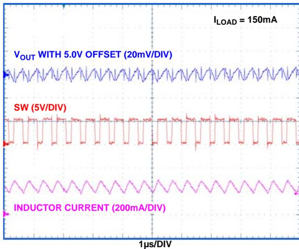
FIGURE 9. OUTPUT RIPPLE VOLTAGE ( $I_{LOAD} = 150mA$ )
