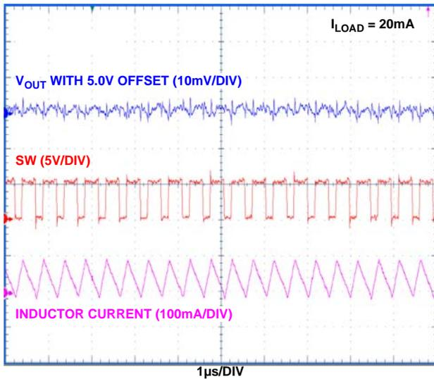
FIGURE 7. OUTPUT RIPPLE VOLTAGE ( $I_{LOAD} = 20mA$ )
