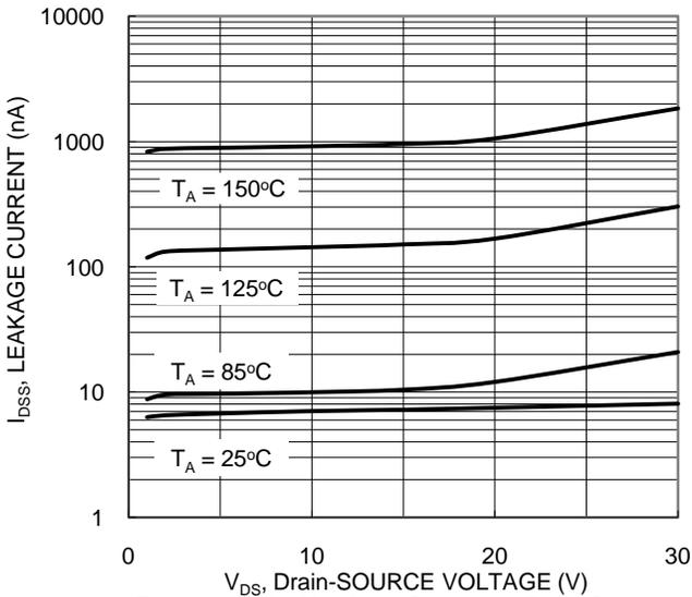
Figure 9. Typical Leakage Current vs. Drain-Source Voltage
