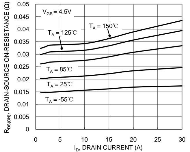
Figure 4. Typical On-Resistance vs. Drain Current and Temperature
