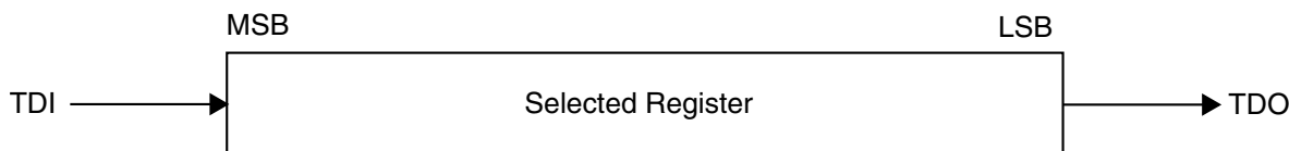
Figure 53-2. Shifting Data Through a Register
