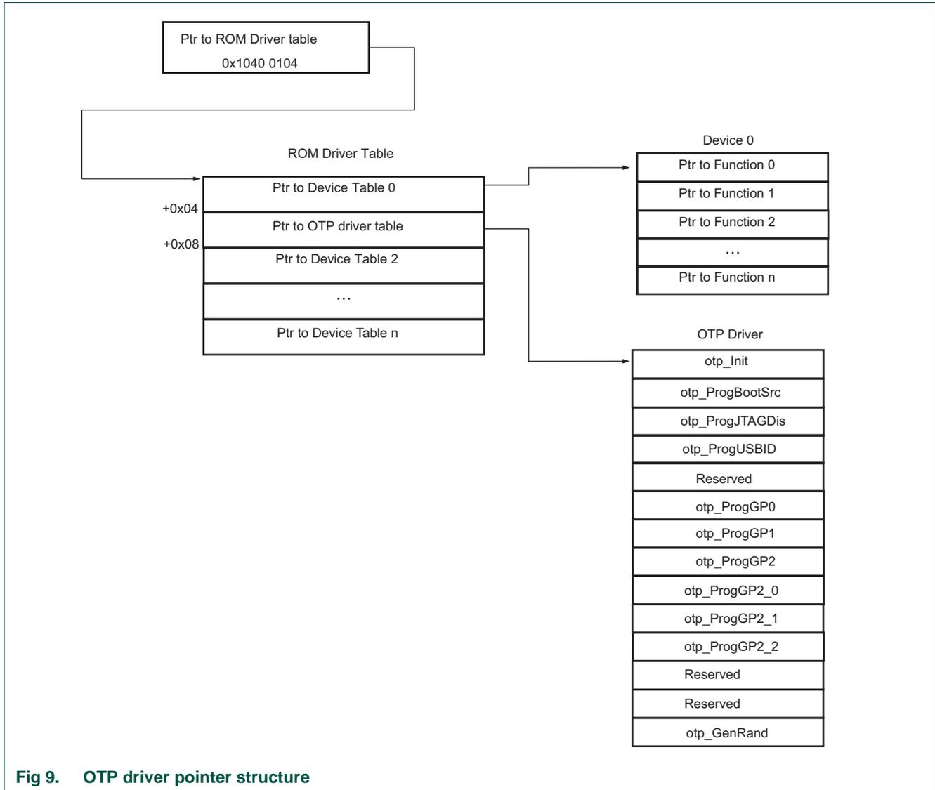
Fig 9. OTP driver pointer structure
