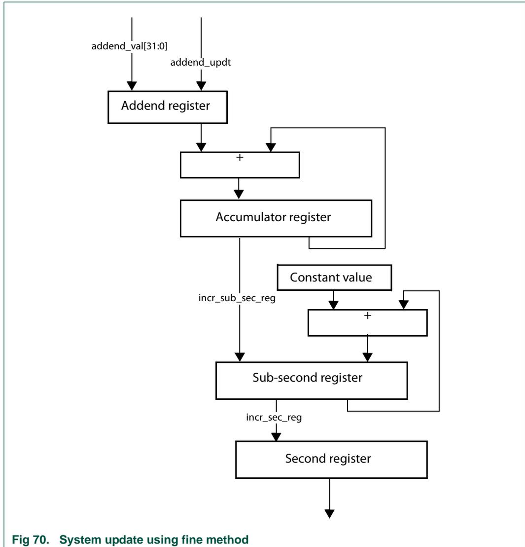
**Fig 70. System update using fine method**
