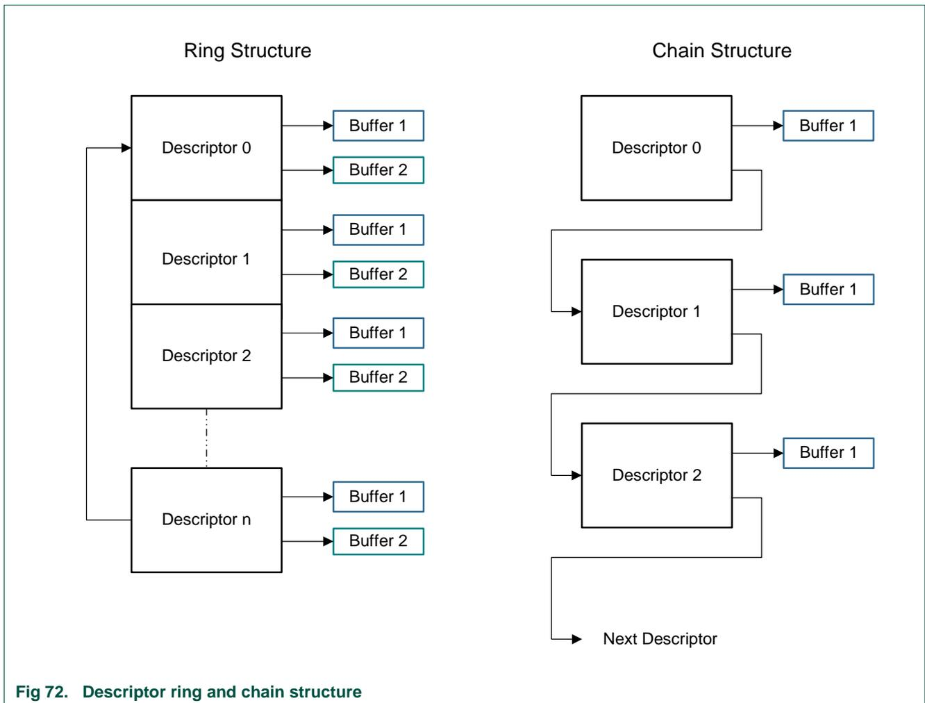
Fig 72. Descriptor ring and chain structure
