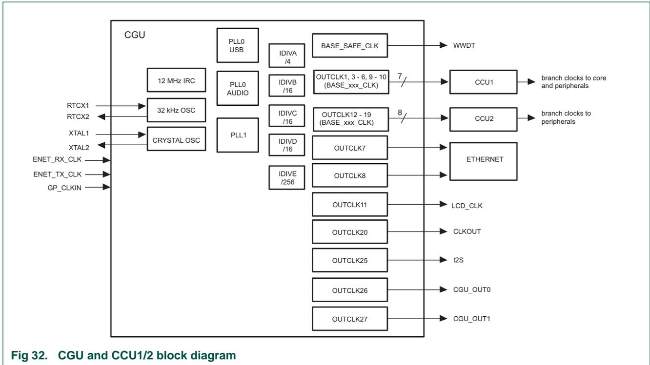
Fig 32. CGU and CCU1/2 block diagram
