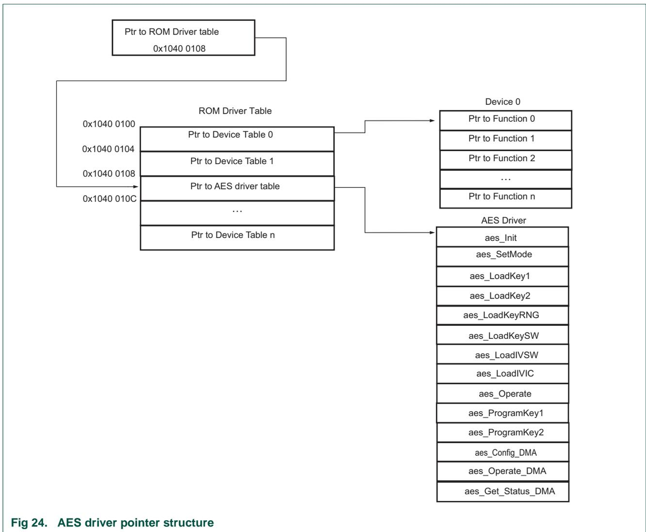
Fig 24. AES driver pointer structure
