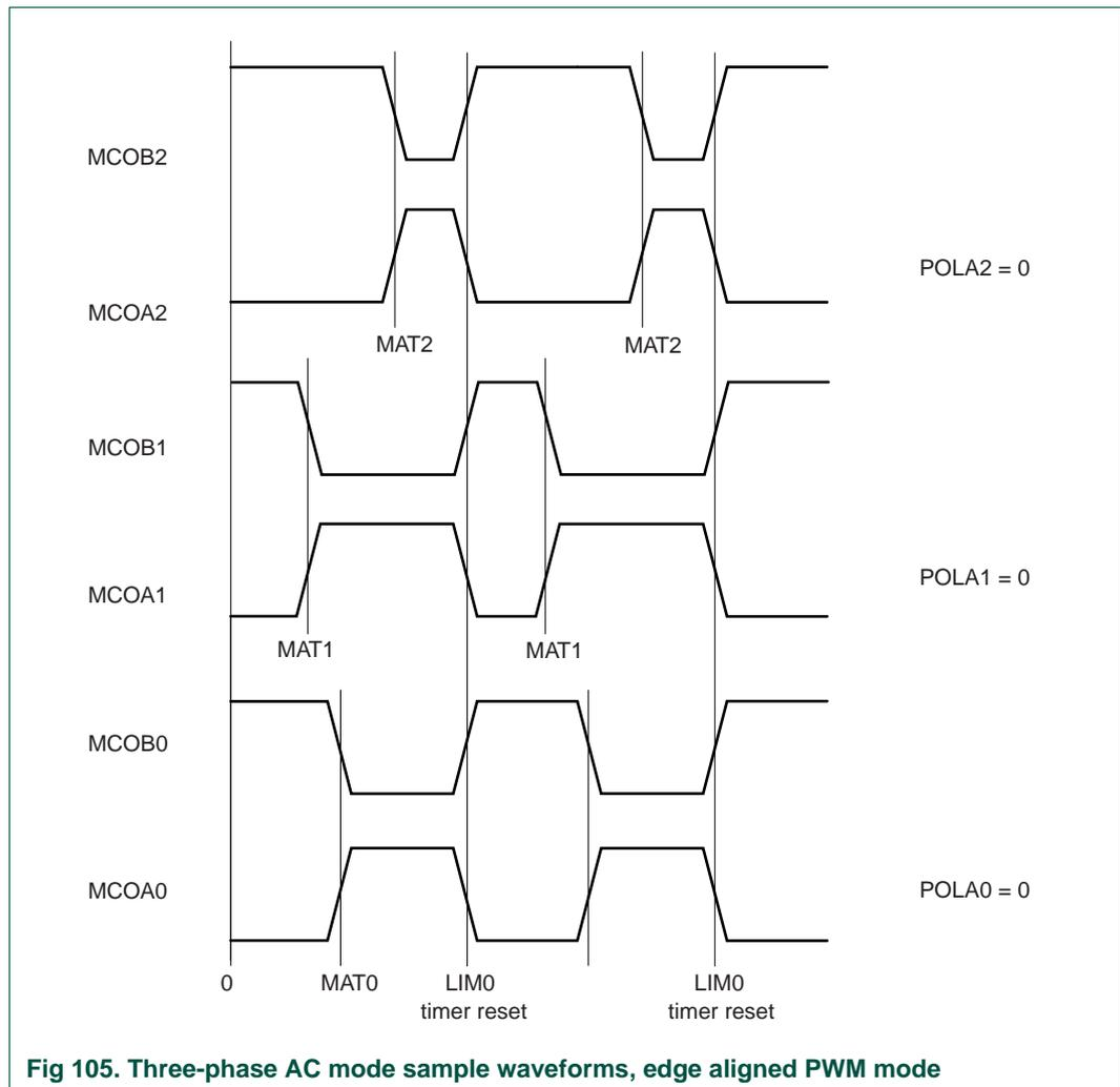
Fig 105. Three-phase AC mode sample waveforms, edge aligned PWM mode
