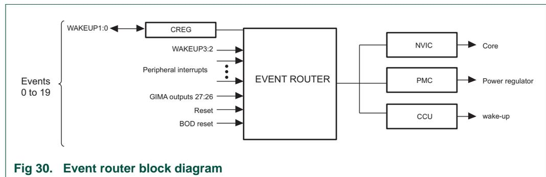
Fig 30. Event router block diagram
