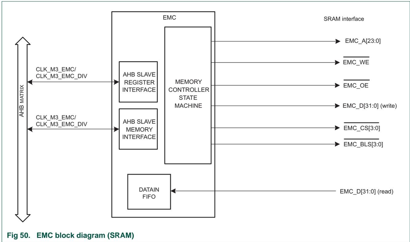
Fig 50. EMC block diagram (SRAM)
