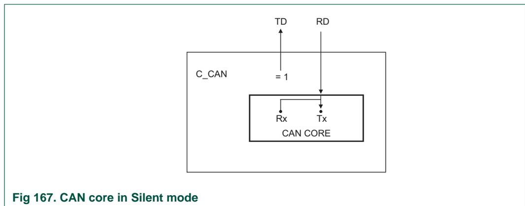
Fig 167. CAN core in Silent mode
