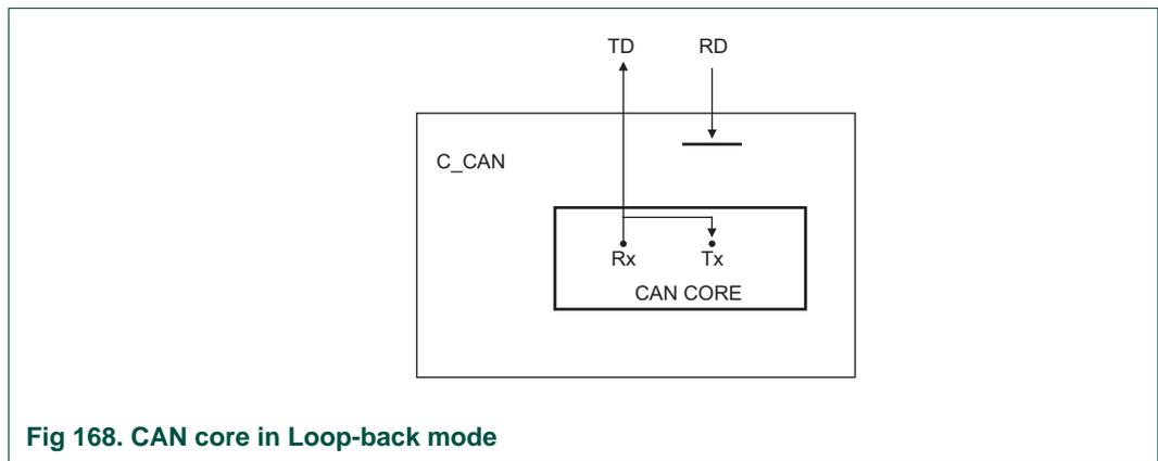
**Fig 168. CAN core in Loop-back mode**
