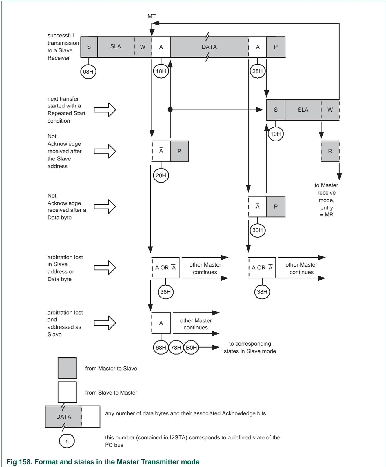
Fig 158. Format and states in the Master Transmitter mode
