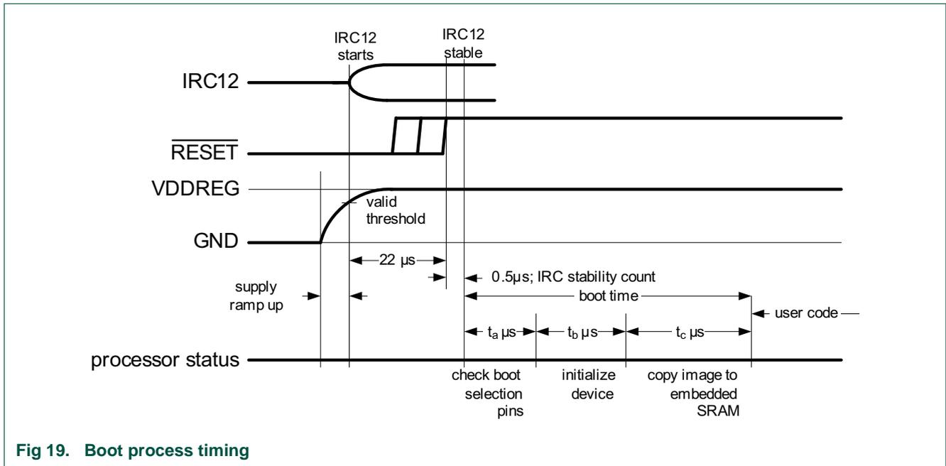
Fig 19. Boot process timing
