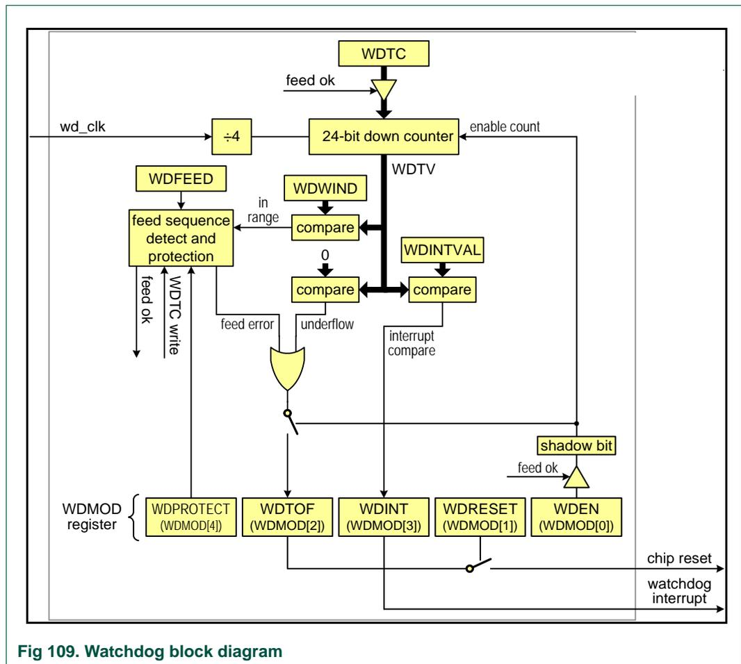
Fig 109. Watchdog block diagram
