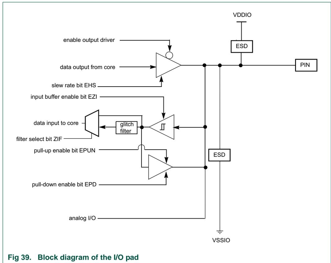
Fig 39. Block diagram of the I/O pad
