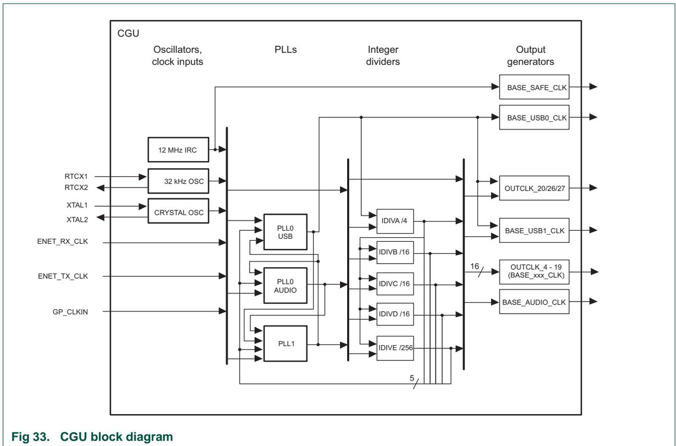
Fig 33. CGU block diagram
