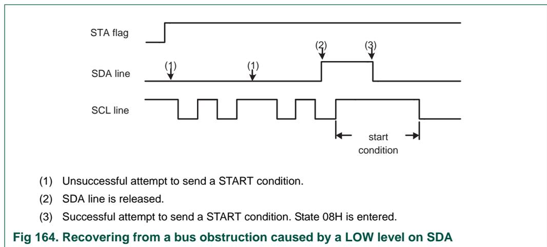
**Fig 164. Recovering from a bus obstruction caused by a LOW level on SDA**
