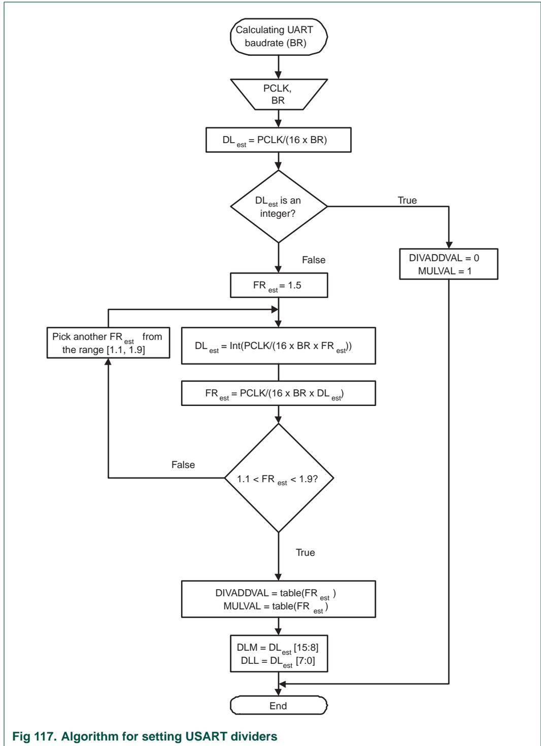
Fig 117. Algorithm for setting USART dividers
