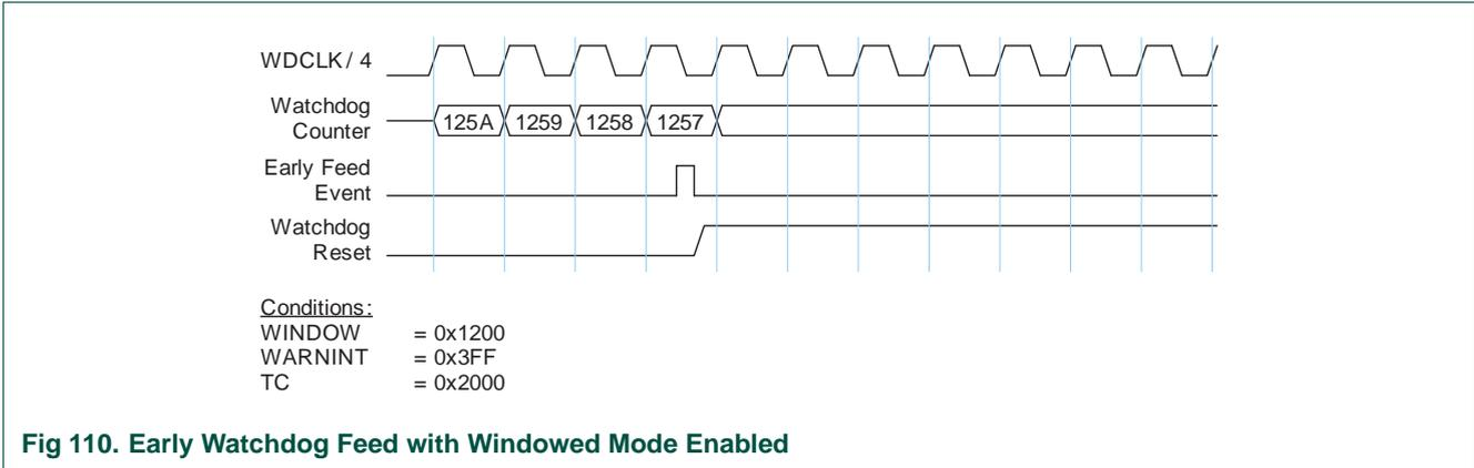
Fig 110. Early Watchdog Feed with Windowed Mode Enabled
