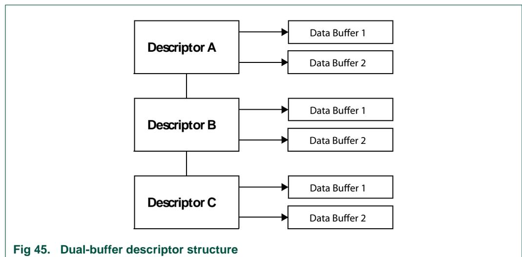
Fig 45. Dual-buffer descriptor structure
