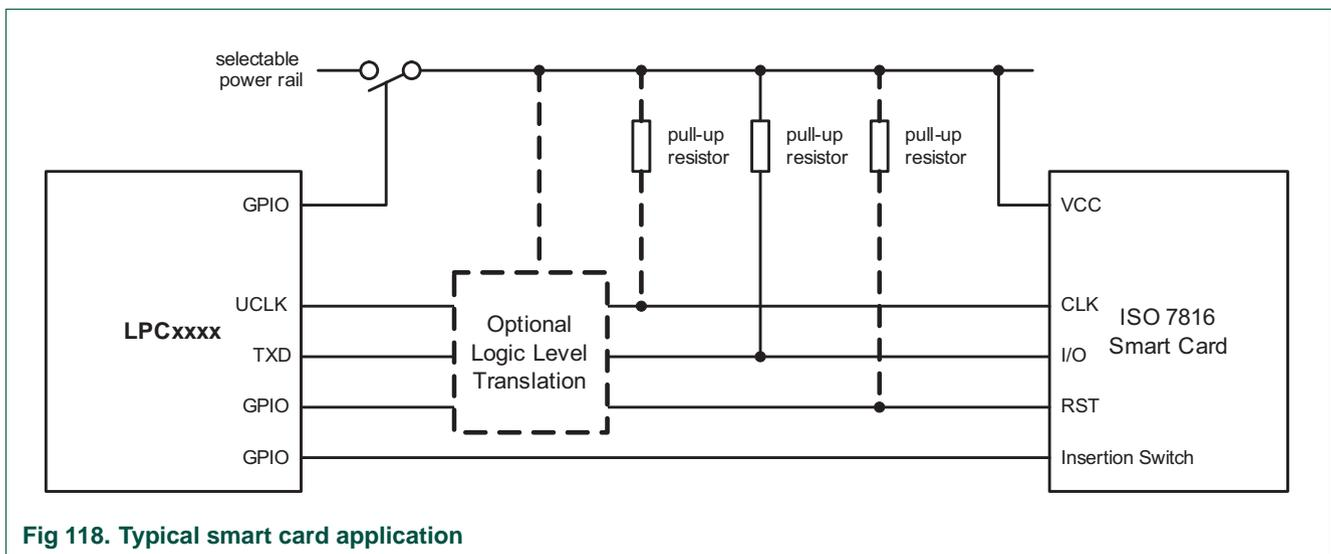
Fig 118. Typical smart card application
