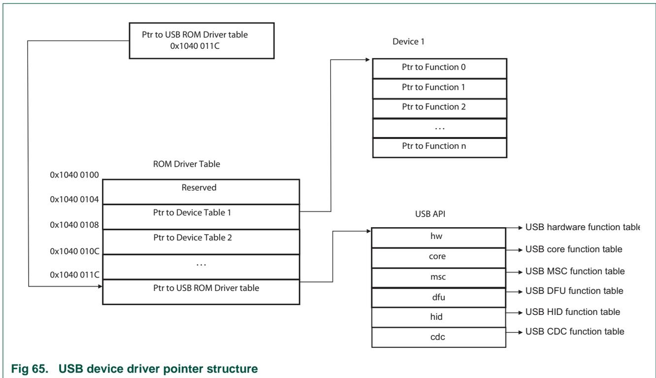
Fig 65. USB device driver pointer structure
