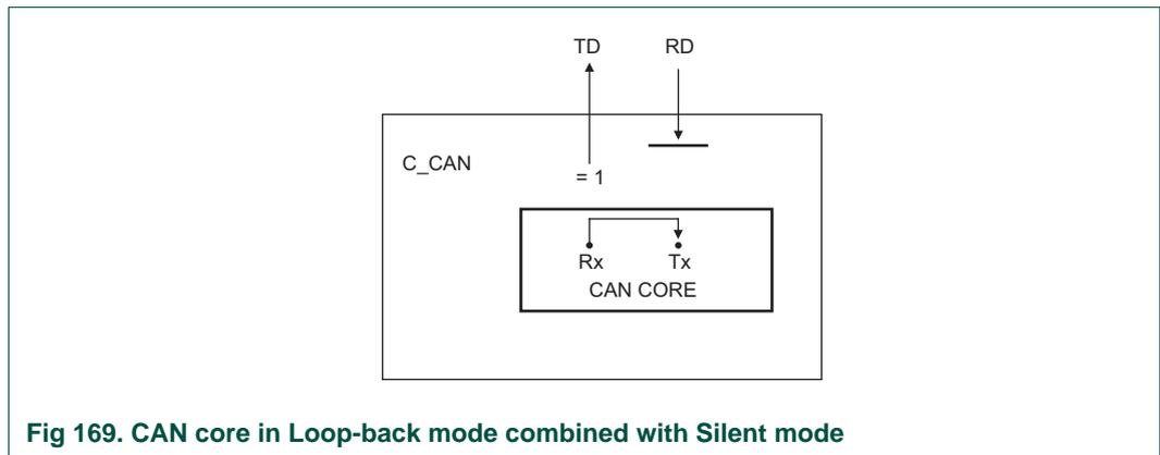
**Fig 169. CAN core in Loop-back mode combined with Silent mode**
