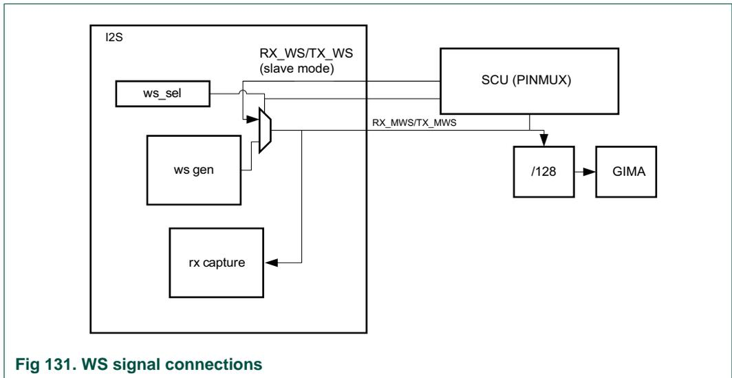
Fig 131. WS signal connections
