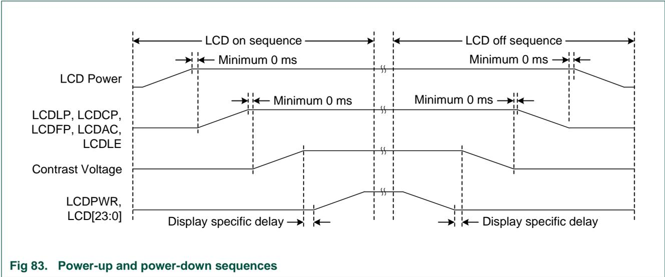
Fig 83. Power-up and power-down sequences
