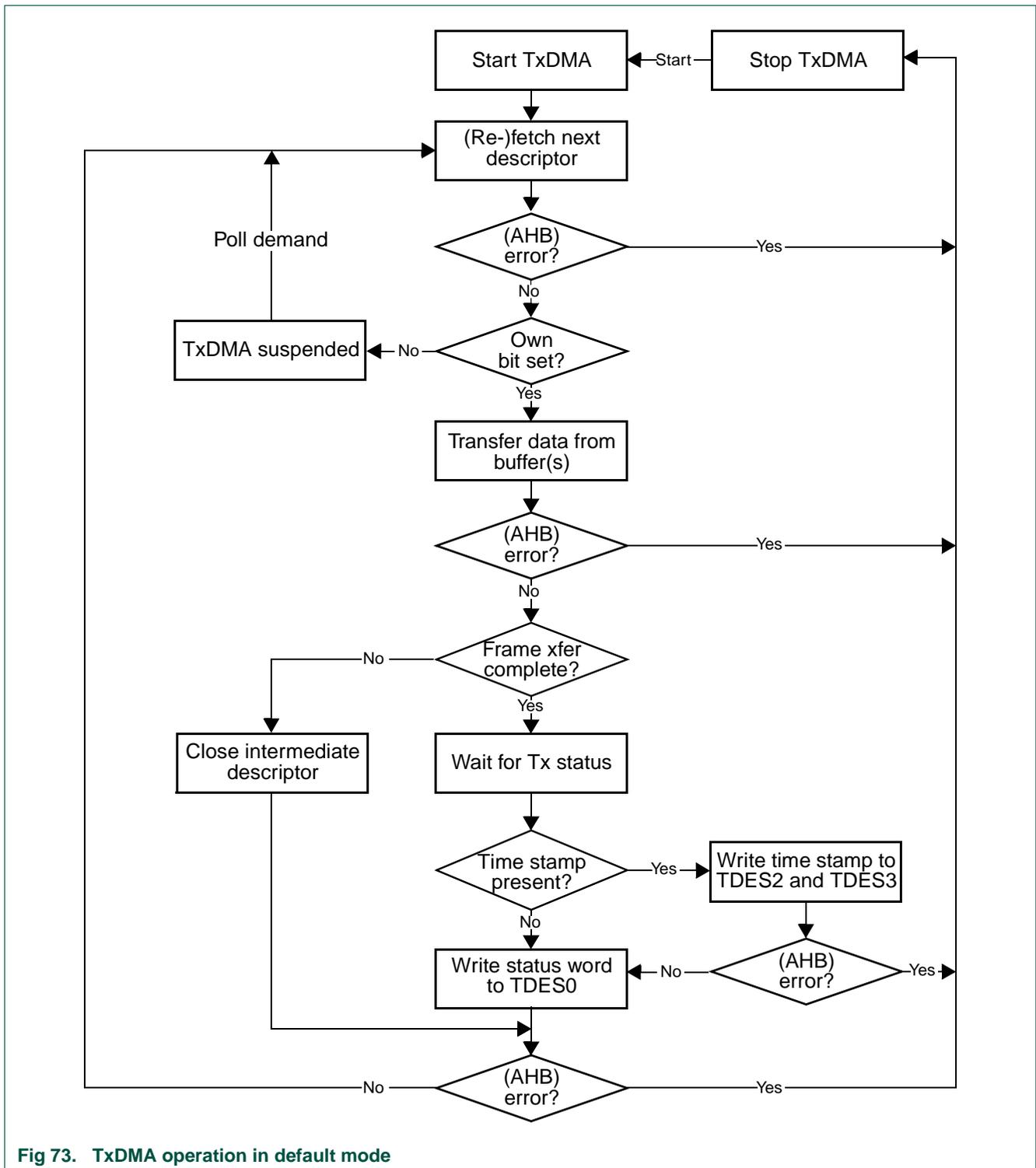
Fig 73. TxDMA operation in default mode
