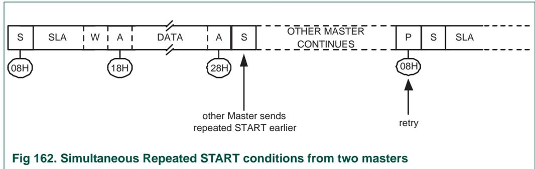
Fig 162. Simultaneous Repeated START conditions from two masters
