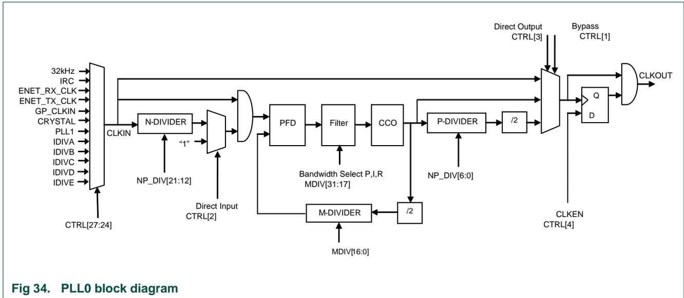
Fig 34. PLL0 block diagram
