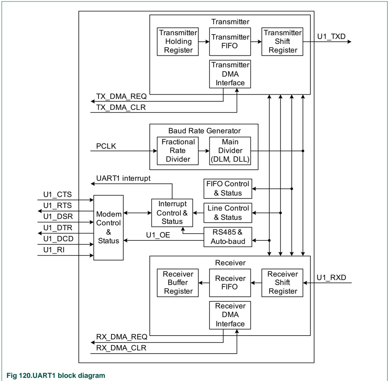
Fig 120. UART1 block diagram
