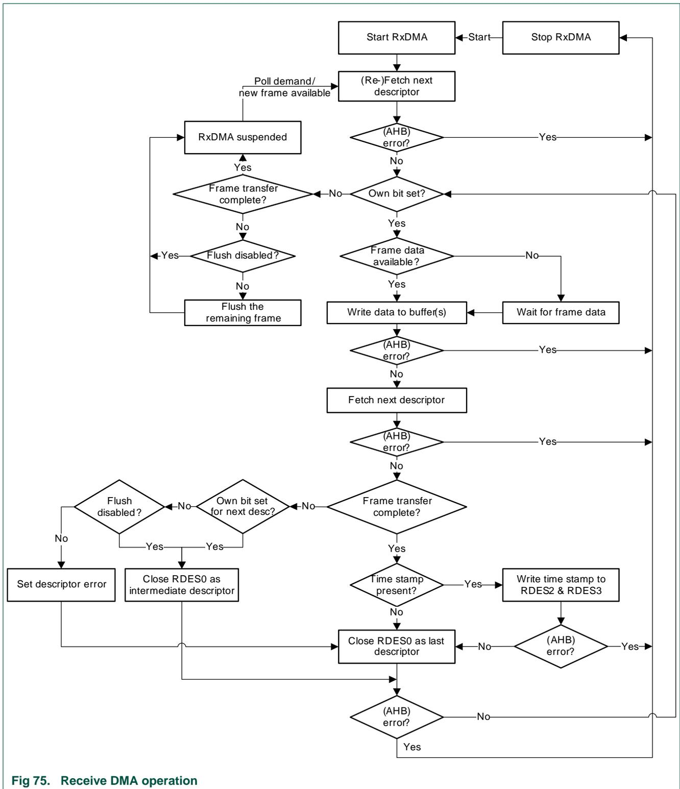
Fig 75. Receive DMA operation
