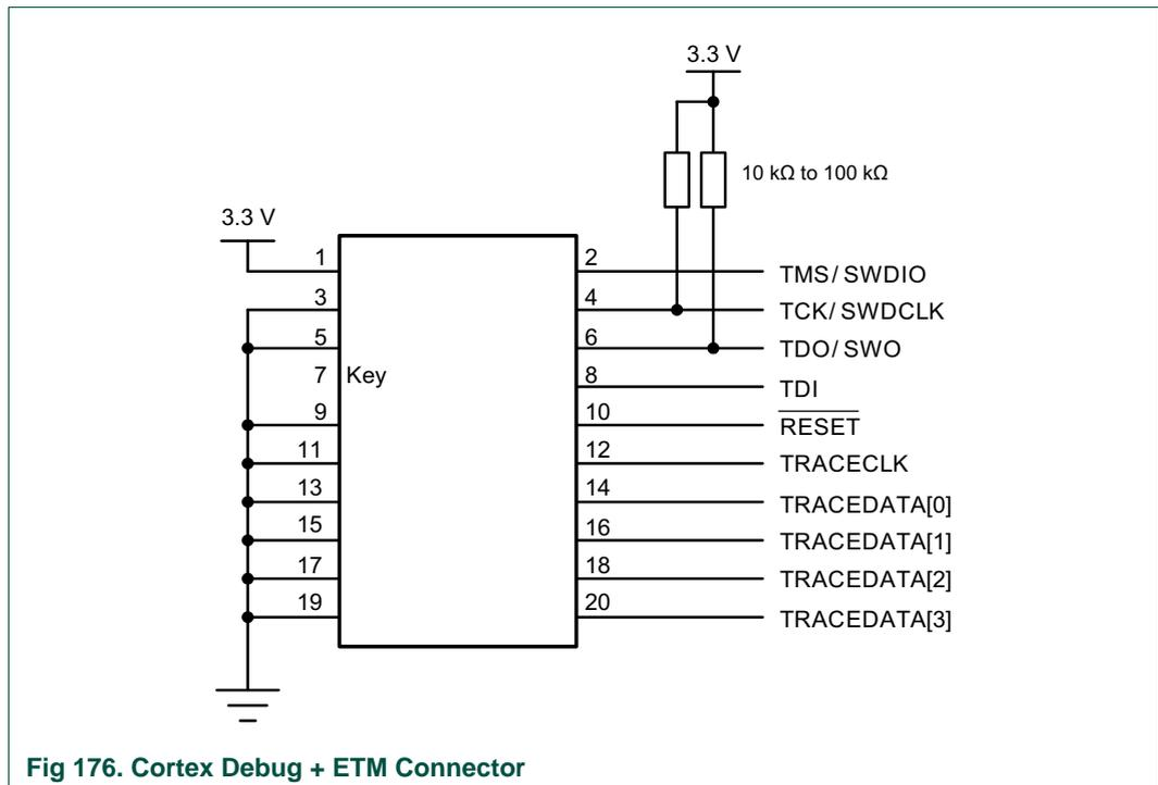
Fig 176. Cortex Debug + ETM Connector
