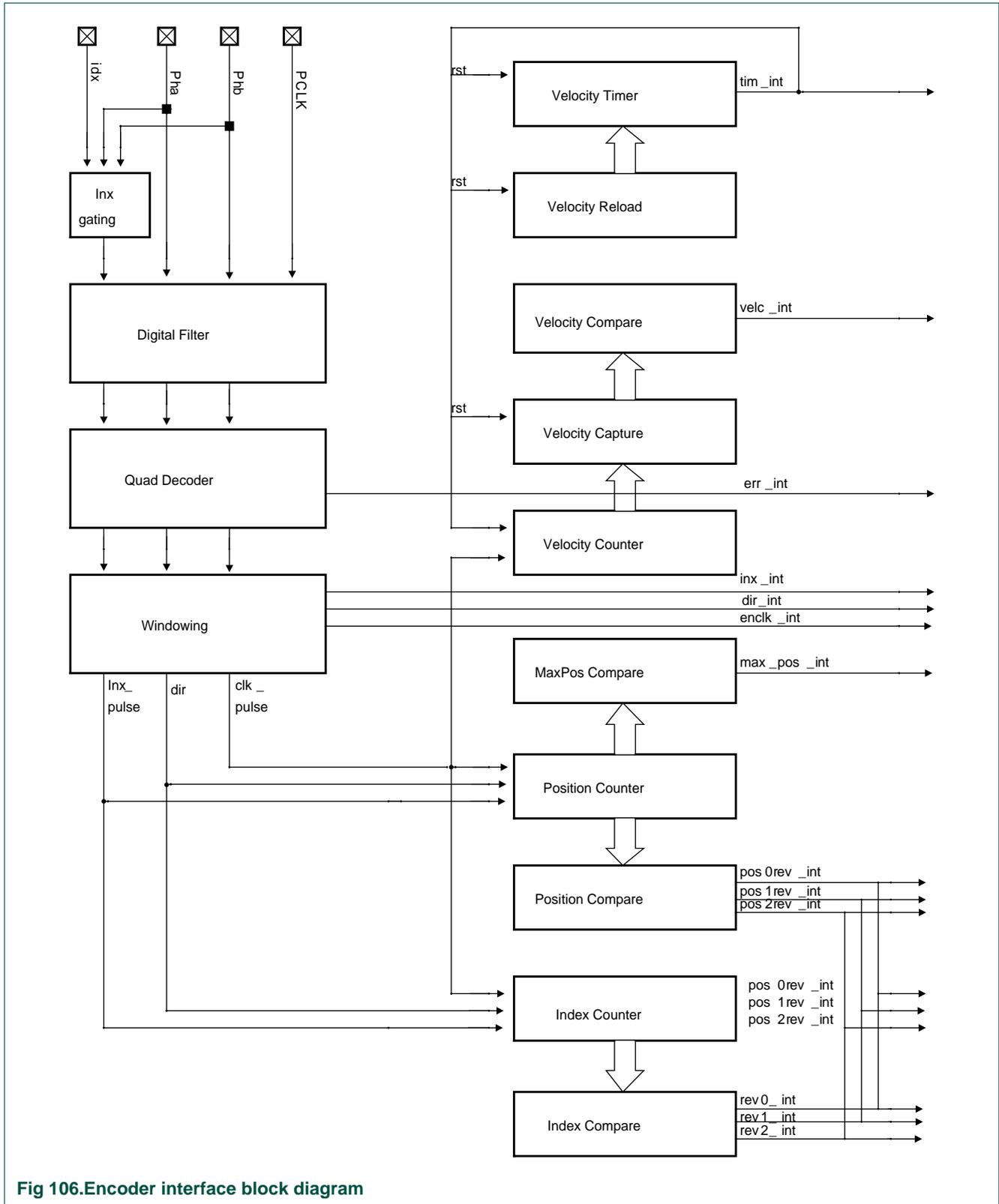
Fig 106.Encoder interface block diagram
