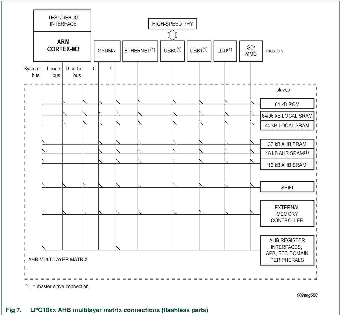
Fig 7. LPC18xx AHB multilayer matrix connections (flashless parts)
