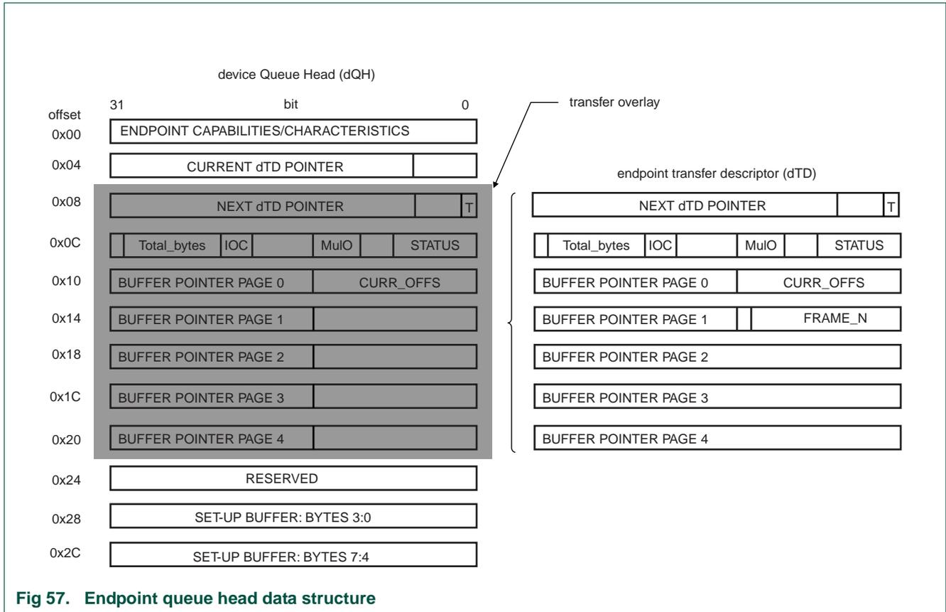
Fig 57. Endpoint queue head data structure
