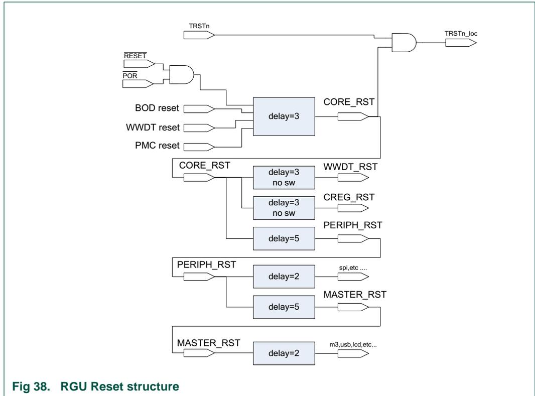
Fig 38. RGU Reset structure
