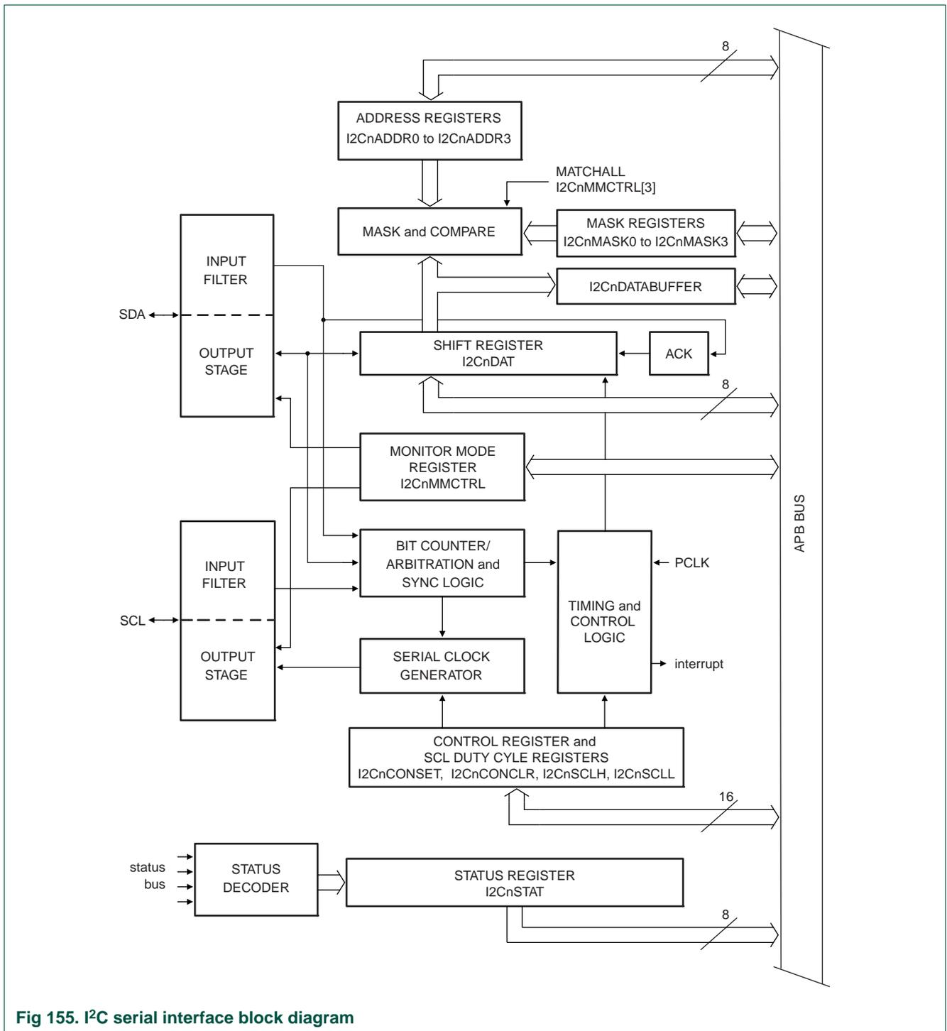
Fig 155. I<sup>2</sup>C serial interface block diagram
