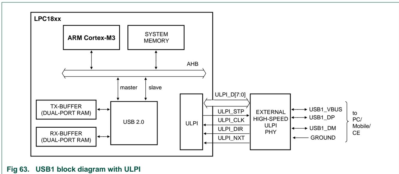
Fig 63. USB1 block diagram with ULPI
