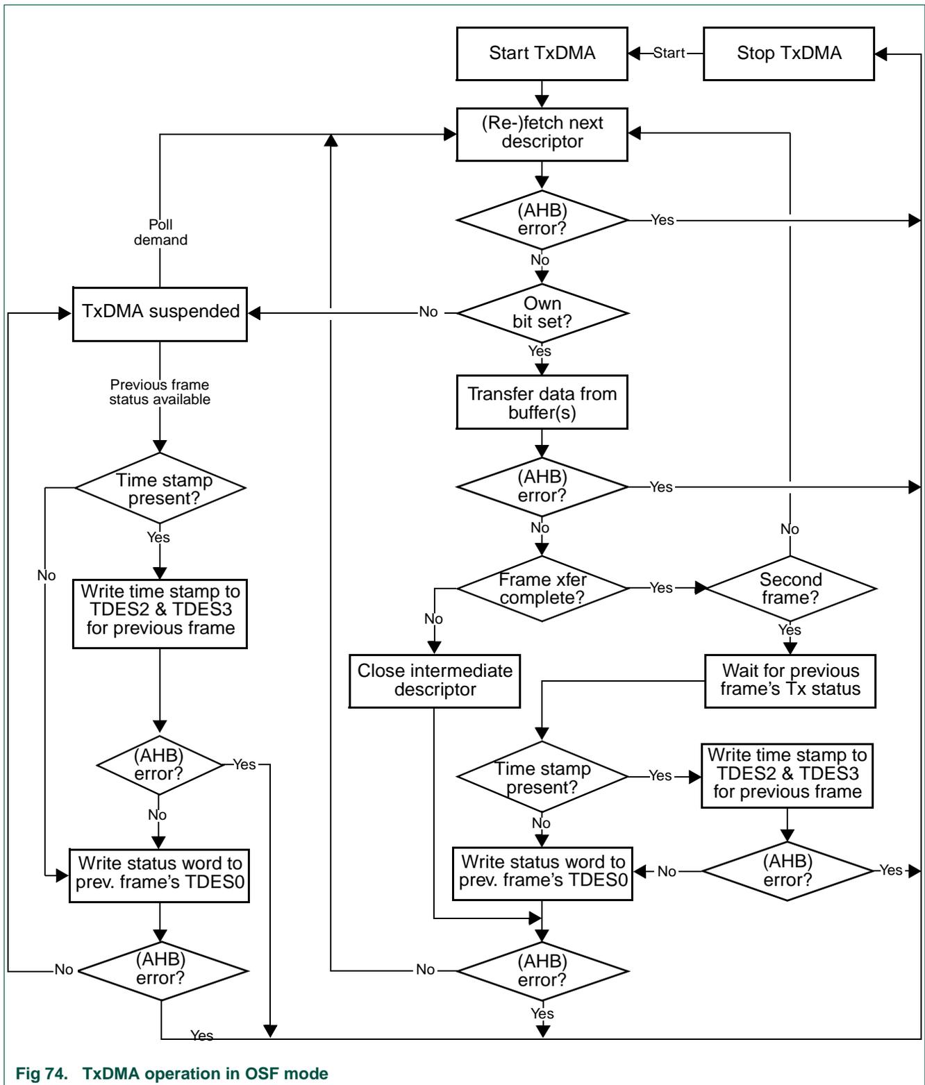
Fig 74. TxDMA operation in OSF mode
