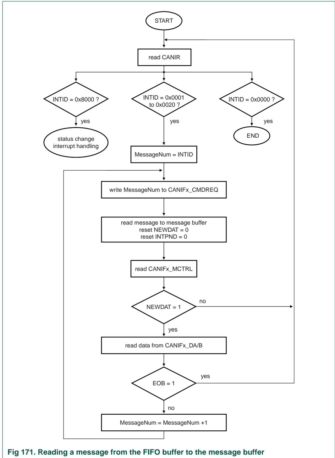
Fig 171. Reading a message from the FIFO buffer to the message buffer
