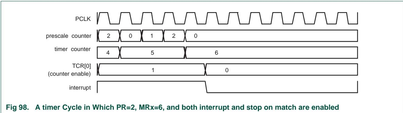
Fig 98. A timer Cycle in Which PR=2, MRx=6, and both interrupt and stop on match are enabled
