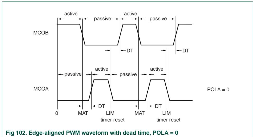
Fig 102. Edge-aligned PWM waveform with dead time, POLA = 0
