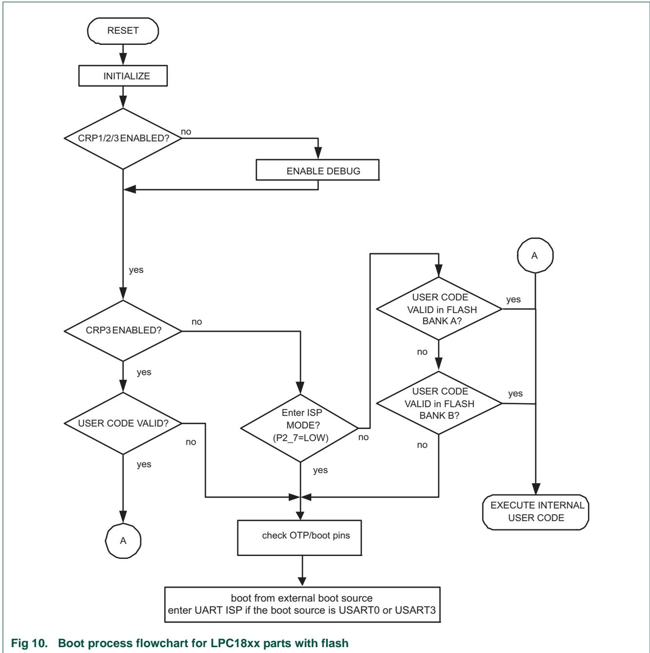
Fig 10. Boot process flowchart for LPC18xx parts with flash
