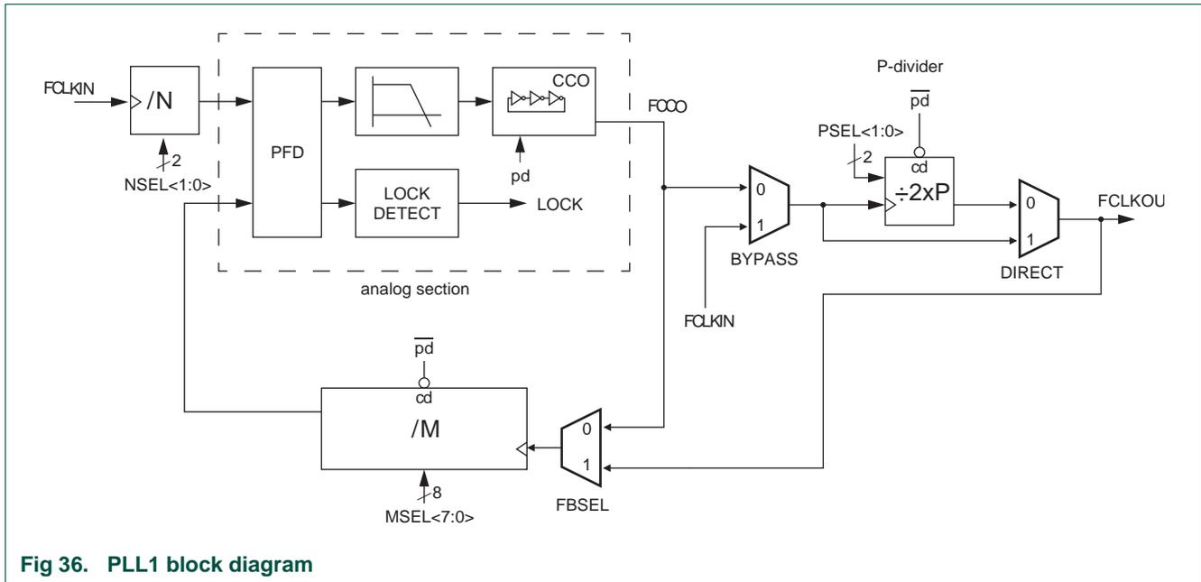
Fig 36. PLL1 block diagram
