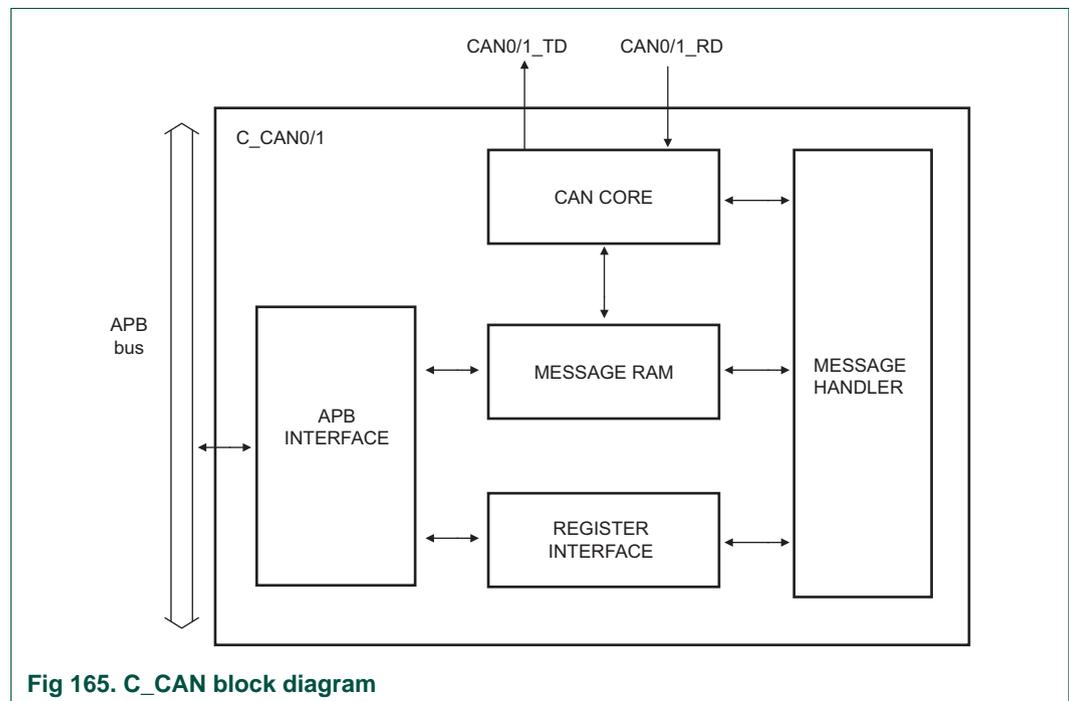
Fig 165. C\_CAN block diagram
