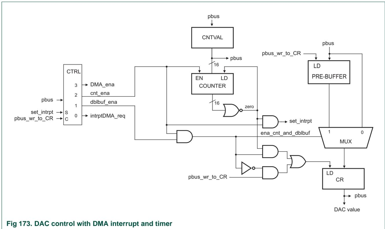
Fig 173. DAC control with DMA interrupt and timer
