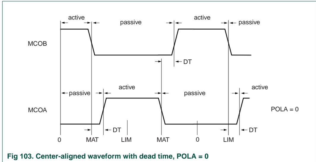
Fig 103. Center-aligned waveform with dead time, POLA = 0
