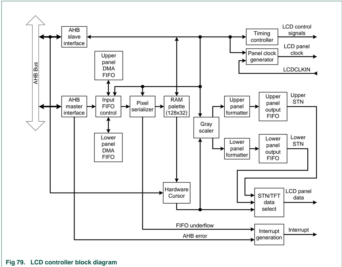
Fig 79. LCD controller block diagram
