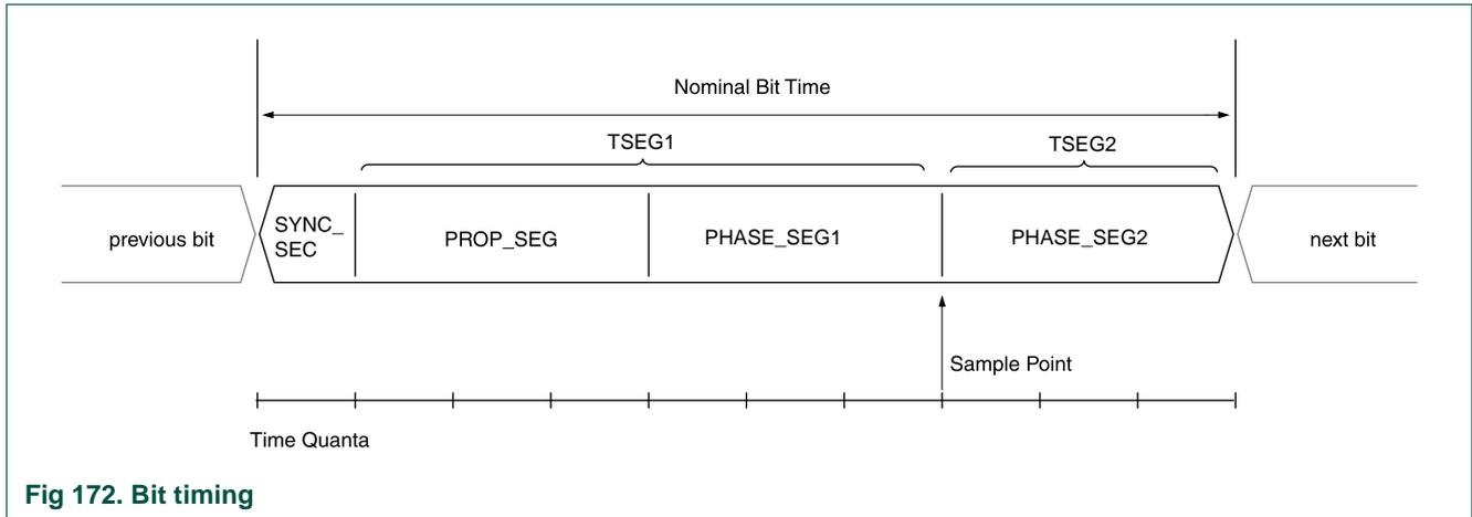
Fig 172. Bit timing
