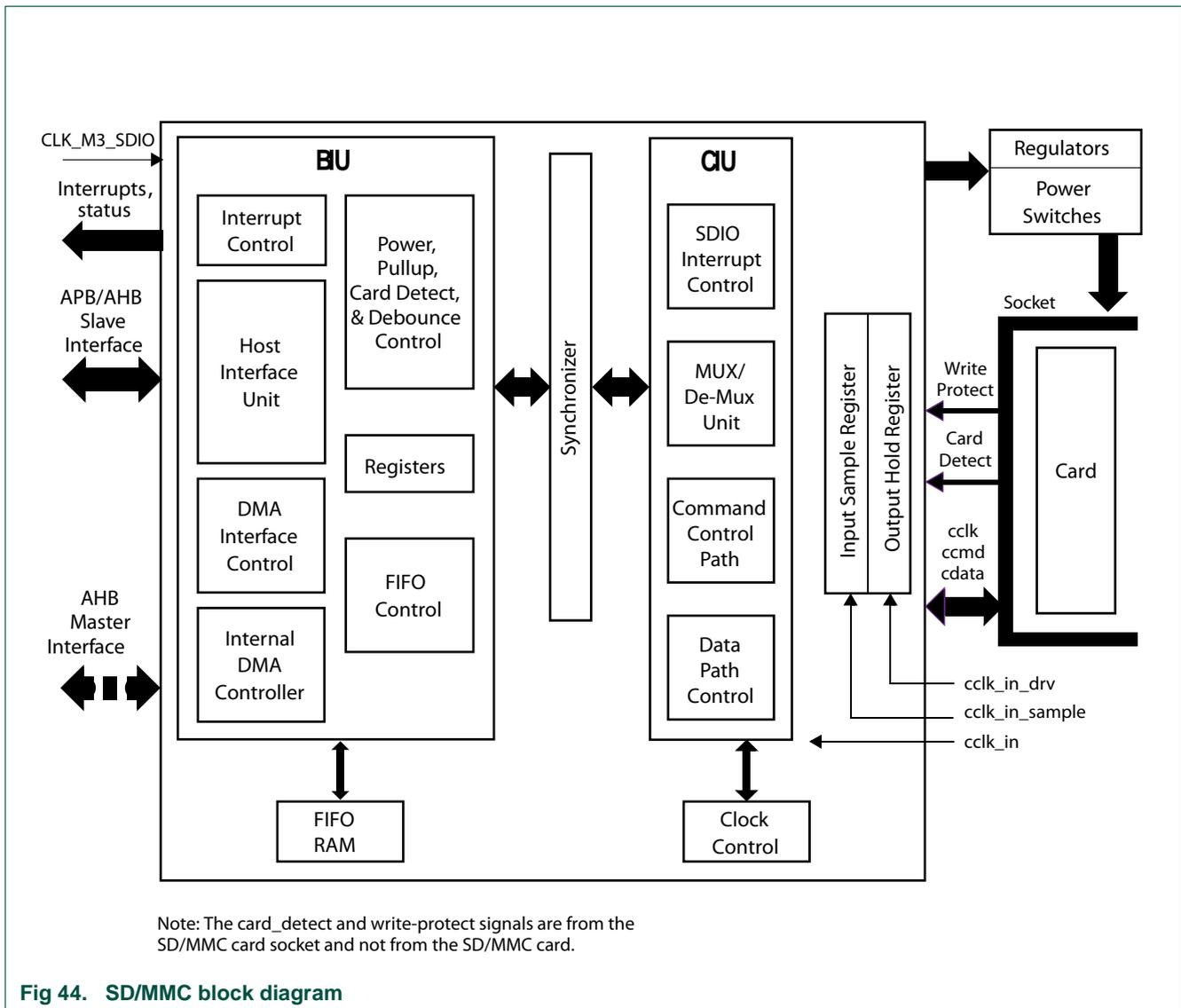
Fig 44. SD/MMC block diagram
