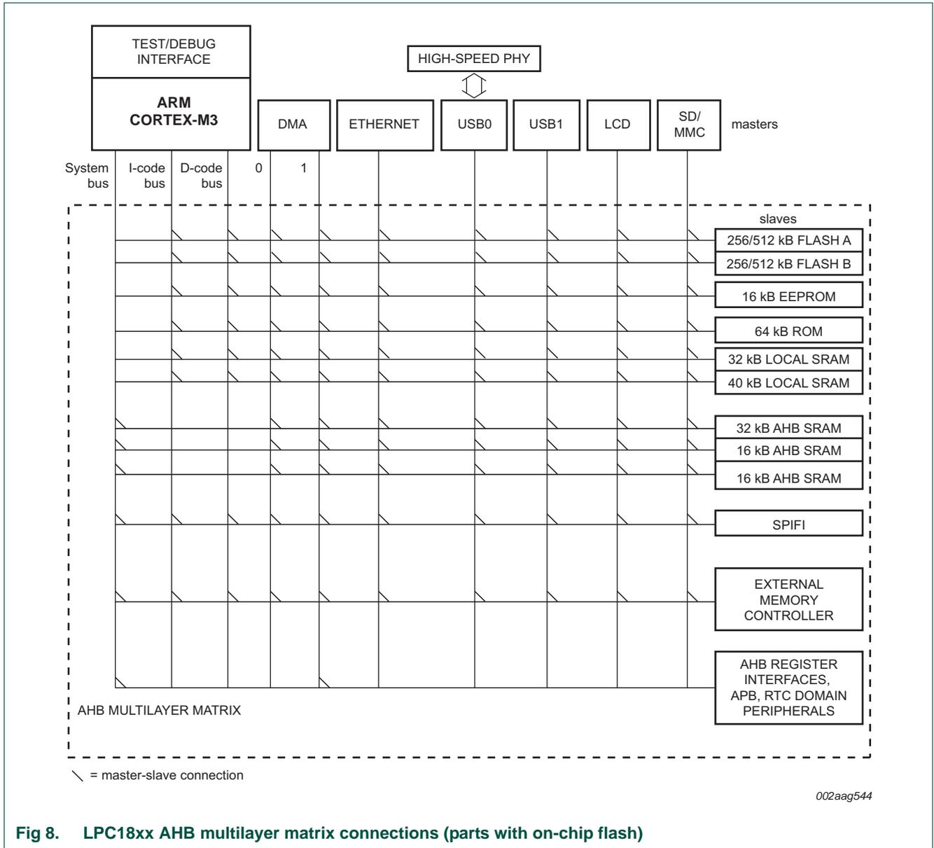
Fig 8. LPC18xx AHB multilayer matrix connections (parts with on-chip flash)
