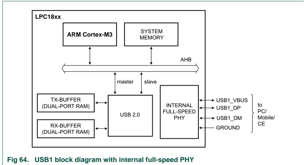
Fig 64. USB1 block diagram with internal full-speed PHY
