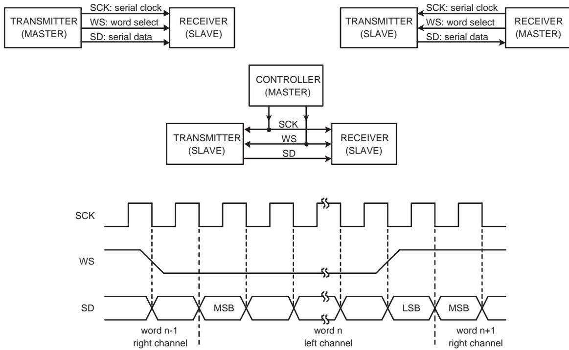
Fig 132. Simple I2S configurations and bus timing
