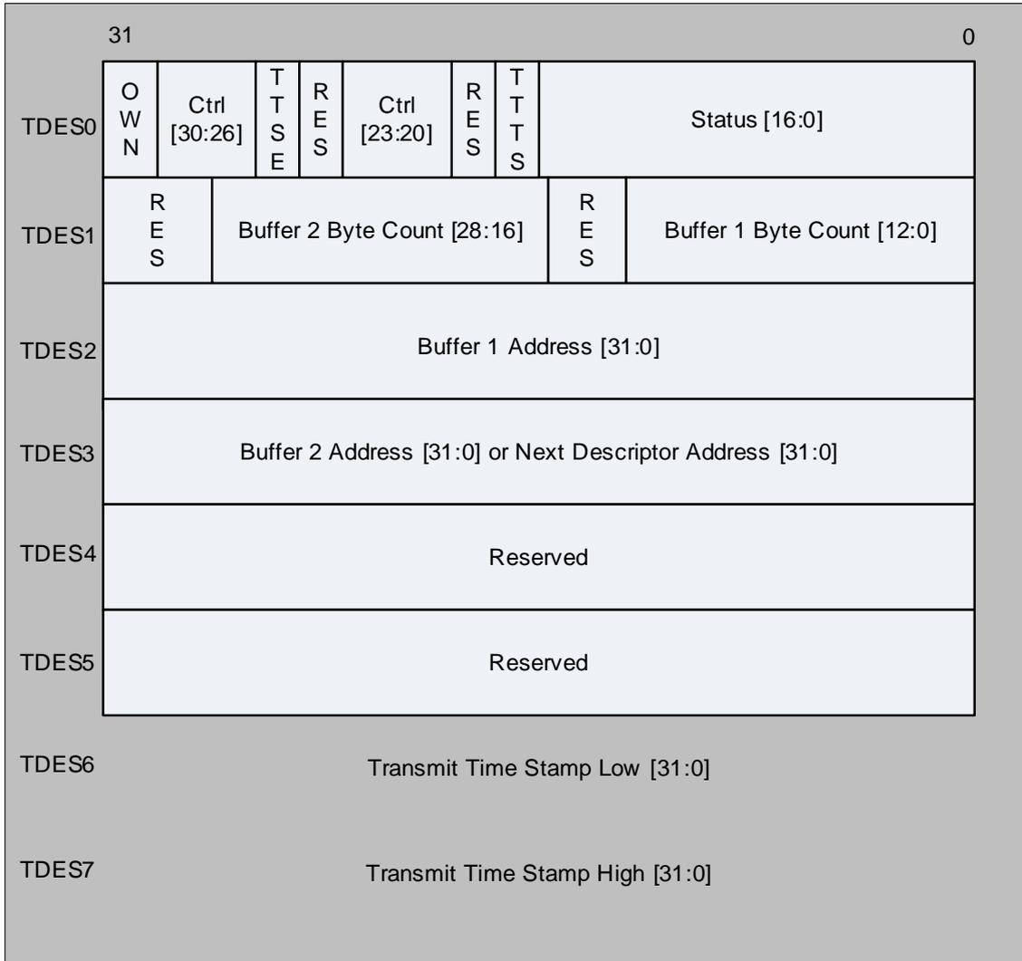
Fig 76. Transmitter descriptor fields
