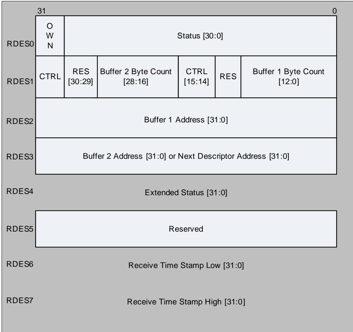
**Fig 78. Receive descriptor fields (alternate configuration)**
