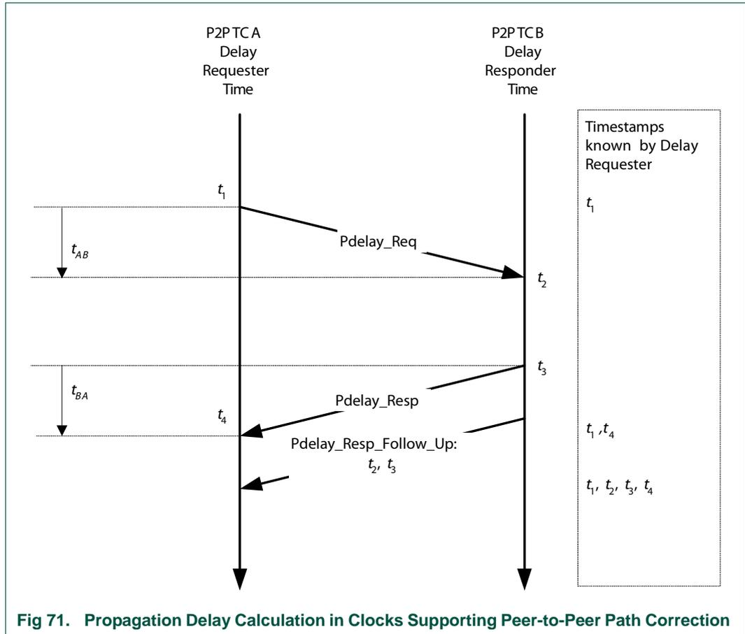
**Fig 71. Propagation Delay Calculation in Clocks Supporting Peer-to-Peer Path Correction**
