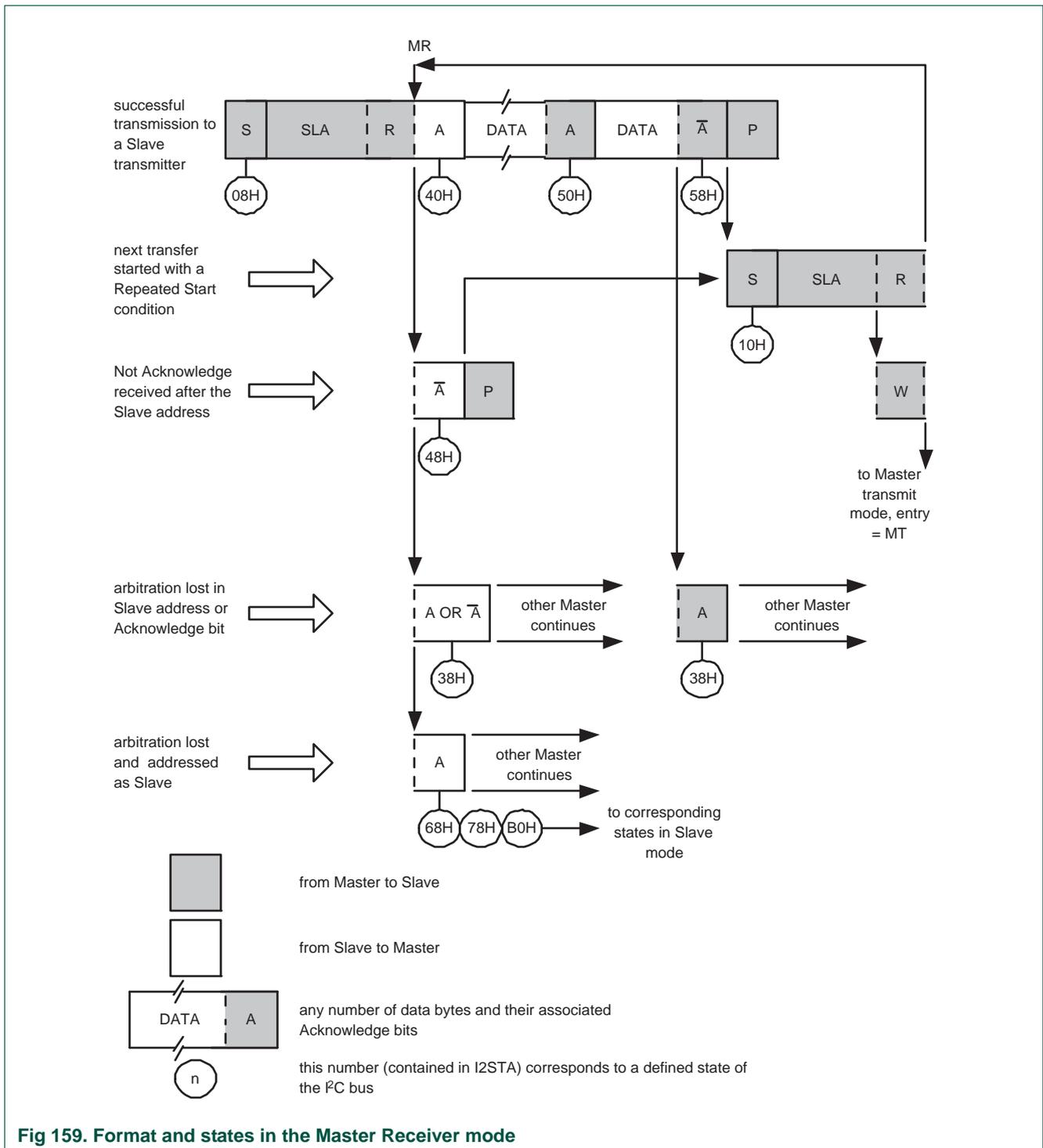
Fig 159. Format and states in the Master Receiver mode
