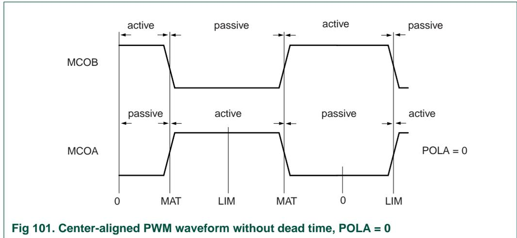
Fig 101. Center-aligned PWM waveform without dead time, POLA = 0
