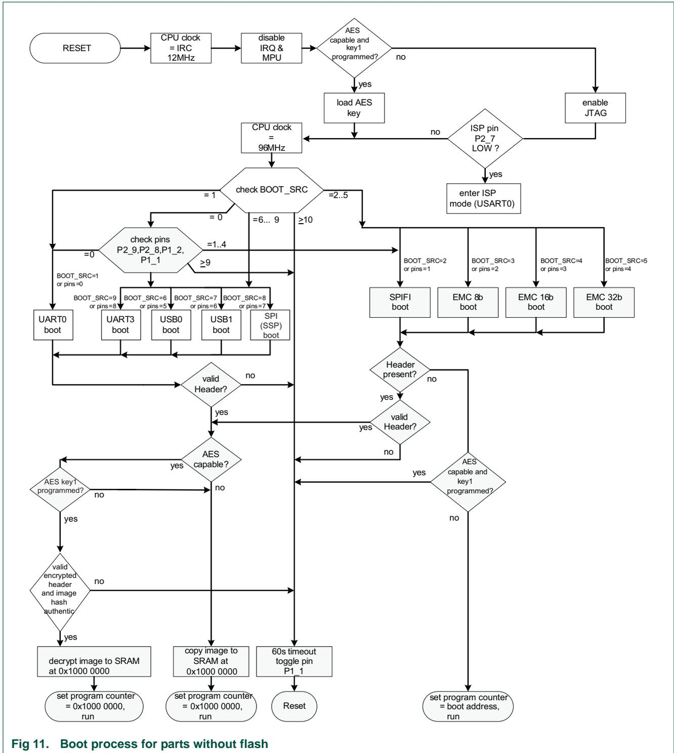
Fig 11. Boot process for parts without flash
