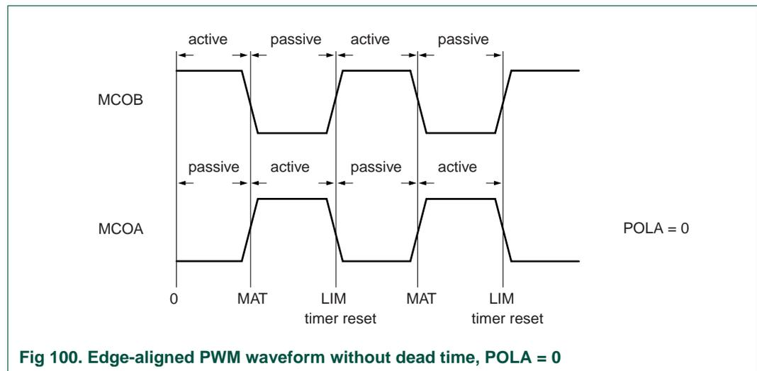
Fig 100. Edge-aligned PWM waveform without dead time, POLA = 0
