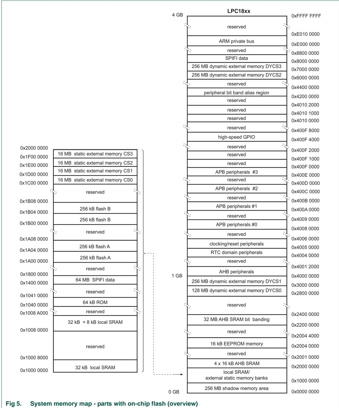
Fig 5. System memory map - parts with on-chip flash (overview)
