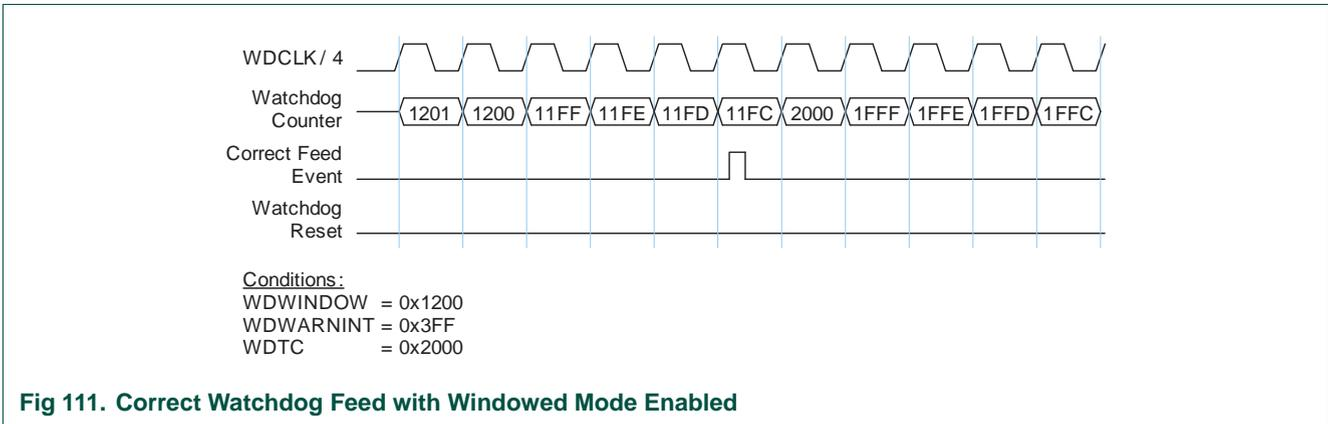
Fig 111. Correct Watchdog Feed with Windowed Mode Enabled
