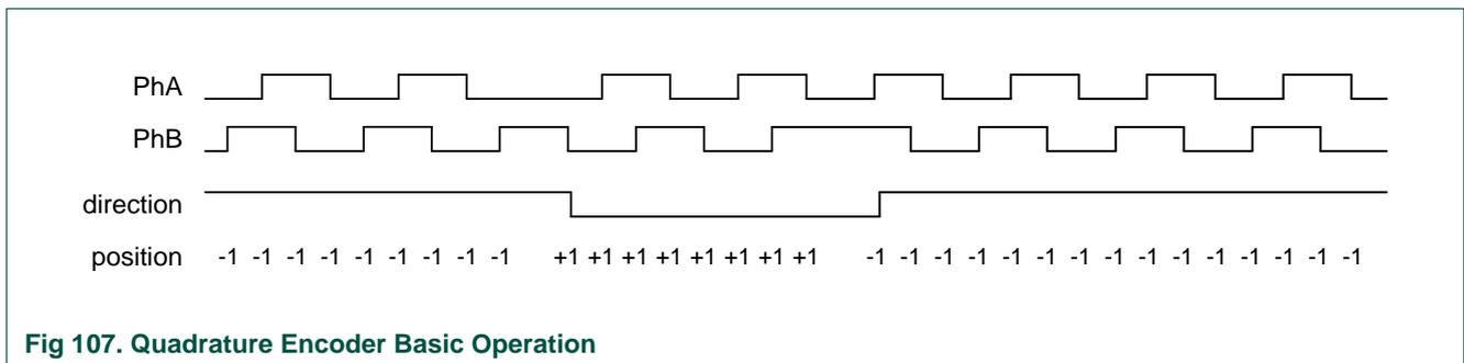
Fig 107. Quadrature Encoder Basic Operation
