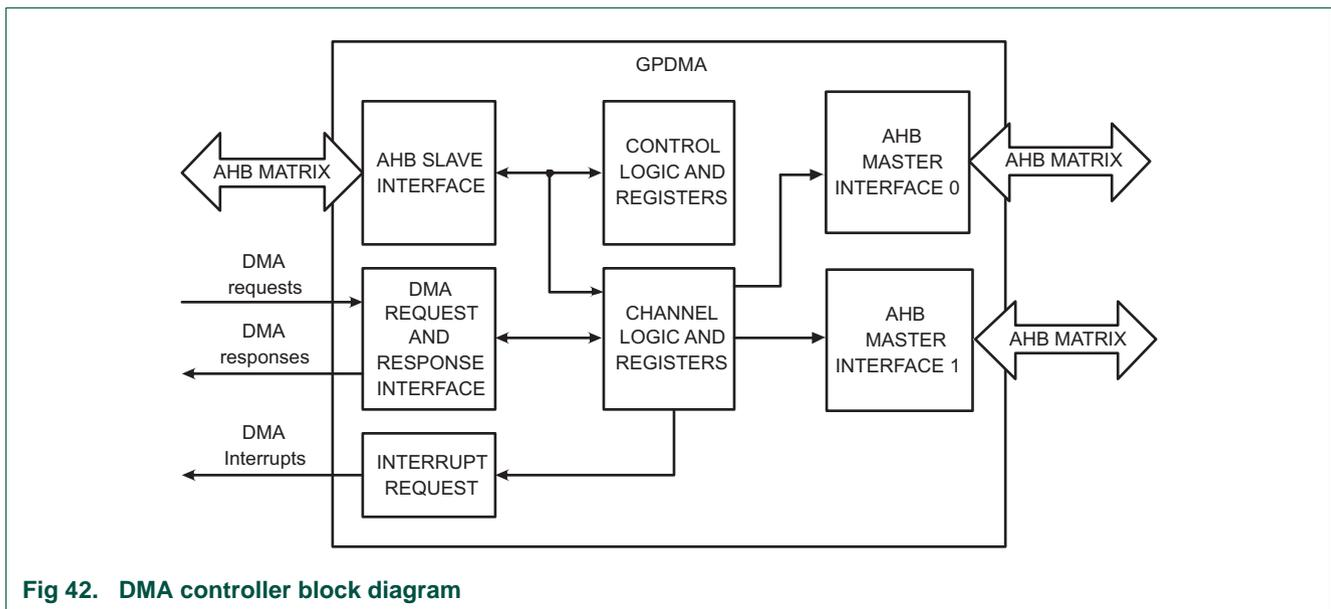
Fig 42. DMA controller block diagram
