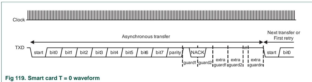
Fig 119. Smart card T = 0 waveform
