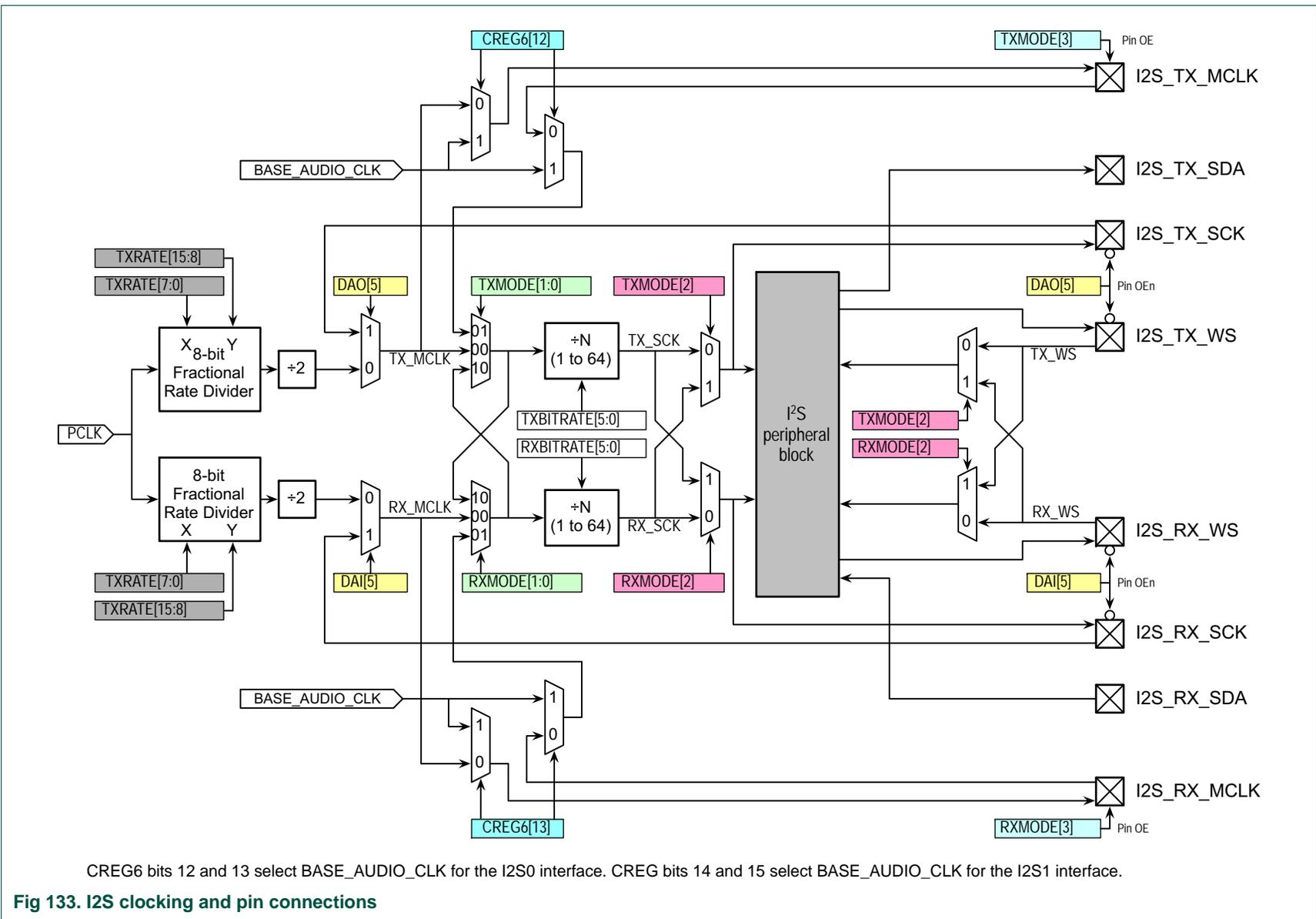
CREG6 bits 12 and 13 select BASE\_AUDIO\_CLK for the I2S0 interface. CREG bits 14 and 15 select BASE\_AUDIO\_CLK for the I2S1 interface.
