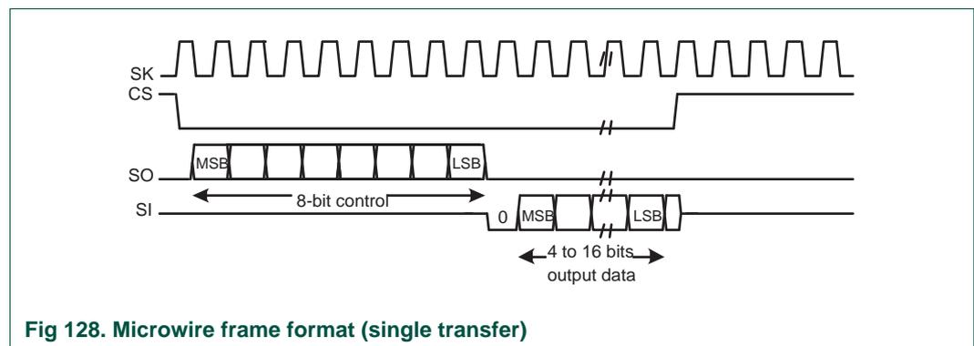
Fig 128. Microwire frame format (single transfer)
