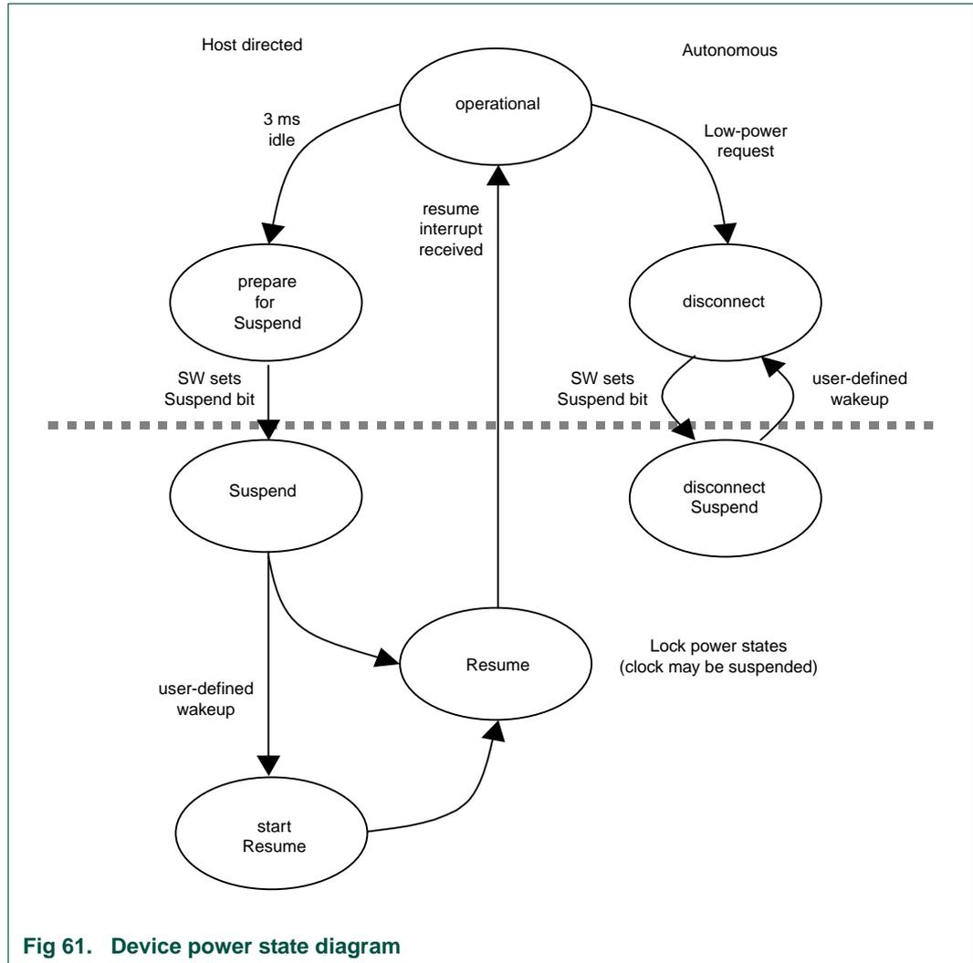
Fig 61. Device power state diagram
