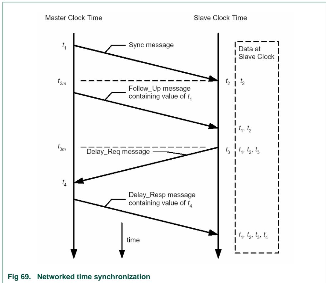
**Fig 69. Networked time synchronization**
