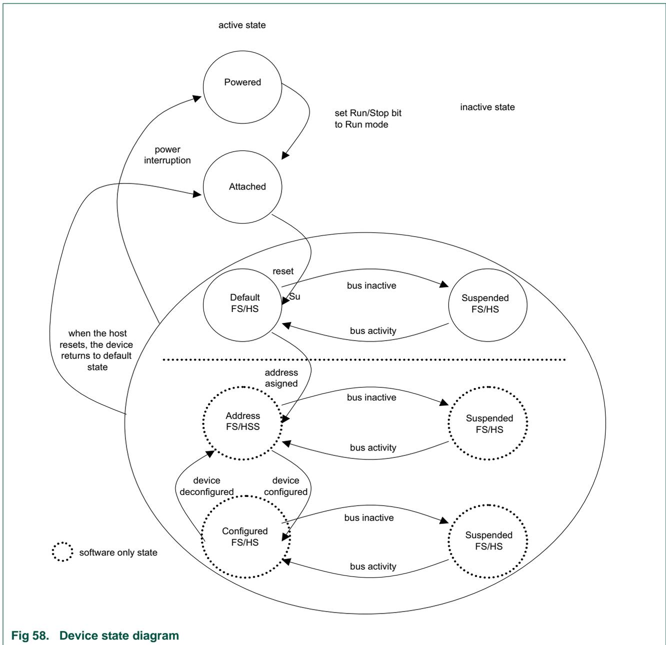
Fig 58. Device state diagram
