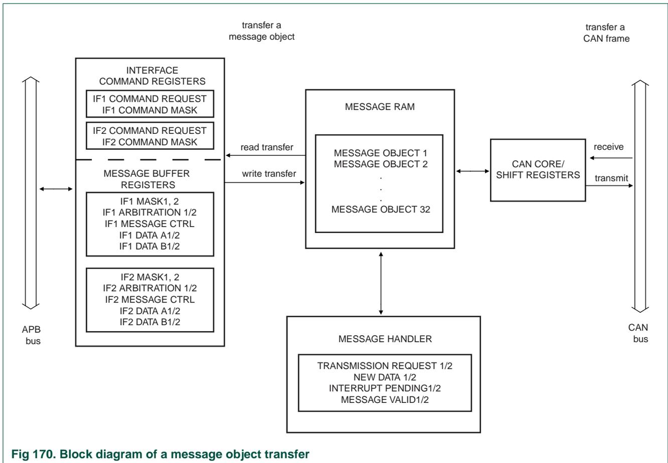
Fig 170. Block diagram of a message object transfer
