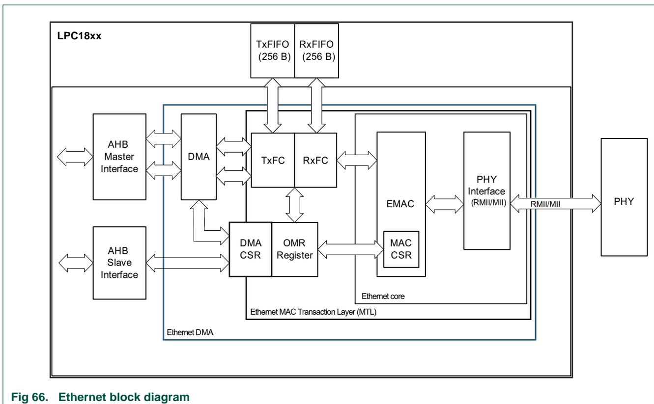
Fig 66. Ethernet block diagram
