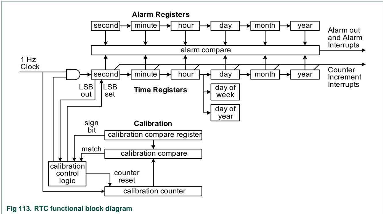
Fig 113. RTC functional block diagram
