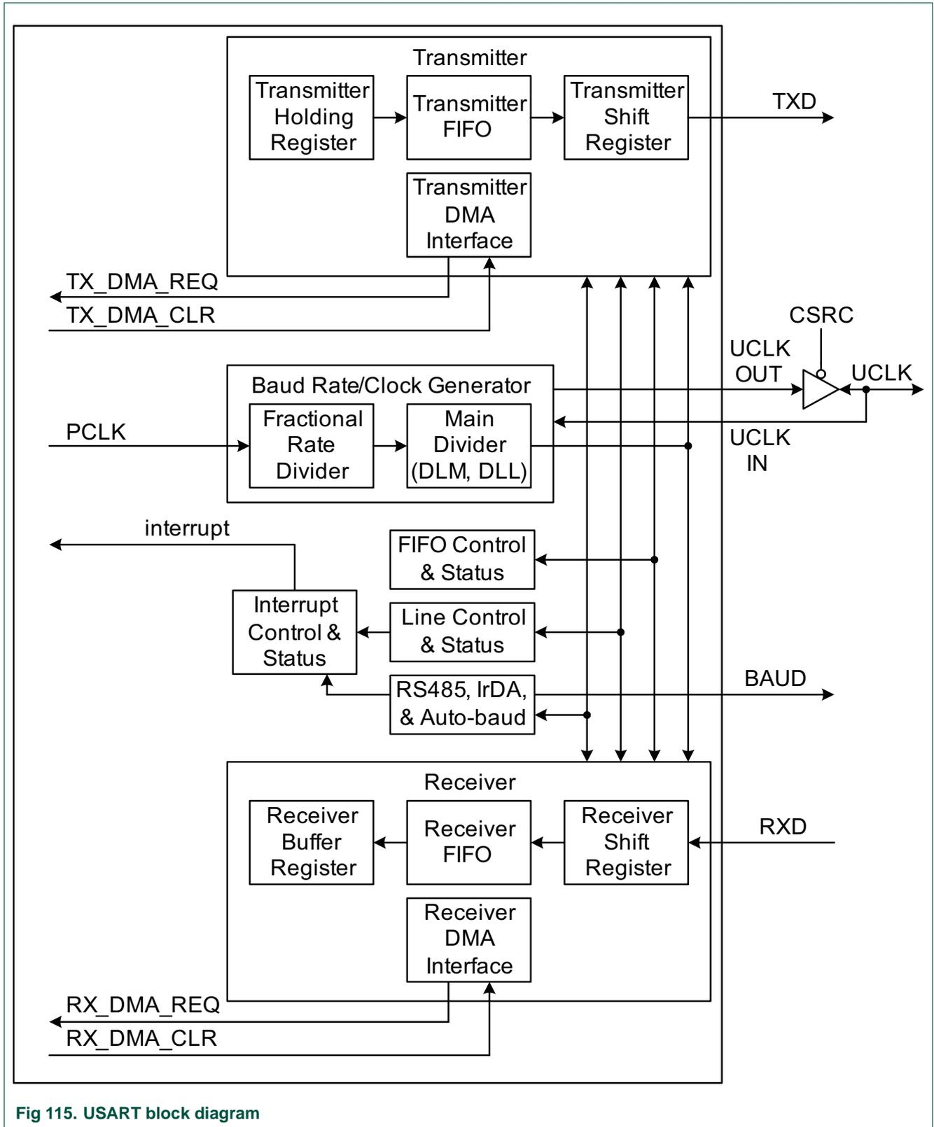
Fig 115. USART block diagram
