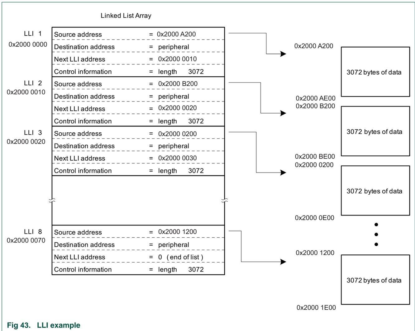
The first LLI, stored at 0x2000 0000, defines the first block of data to be transferred, which is the data stored from address 0x2000 A200 to 0x2000 AE00:
