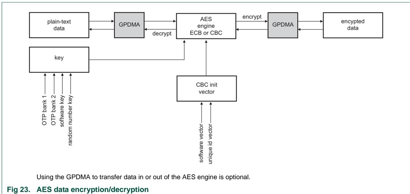
**Fig 23. AES data encryption/decryption**
