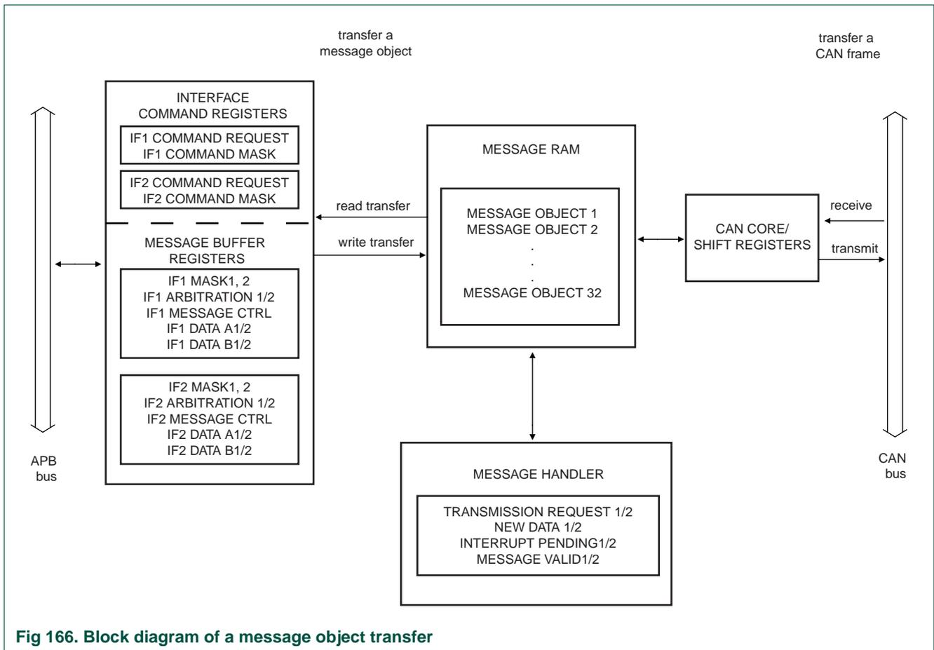
Fig 166. Block diagram of a message object transfer
