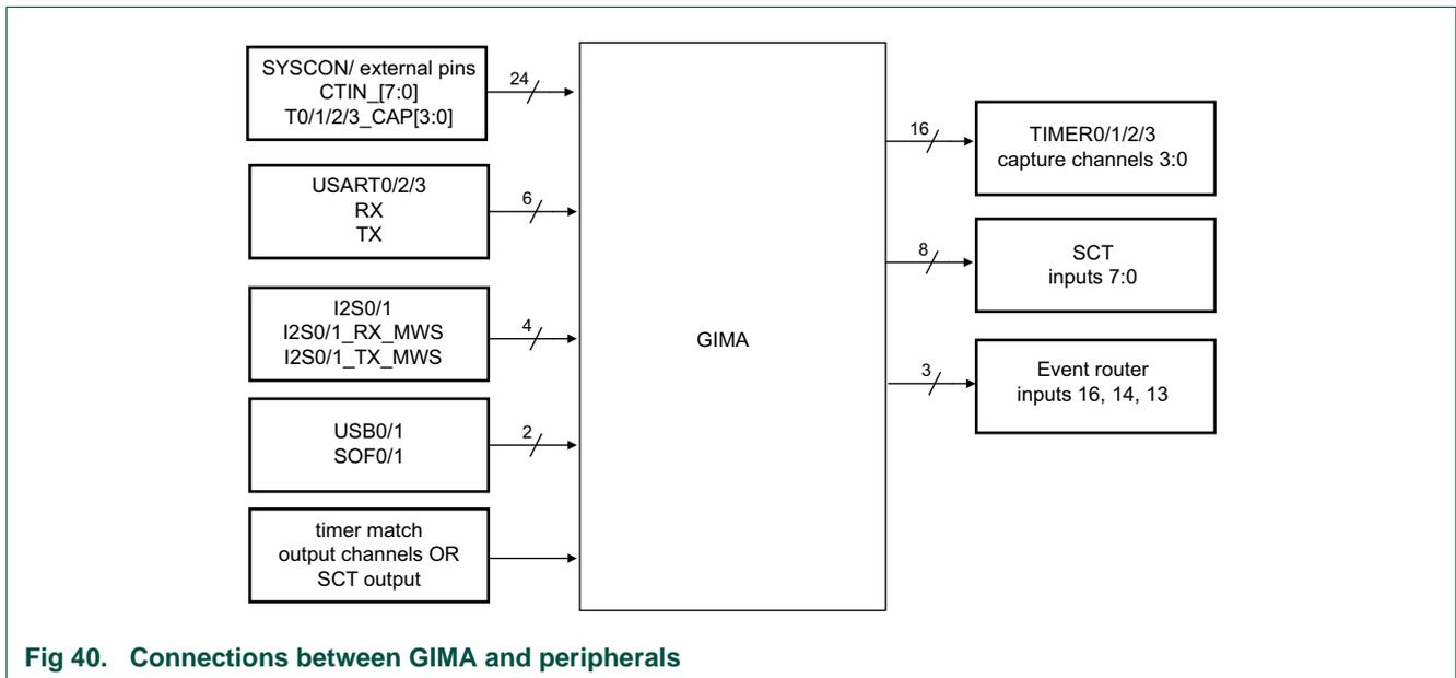
Fig 40. Connections between GIMA and peripherals
