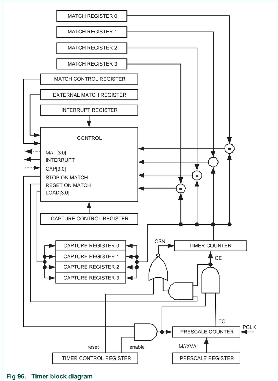
Fig 96. Timer block diagram
