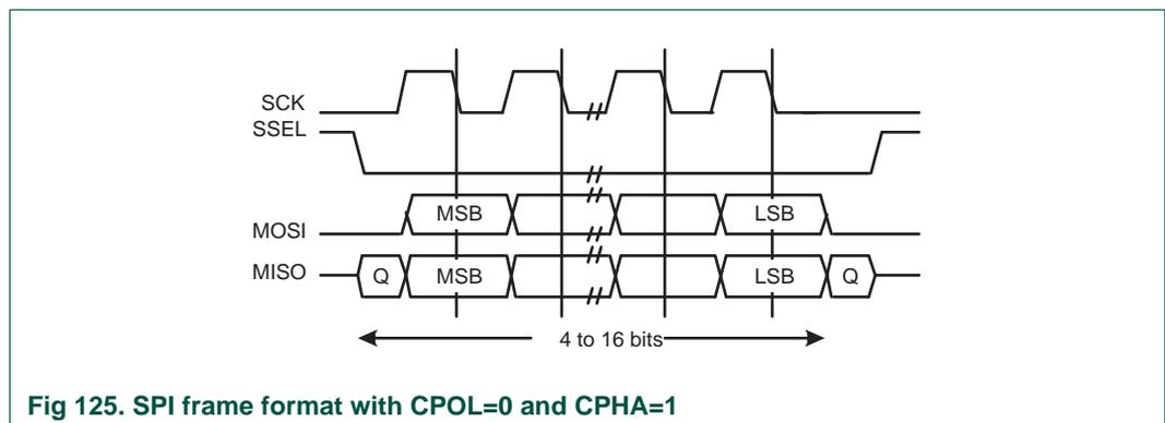
Fig 125. SPI frame format with CPOL=0 and CPHA=1
