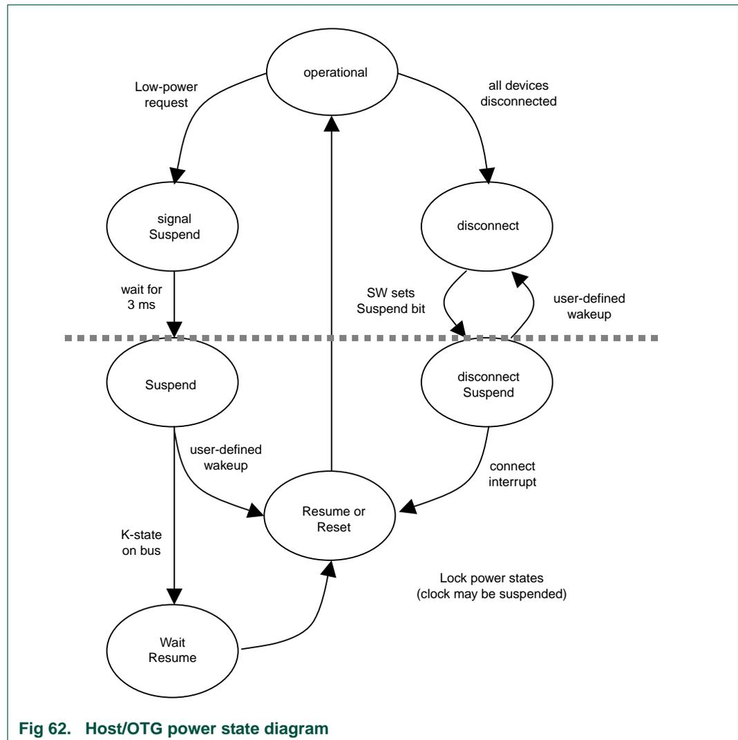
Fig 62. Host/OTG power state diagram
