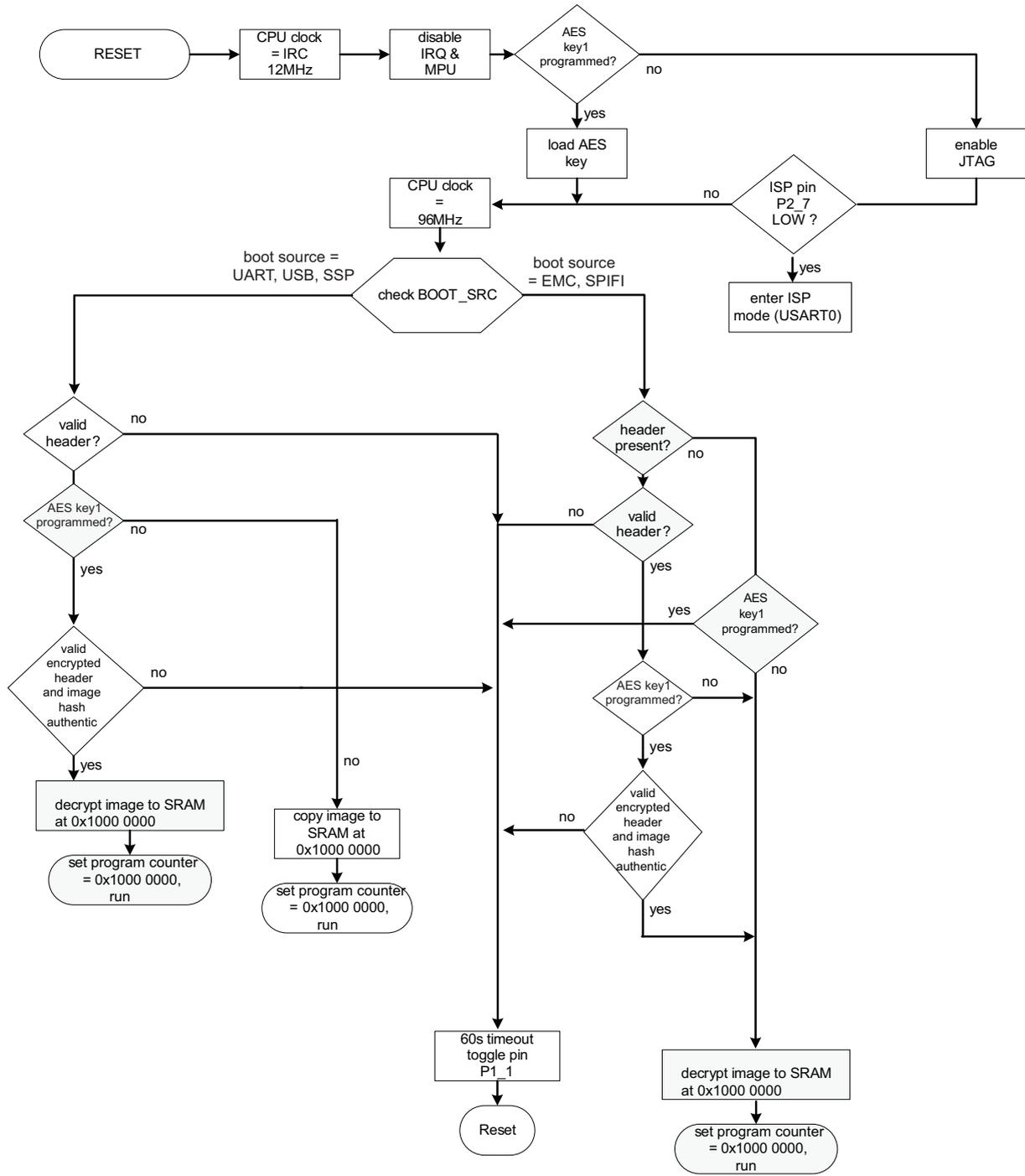
For parts with on-chip flash, the boot source is checked when the ISP pin is pulled LOW. All other flows are identical to flashless parts. See [Figure 11](#).
