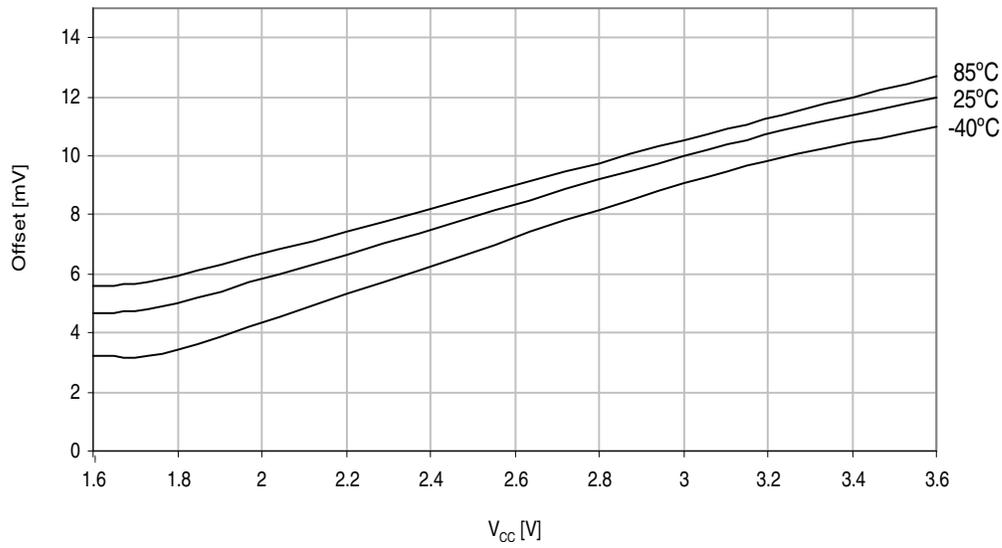
**Figure 37-29. ADC Offset vs.  $V_{REF}$**
