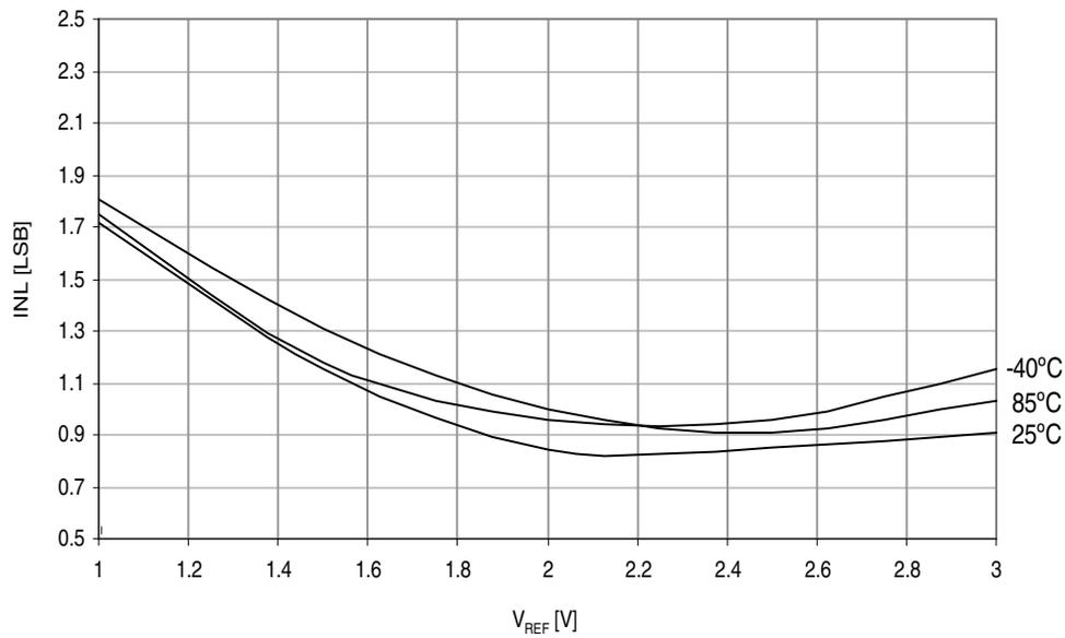
**Figure 37-25. ADC INL vs.  $V_{REF}$ .**
