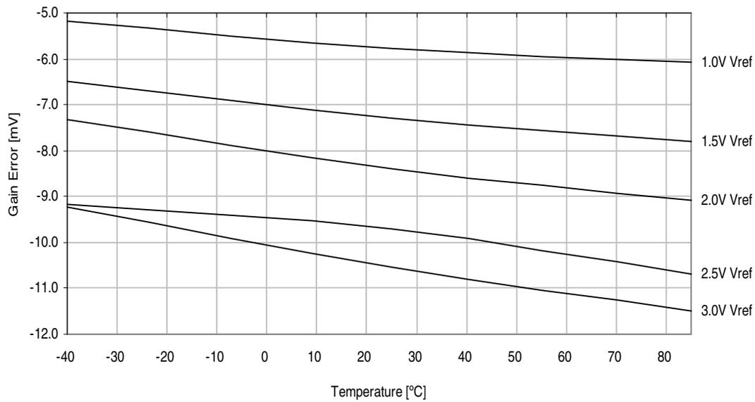
**Figure 37-37. ADC Gain Error vs. Temperature.**
