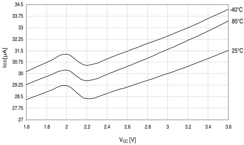
Figure 37-8. Idle mode supply current vs.  $V_{CC}$ .
