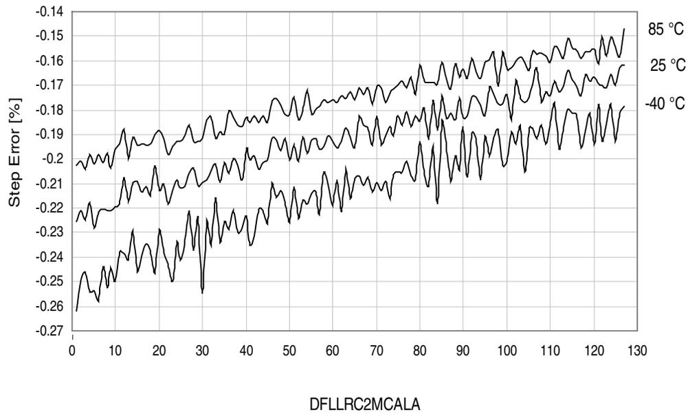
Figure 37-64. 2MHz internal oscillator CALB calibration step size.
