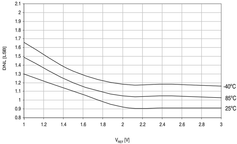
**Figure 37-27. ADC DNL vs.  $V_{REF}$ .**
