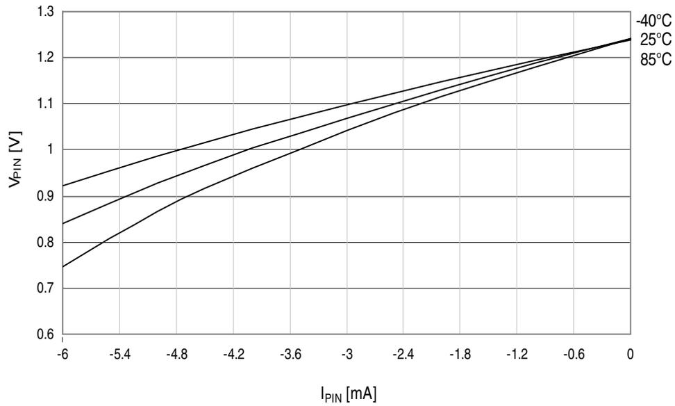
Figure 37-16. I/O pin output voltage vs. source current.
