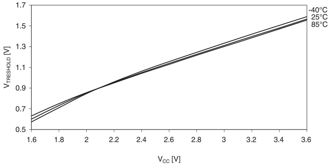
Figure 37-23. I/O pin input hysteresis vs.  $V_{CC}$ .
