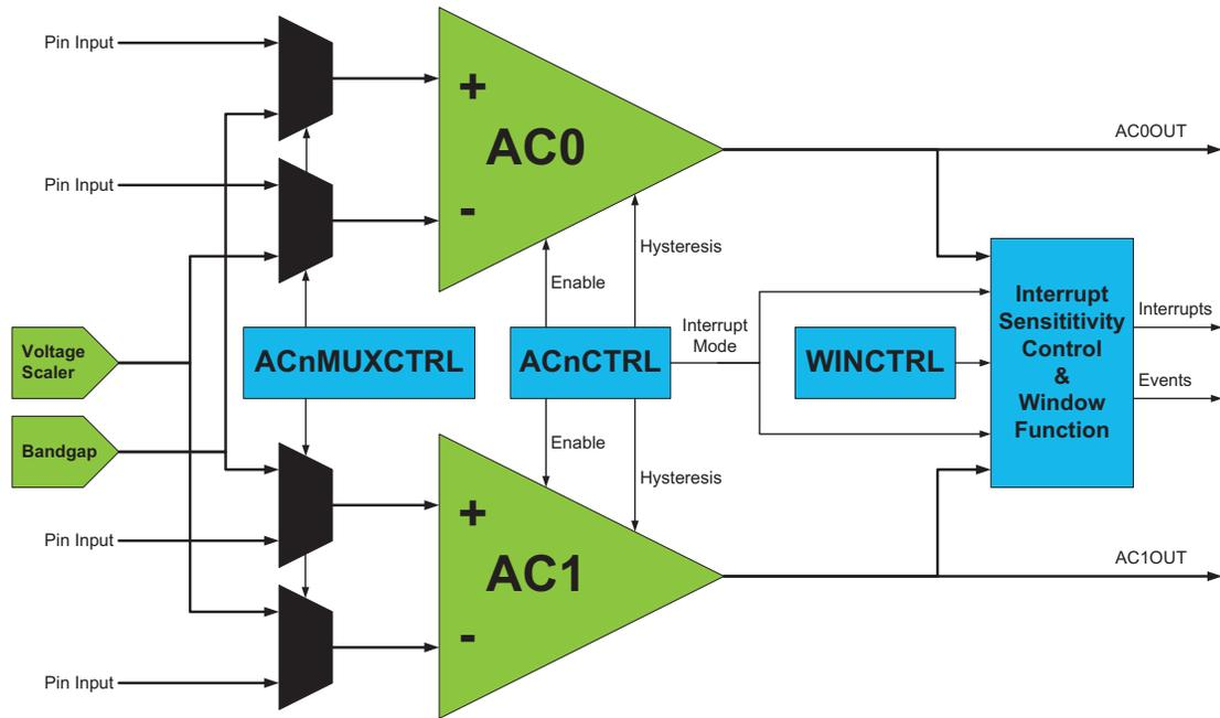
The window function is realized by connecting the external inputs of the two analog comparators in a pair as shown in [Figure 30-2](#).
