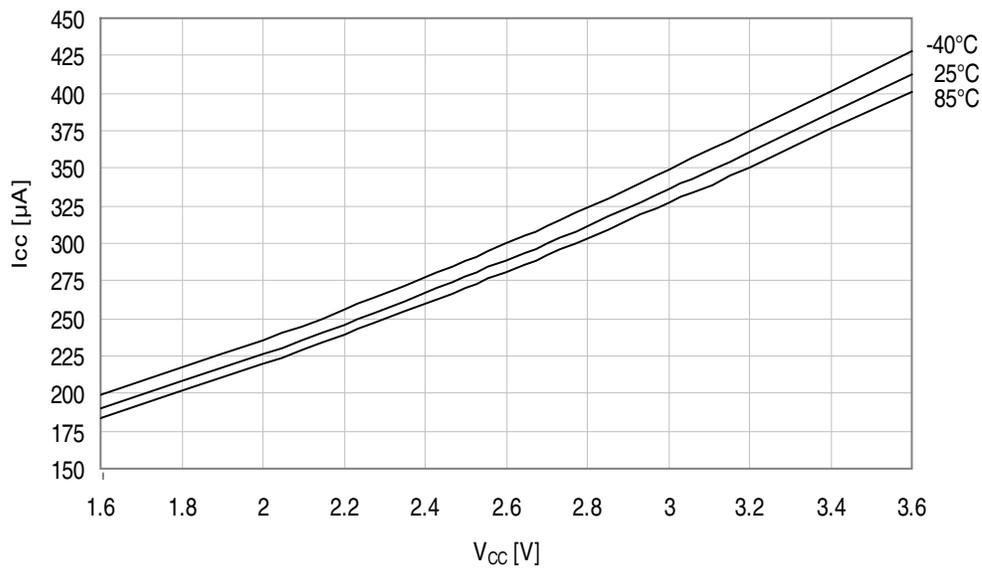
**Figure 37-9. Idle mode current vs.  $V_{CC}$ .**
