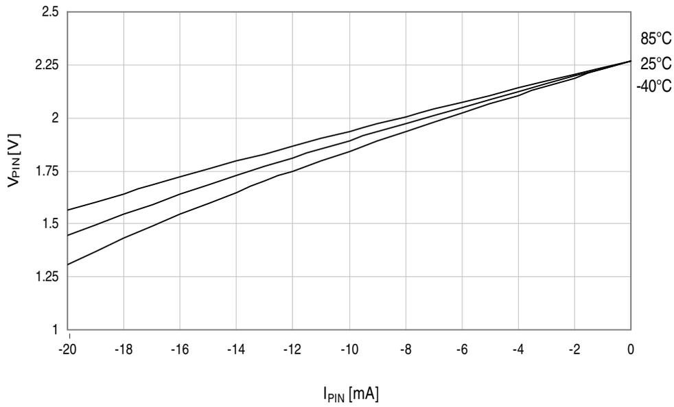
Figure 37-18. I/O pin output voltage vs. sink current.
