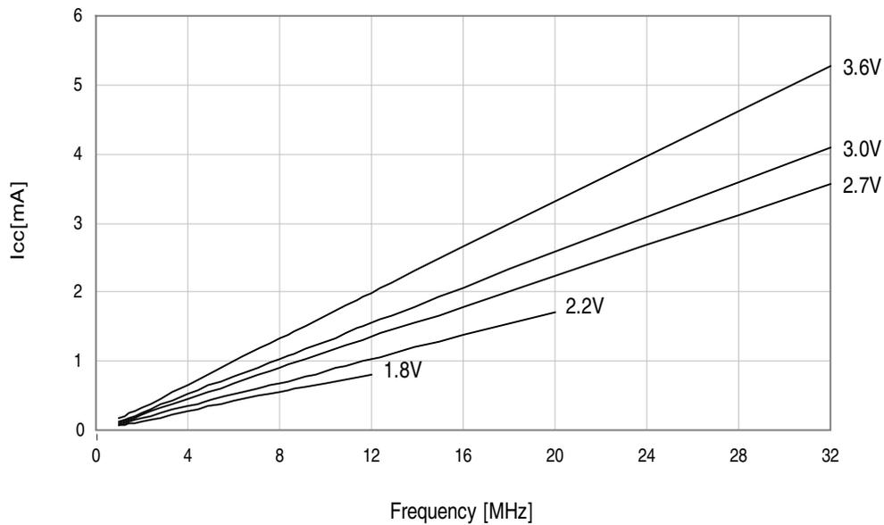
Figure 37-7. Idle mode supply current vs.  $V_{CC}$ .
