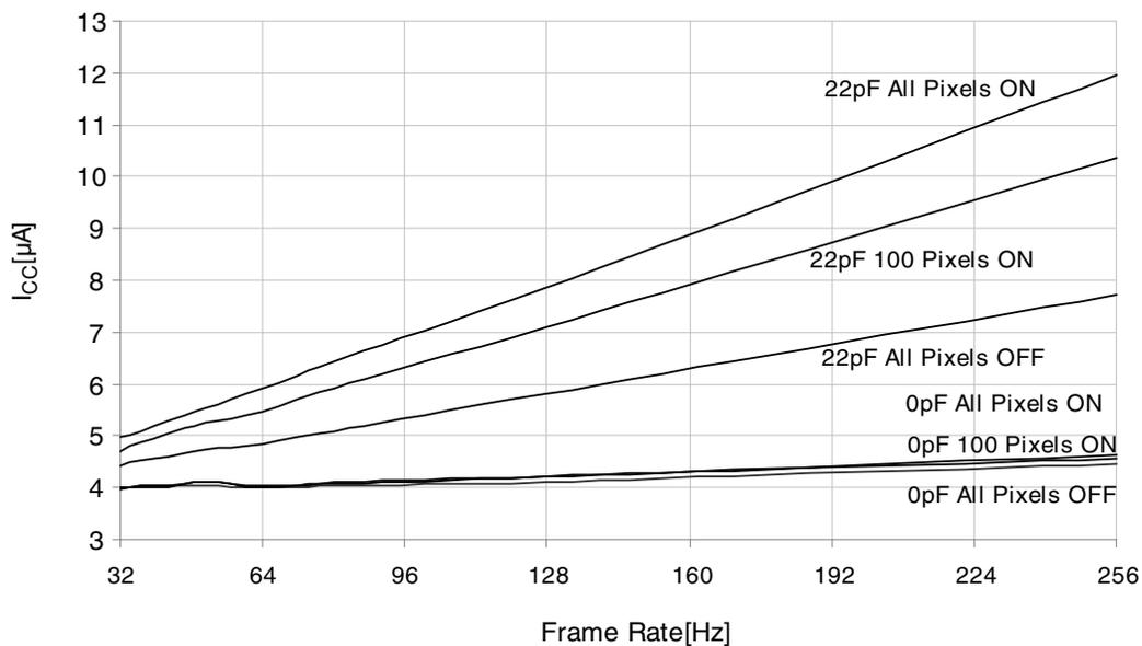
**Figure 37-78.  $I_{CC}$  vs. Frame Rate**
