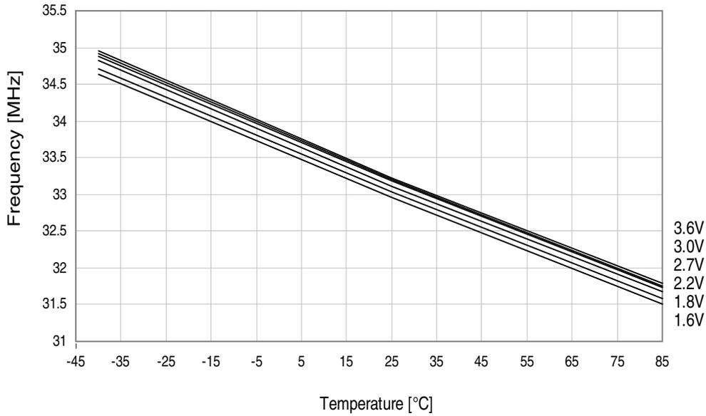
Figure 37-66. 32MHz internal oscillator frequency vs. temperature.
