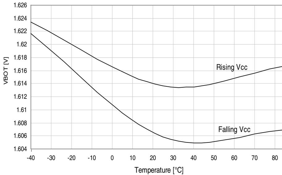
Figure 37-49. BOD thresholds vs. temperature.
