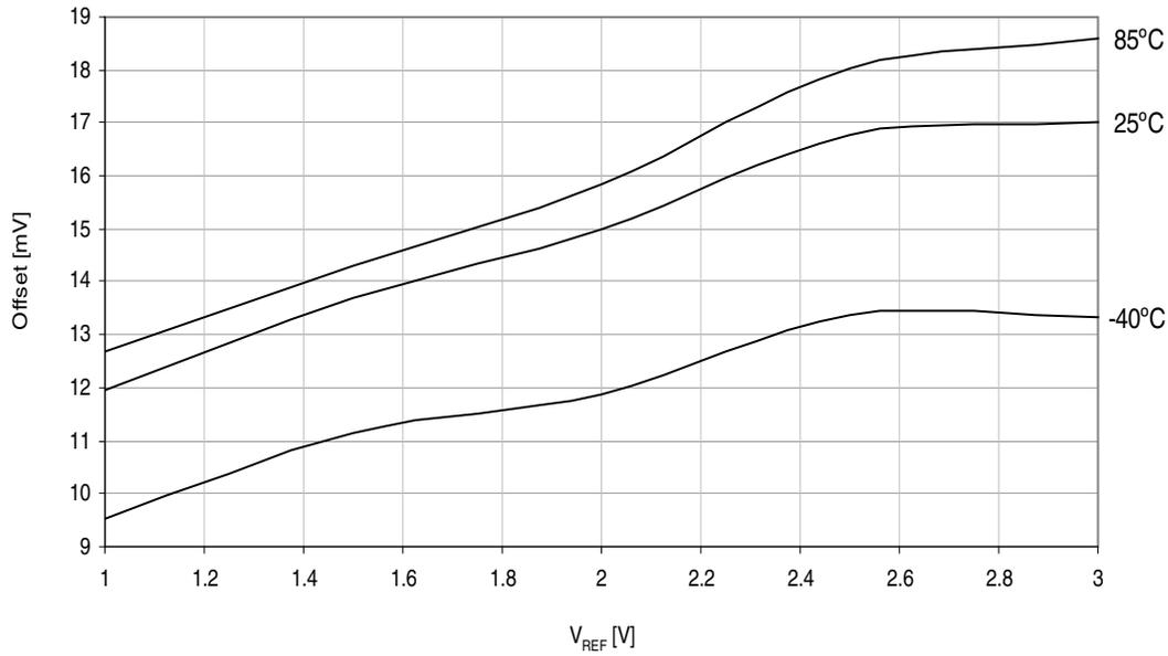
**Figure 37-30. ADC Offset vs.  $V_{REF}$**
