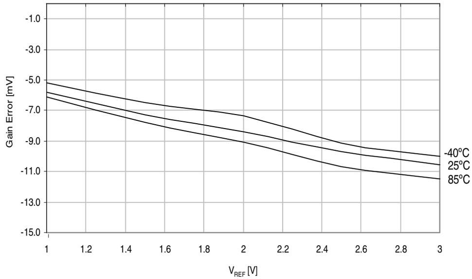
**Figure 37-33. ADC Gain Error vs.  $V_{REF}$ .**
