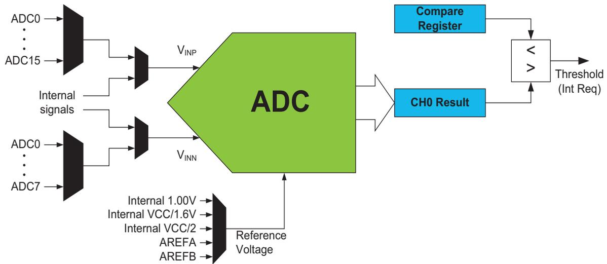
The ADC may be configured for 8- or 12-bit result, reducing the minimum conversion time (propagation delay) from 3.35 $\mu$ s for 12-bit to 2.3 $\mu$ s for 8-bit result.
