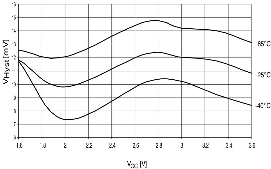
**Figure 37-39. Analog comparator hysteresis vs.  $V_{CC}$ .**
