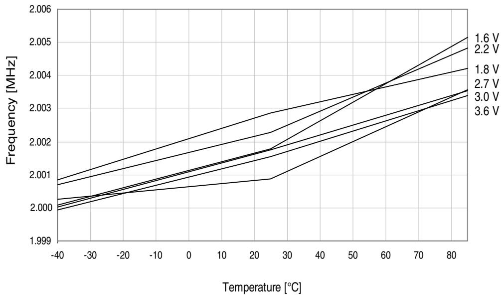
Figure 37-63. 2MHz internal oscillator CALA calibration step size.
