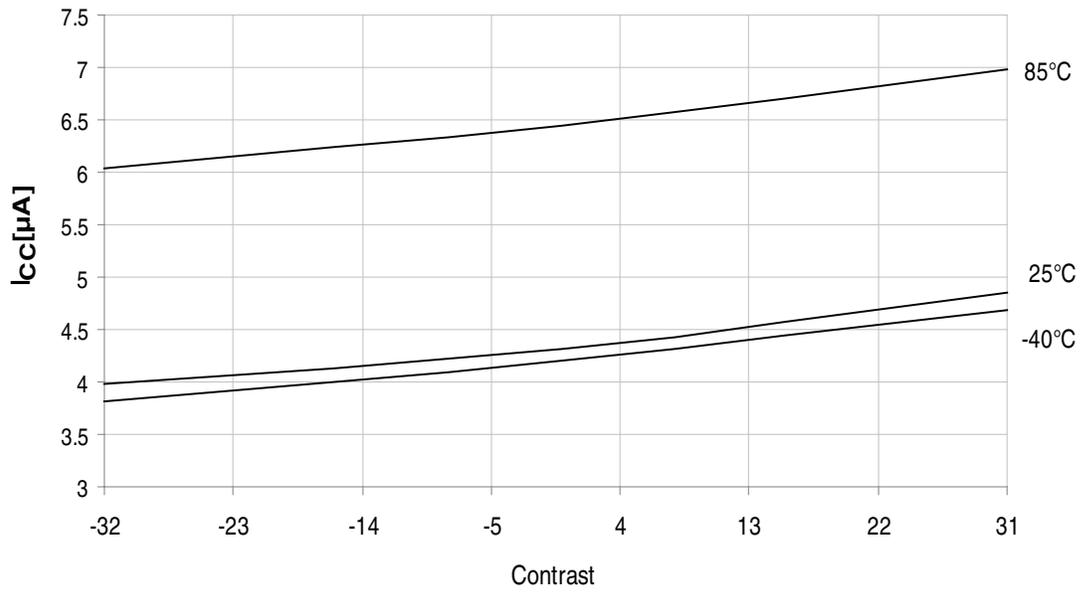
**Figure 37-81. Psave LCD LP 32Hz vs. Temperature**
