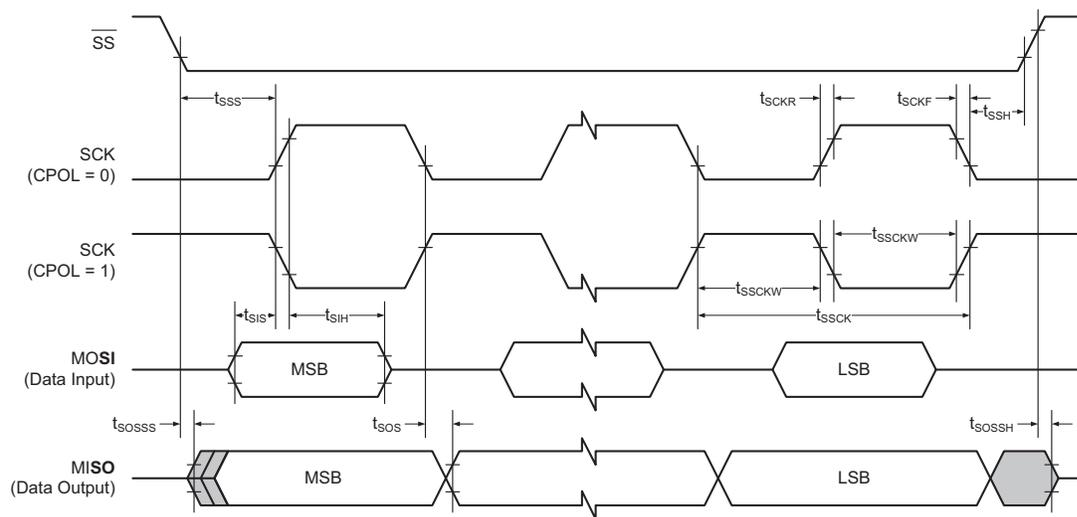
**Table 36-29. SPI Timing characteristics and requirements.**
