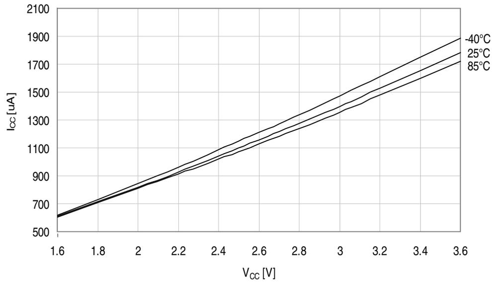
Figure 37-4. Active mode supply current vs.  $V_{CC}$ .
