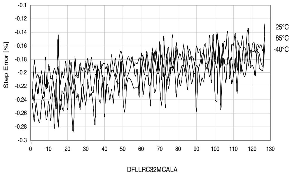
Figure 37-68. 32MHz internal oscillator CALB calibration step size.
