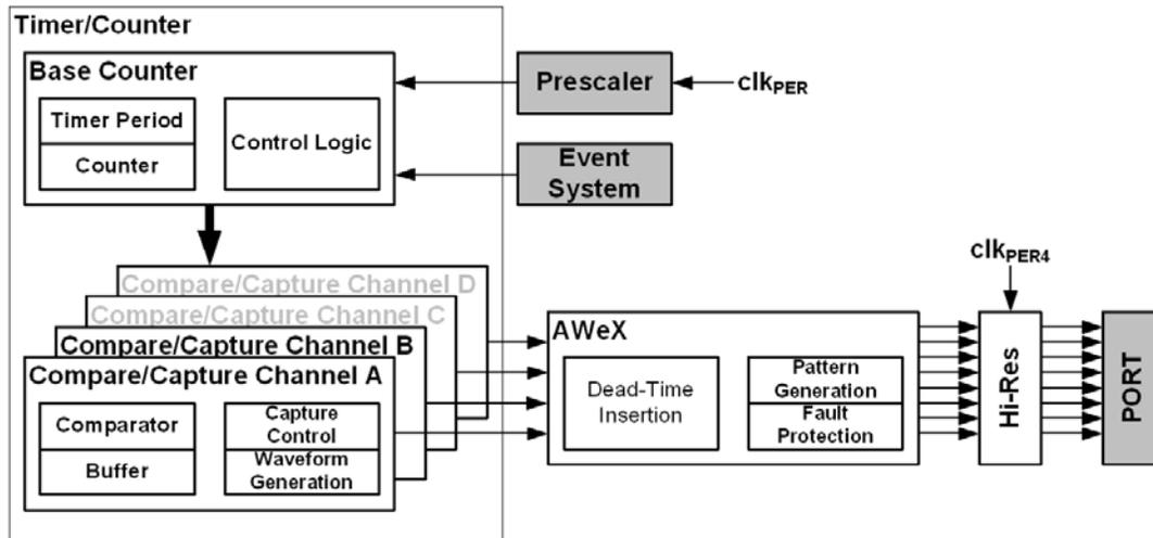
PORTC has one Timer/Counter 0 and one Timer/Counter1. Notation of these are TCC0 (Time/Counter C0) and TCC1 respectively.
