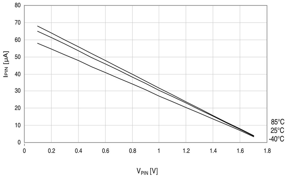
Figure 37-13. I/O pin pull-up resistor current vs. input voltage.
