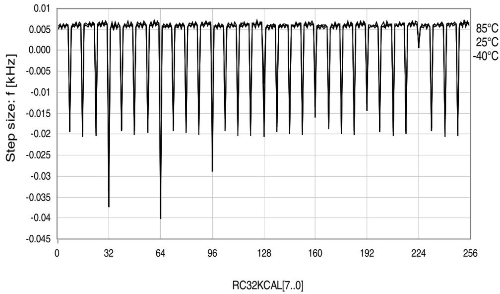
Figure 37-60. 32.768kHz internal oscillator frequency vs. calibration value.
