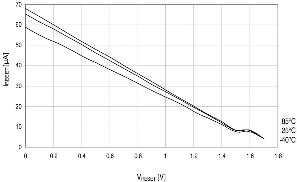
Figure 37-53. Reset pin pull-up resistor current vs. reset pin voltage.
