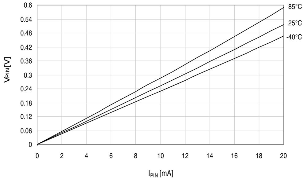
Figure 37-20. I/O pin output voltage vs. sink current.
