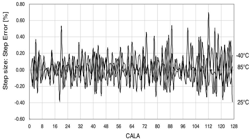
**Figure 37-74. 48MHz internal oscillator frequency vs. CALA calibration value.**
