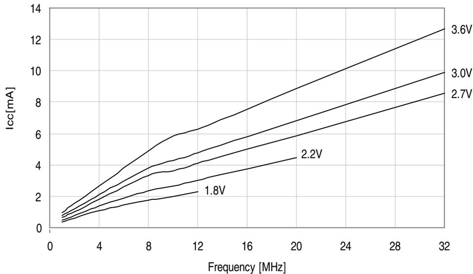
Figure 37-3. Active mode supply current vs.  $V_{CC}$ .
