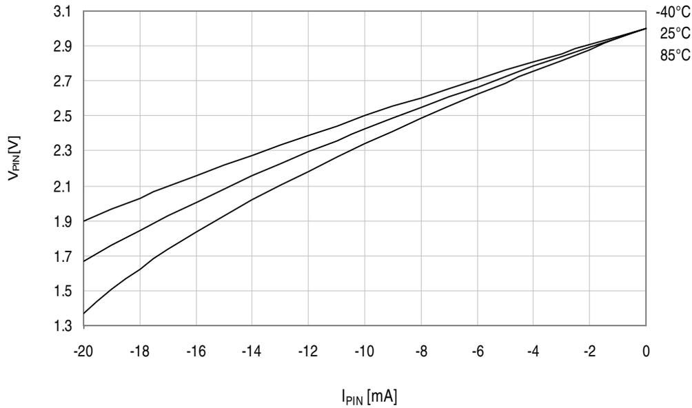
Figure 37-17. I/O pin output voltage vs. source current.
