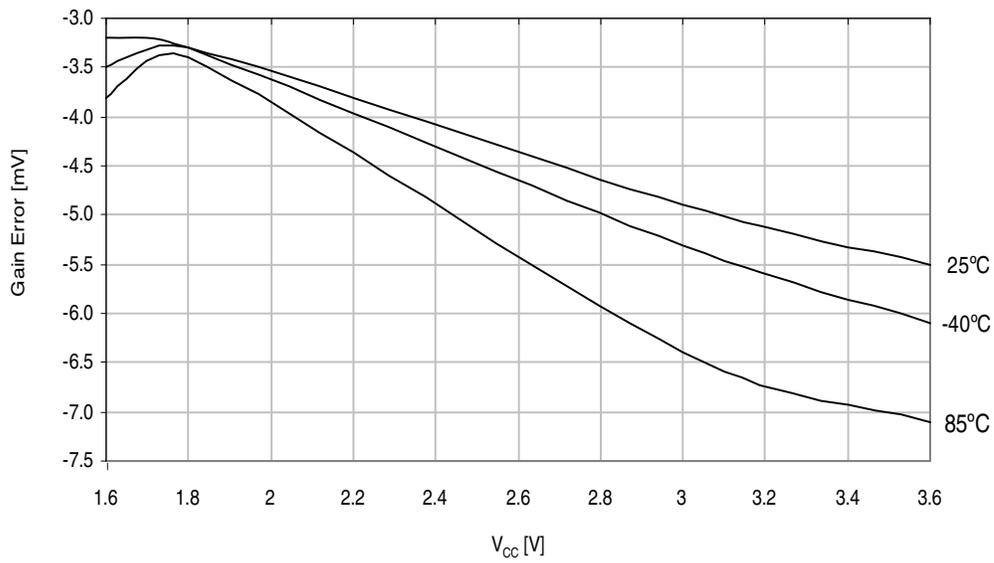
**Figure 37-35. ADC Gain Error vs.  $V_{CC}$ .**
