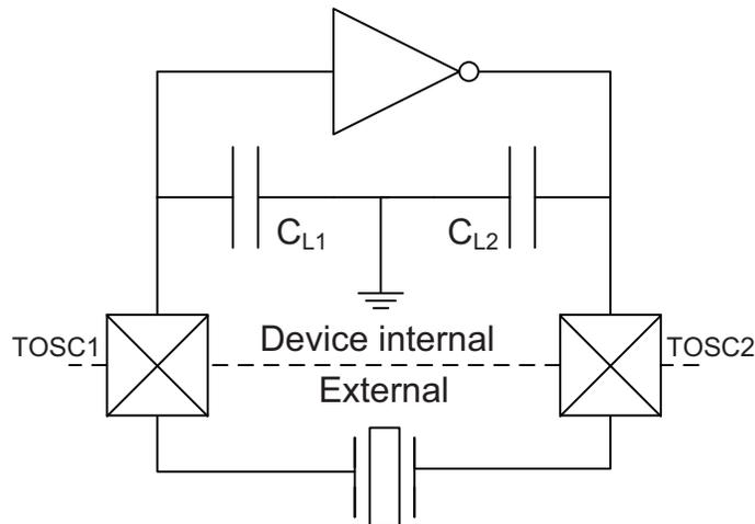
The input capacitance between the TOSC pins is  $C_{L1} + C_{L2}$  in series as seen from the crystal when oscillating without external capacitors.
