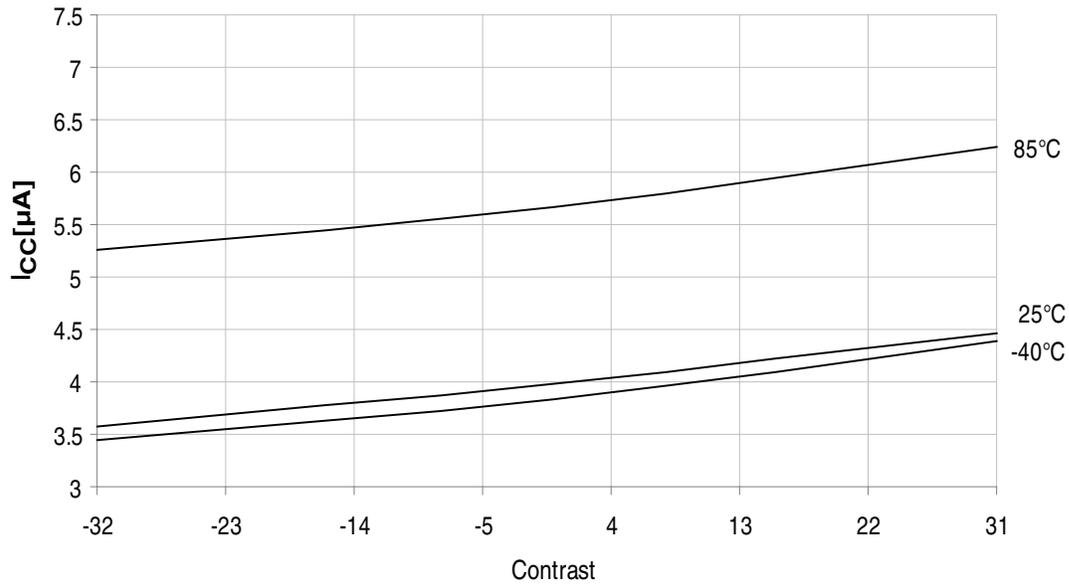
**Figure 37-80.  $I_{CC}$  vs. Contrast**
