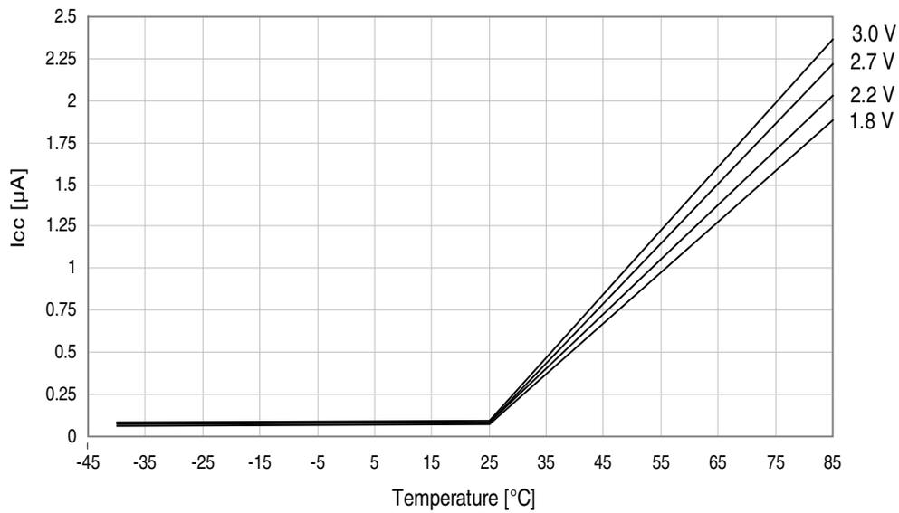
**Figure 37-11. Power-down mode supply current vs. Temperature.**
