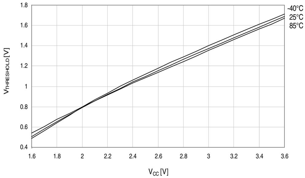
Figure 37-56. Reset pin input threshold voltage vs.  $V_{CC}$ .
