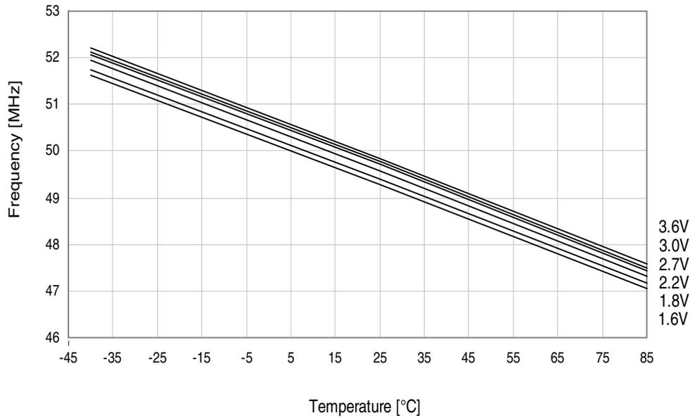
Figure 37-72. 48MHz internal oscillator frequency vs. temperature.
