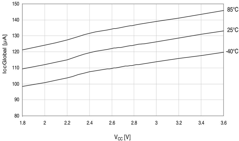
**Figure 37-47. BOD current consumption vs.  $V_{CC}$ .**
