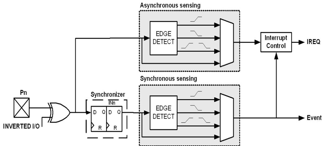
When a pin is configured with inverted I/O, the pin value is inverted before the input sensing.
