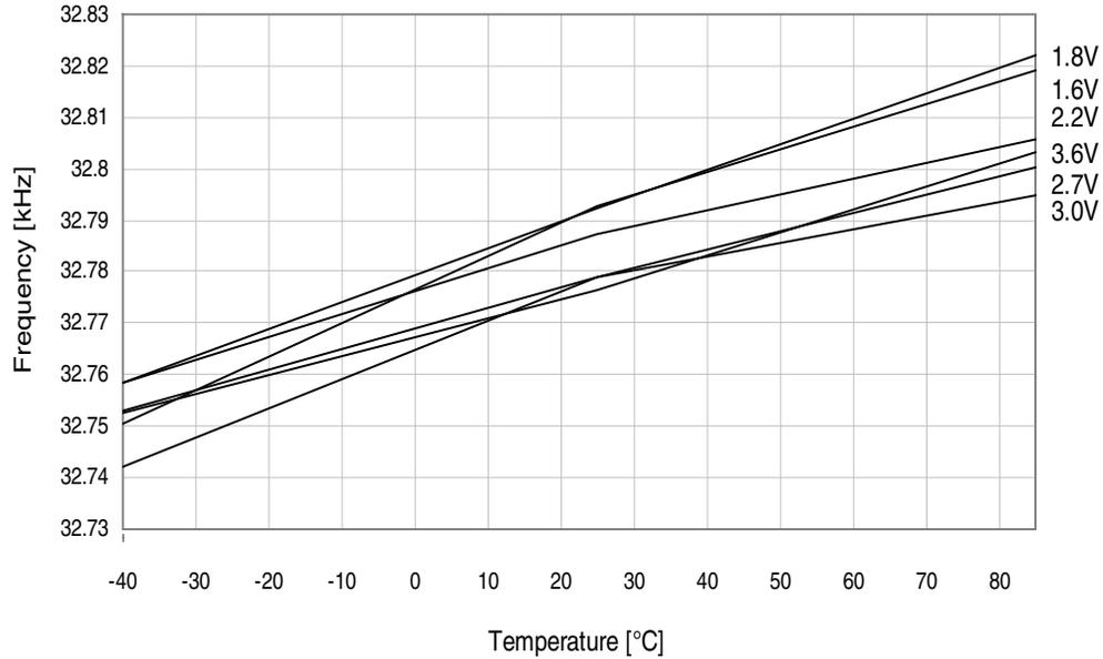
Figure 37-58. 32.768kHz ULP internal oscillator frequency vs. temperature.
