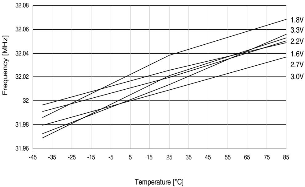
Figure 37-67. 32MHz internal oscillator CALA calibration step size.
