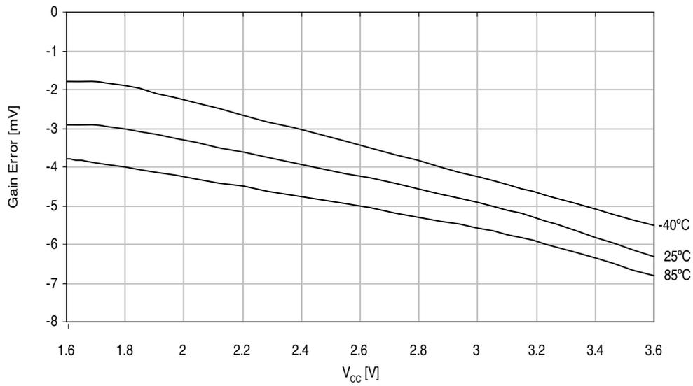
**Figure 37-36. ADC Gain Error vs. Temperature.**
