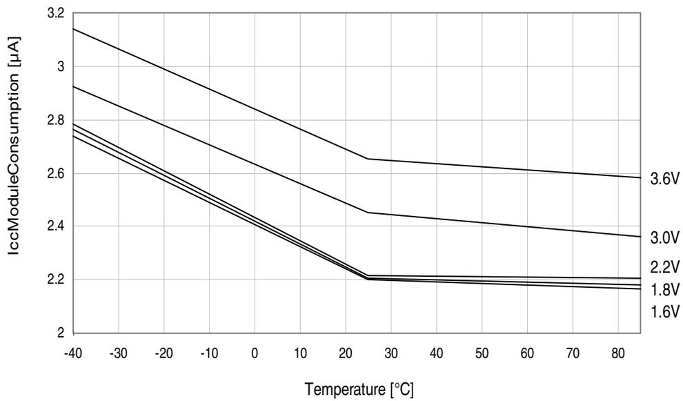
**Figure 37-82. Psave LCD LP 32Hz vs. Temperature**
