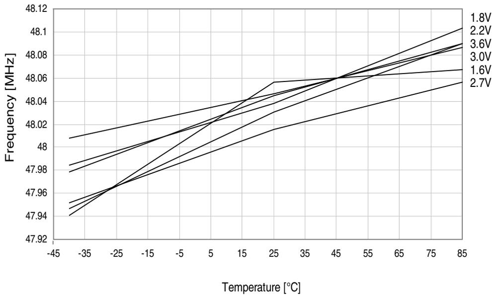
**Figure 37-73. 32MHz internal oscillator CALA calibration step size.**
