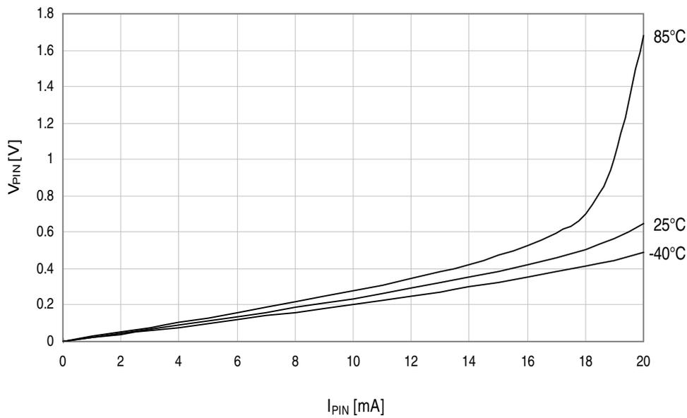
Figure 37-19. I/O pin output voltage vs. sink current.
