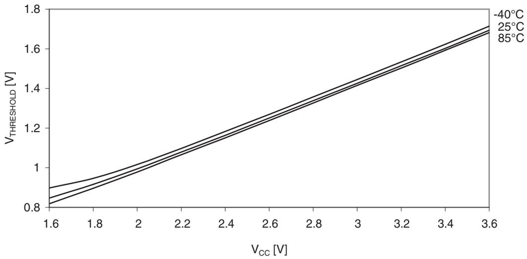
Figure 37-22. I/O pin input threshold voltage vs.  $V_{CC}$ .
