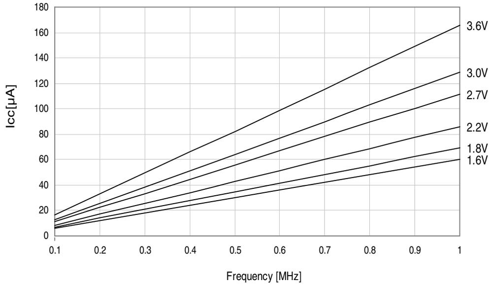
Figure 37-6. Idle mode supply current vs. frequency.
