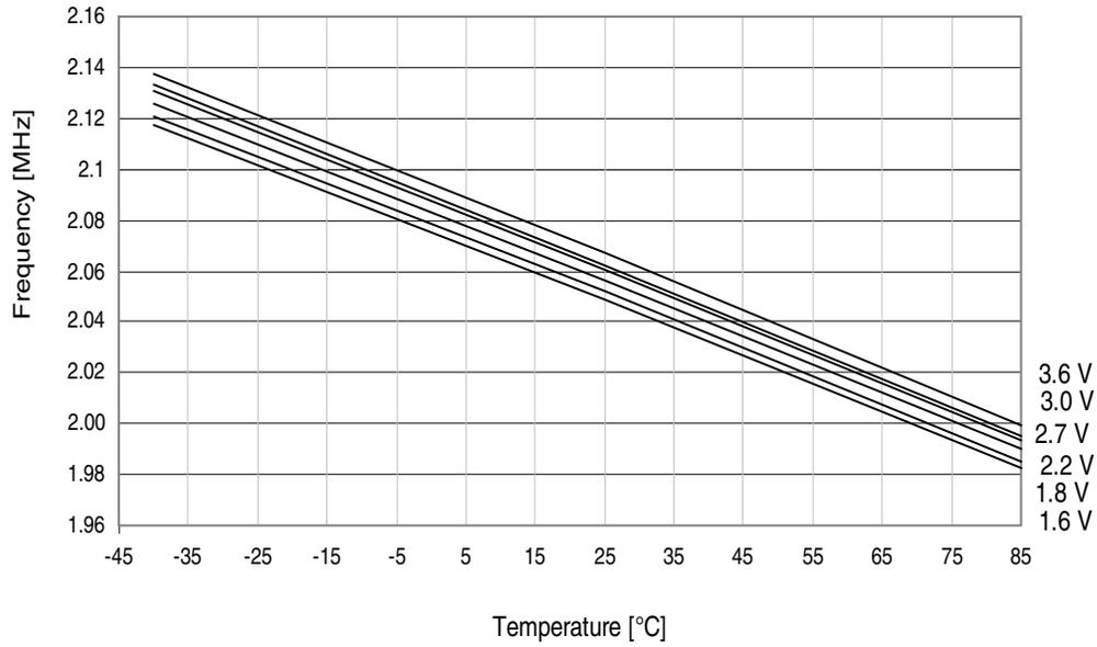
Figure 37-62. 2MHz internal oscillator frequency vs. temperature.
