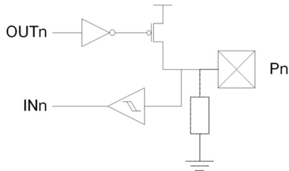
Figure 15-6. I/O configuration - Wired-AND with optional pull-up
