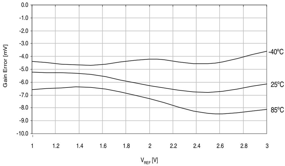
**Figure 37-34. ADC Gain Error vs.  $V_{CC}$ .**
