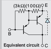
**Silicon PNP Epitaxial Planar Transistor (Complement to type 2SD2081)**
