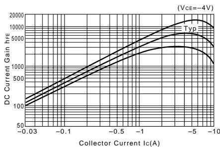
**h<sub>FE</sub>-I<sub>C</sub> Temperature Characteristics (Typical)**
