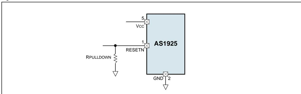
**Note:** A 200kΩ pullup resistor to Vcc is also recommended if the push/pull RESET is required to remain valid for Vcc 0.75V.
