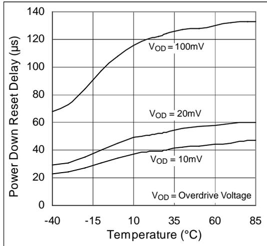
Figure 5. Normalized Reset Timeout Period vs. Temp.
