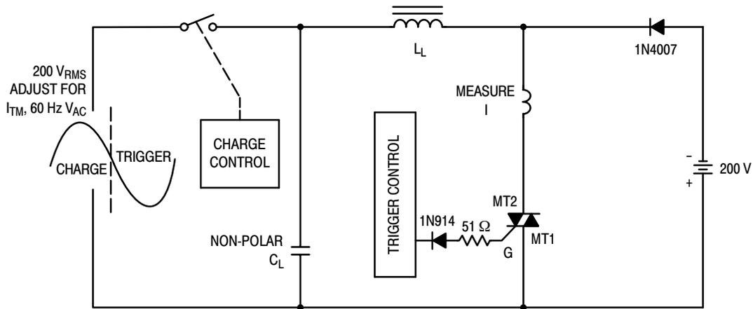
Note: Component values are for verification of rated  $(di/dt)_c$ . See AN1048 for additional information.
