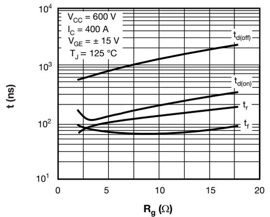
Fig. 8 - Typical Switching Time vs. Gate Resistance  $R_g$
