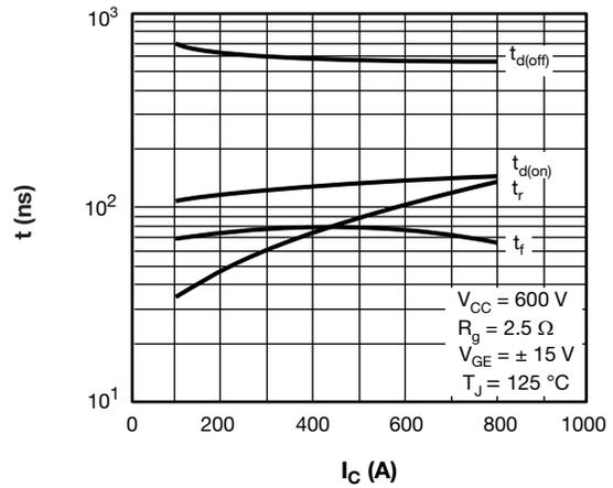
Fig. 7 - Typical Switching Time vs.  $I_C$
