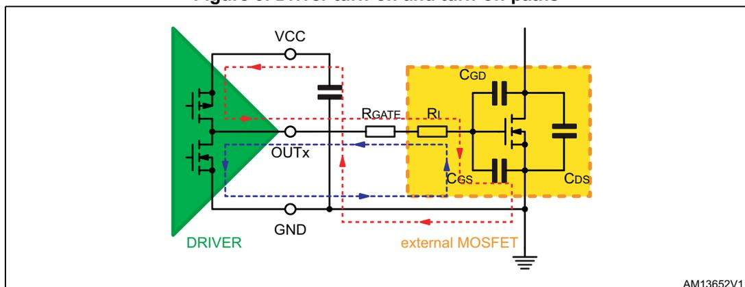
Traces between the driver and the MOSFETs should be short and wide to minimize the inductance of the traces, thus minimizing ringing in the driving signals. Moreover, the number of vias needs to be minimized in order to reduce the related parasitic effect.
