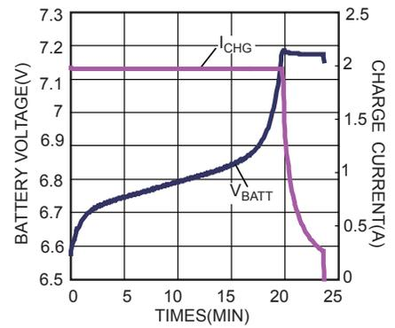
**2 Cells Charge Current vs. Battery Voltage**
