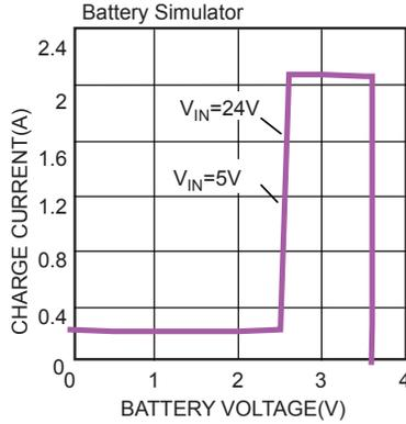
**2 Cells Battery Charge Curve**
