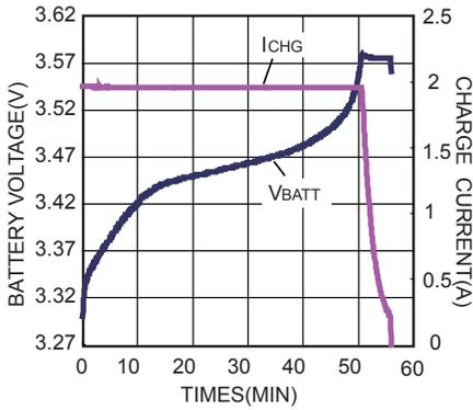
**1 Cell Charge Current vs. Battery Voltage**
