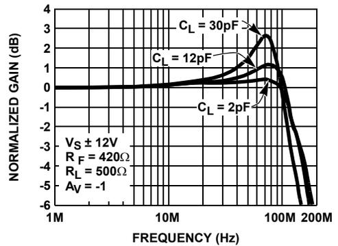
FIGURE 10. INVERTING FREQUENCY RESPONSE FOR VARIOUS  $C_L$
