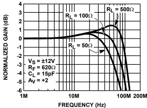
FIGURE 11. NON-INVERTING FREQUENCY RESPONSE FOR VARIOUS  $R_L$
