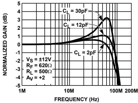
FIGURE 9. NON-INVERTING FREQUENCY RESPONSE FOR VARIOUS  $C_L$
