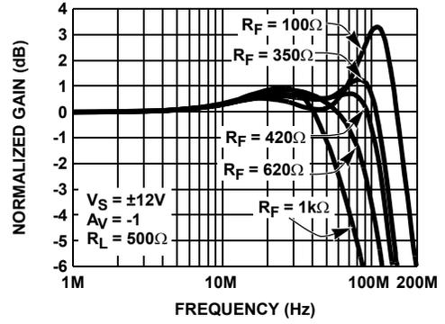
FIGURE 2. INVERTING FREQUENCY RESPONSE FOR VARIOUS  $R_F$
