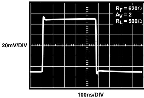
FIGURE 17. SMALL SIGNAL STEP RESPONSE ( $V_S = \pm 12V$ )
