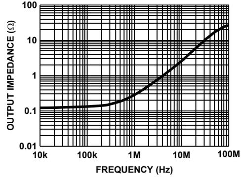
FIGURE 22. CLOSED LOOP OUTPUT IMPEDANCE vs FREQUENCY
