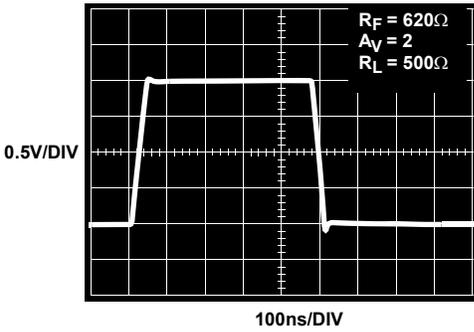
FIGURE 15. LARGE SIGNAL STEP RESPONSE ( $V_S = \pm 12V$ )
