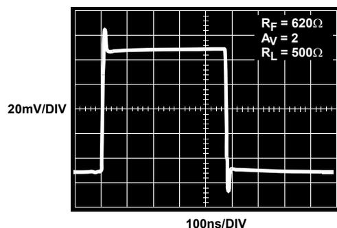
FIGURE 18. SMALL SIGNAL STEP RESPONSE ( $V_S = \pm 2.5V$ )
