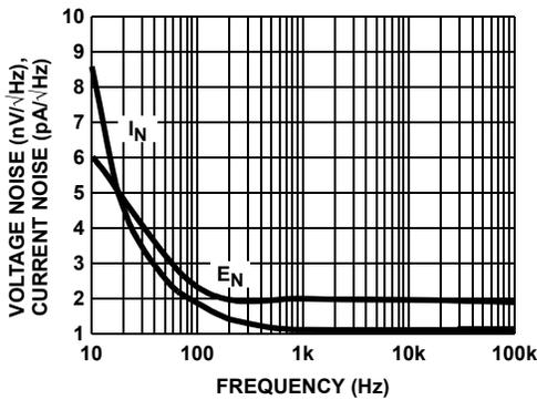
FIGURE 29. VOLTAGE AND CURRENT NOISE vs FREQUENCY
