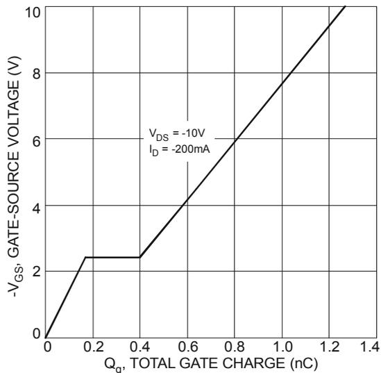
Figure 11 Gate-Charge Characteristics
