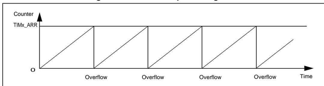
An update event can also be generated by setting the UG bit in the TIM1\_EGR register (either by software or by using the trigger controller).
