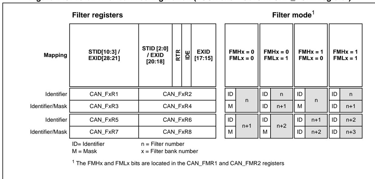
Figure 150. 16/8-bit filter bank configuration (FSCx bits = 0b01 in CAN\_FCRx register)
