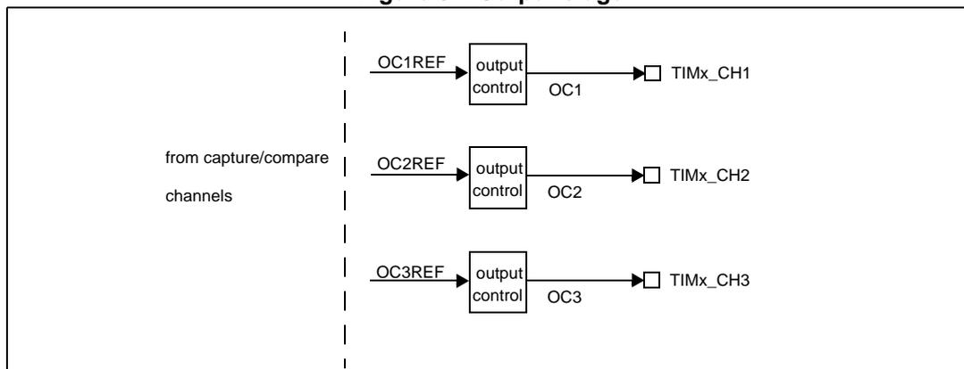
The output stage generates an intermediate waveform which is then used for reference: OCxREF (active high). Polarity acts at the end of the chain (see [Figure 88](#)).
