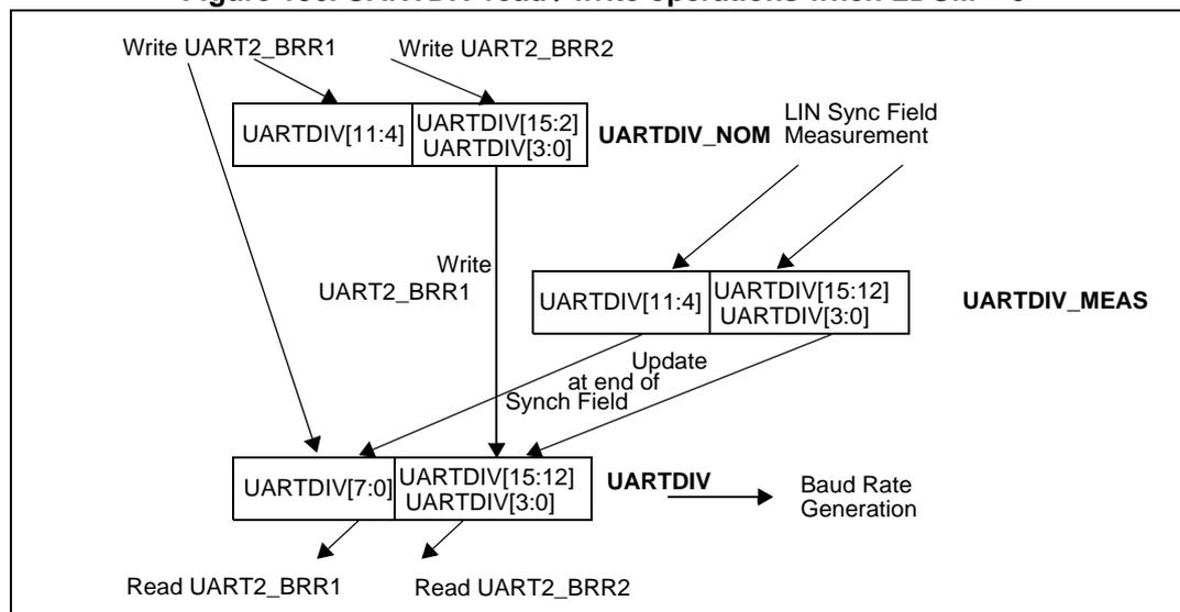
Figure 137. UARTDIV read / write operations when LDUM = 1
