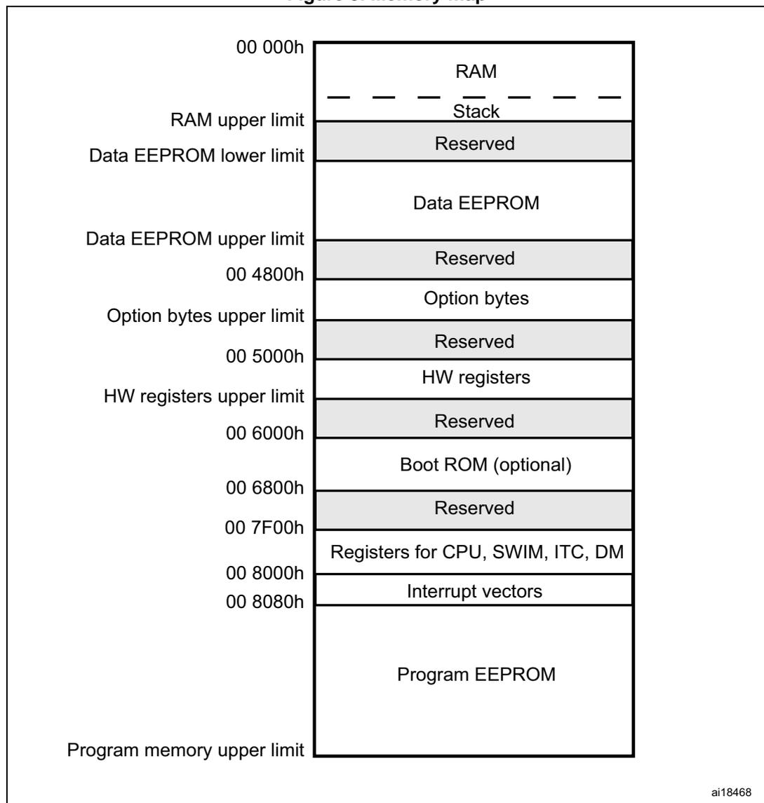
The RAM upper limit, data EEPROM upper and lower limit, Option Byte upper limit, hardware (HW) registers upper limit, and the program memory upper limit are specific to the device configuration. Please refer to the datasheets for quantitative information.
