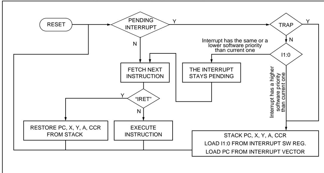
**Caution:** If the interrupt mask bits I0 and I1 are set within an interrupt service routine (ISR) with the instruction SIM, removal of the interrupt mask with RIM causes the software priority to be set to level 0.
