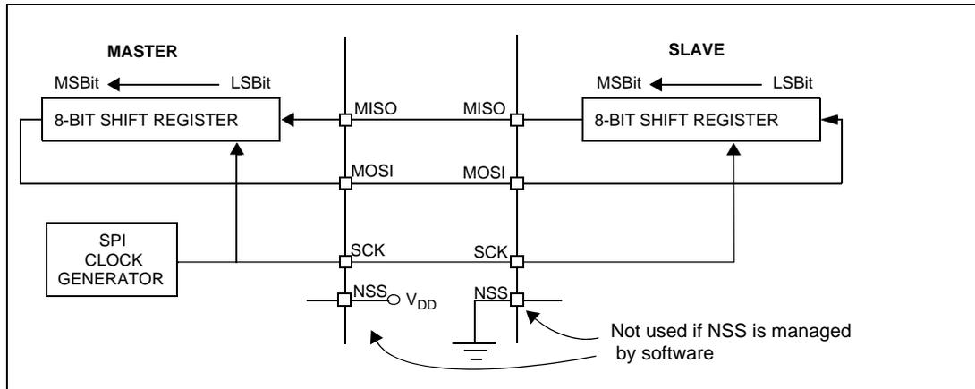
The MOSI pins are connected together and the MISO pins are connected together. In this way data is transferred serially between master and slave (most significant bit first).
