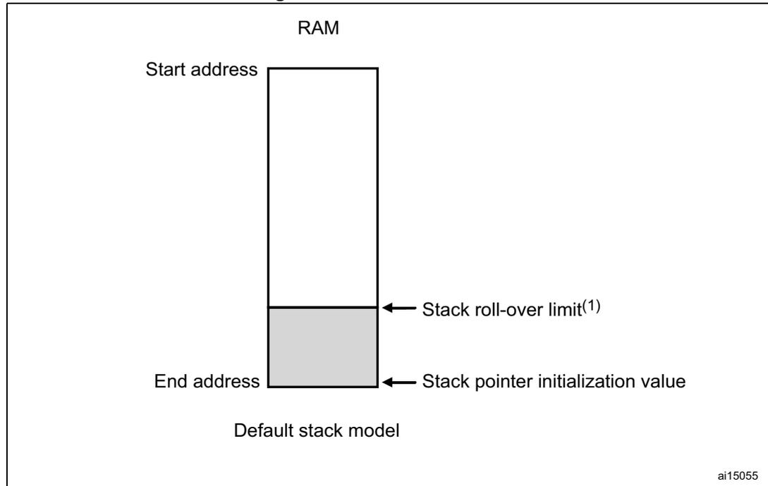
1. The stack roll-over limit is not implemented on all devices. Refer to the datasheets for detailed information.
