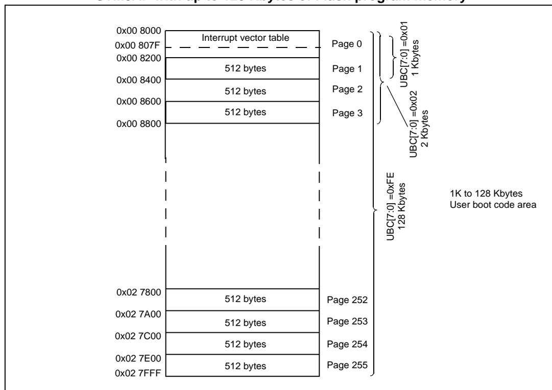
1. UBC[7:0] = 0x00 means no user boot code area is defined. Refer to the datasheets for the description of the UBC option byte.
