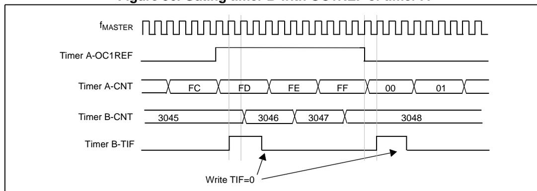
In [Figure 56](#), the timer B counter and prescaler are not initialized before being started. Therefore, they start counting from their current value. It is possible to start from a given value by resetting both timers before starting timer A. In this case, any value can be written in the timer counters. The timers can easily be reset by software using the UG bit in the TIMx\_EGR registers.
