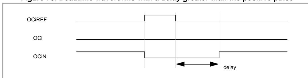
The deadtime delay is the same for each of the channels and is programmable with the DTG bits in the  $TIM1\_DTR$  register. Refer to [Section 17.7.31: Deadtime register \(TIM1\\_DTR\) on page 215](#) for delay calculation.
