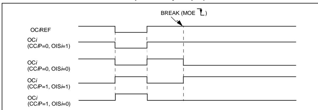
Figure 78 shows an example of behavior of the complementary outputs (TIM1 only) in response to a break.
