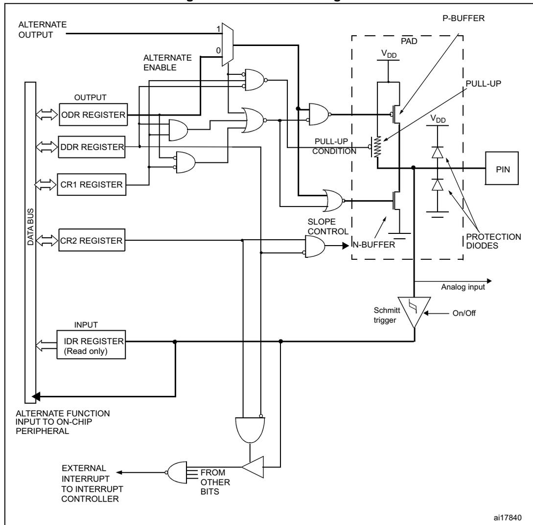
Note: The output stage is disabled when the analog input is selected.
