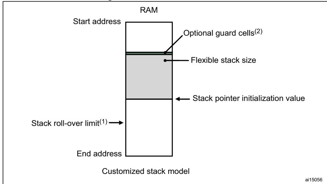
1. The stack roll-over limit is not implemented on all devices.
