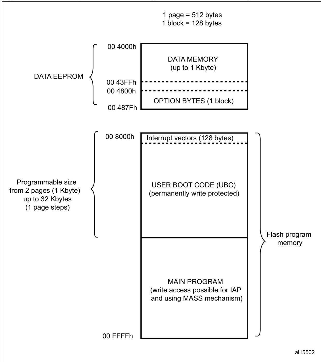
1. The memory mapping is given for the STM8AF devices featuring 32 Kbytes of Flash program memory and 1 Kbytes of SRAM.
