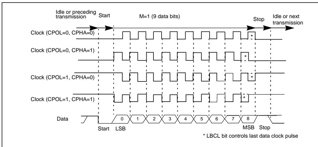
Figure 125. RX data setup/hold time
