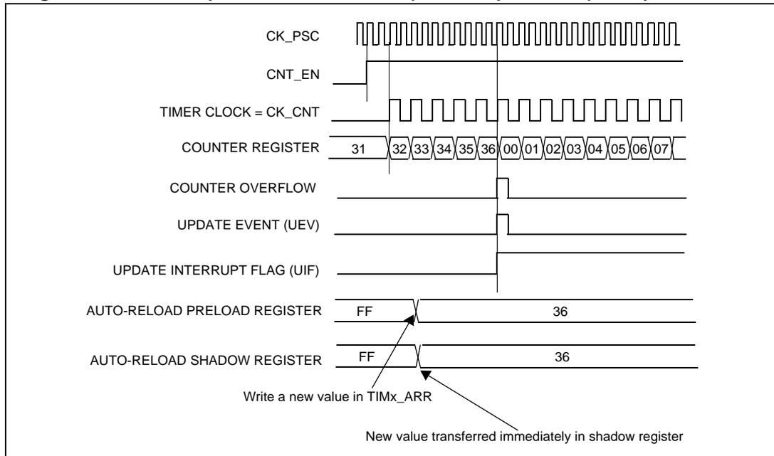
In [Figure 36](#) the prescaler divider is set to 1, so CK\_CNT has the same frequency as CK\_PSC. The auto-reload preload is enabled (ARPE = 1), so the next counter overflow occurs at 0xFF. The new auto-reload value register value of 36h is taken into account after the overflow which generates a UEV.
