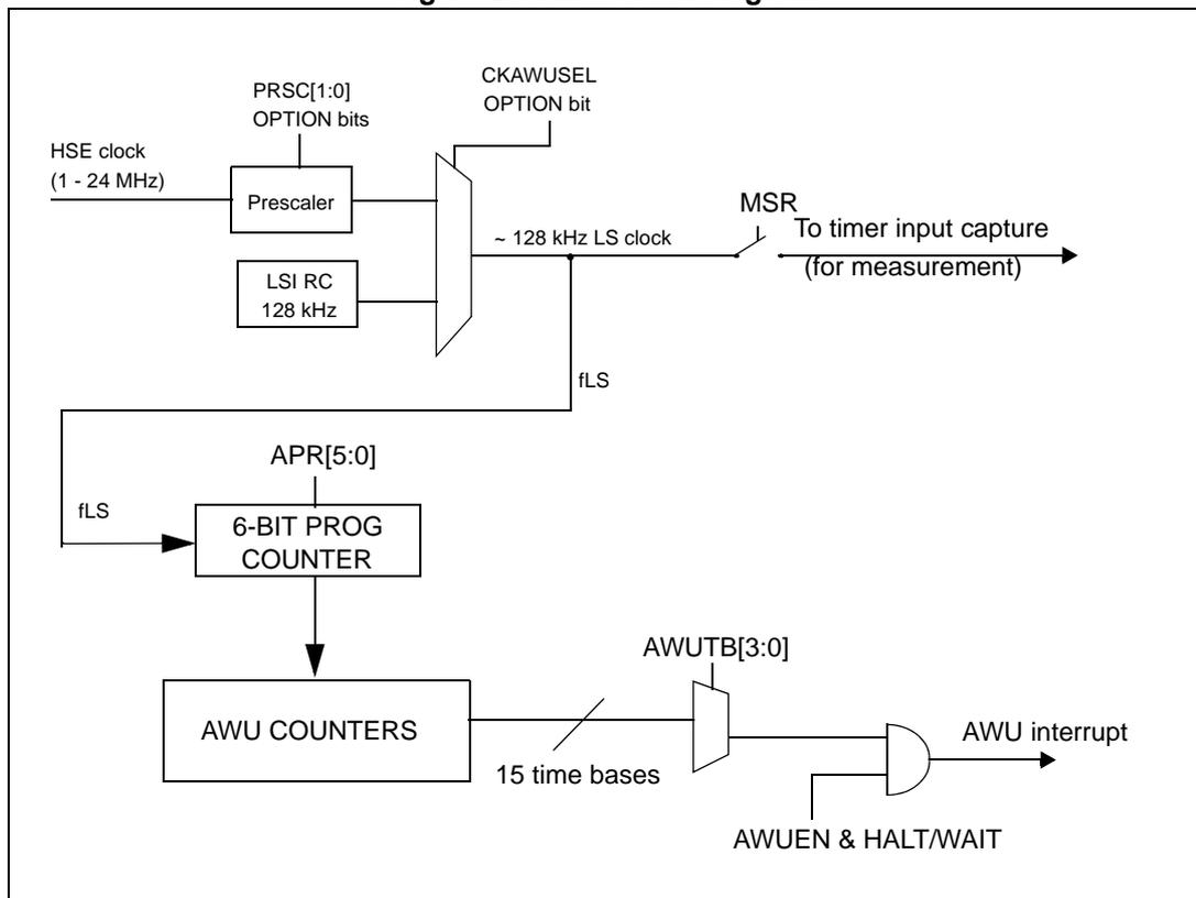
1. The LS clock source is selected by programming the CKAWUSEL option bit as explained in the clock controller chapter.
