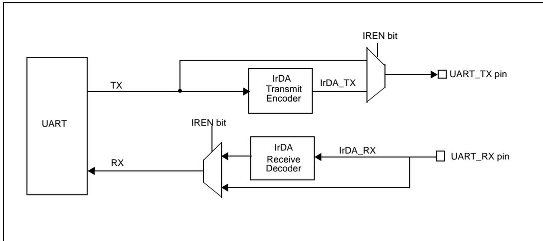
Figure 129. IrDA data modulation (3/16) - normal mode
