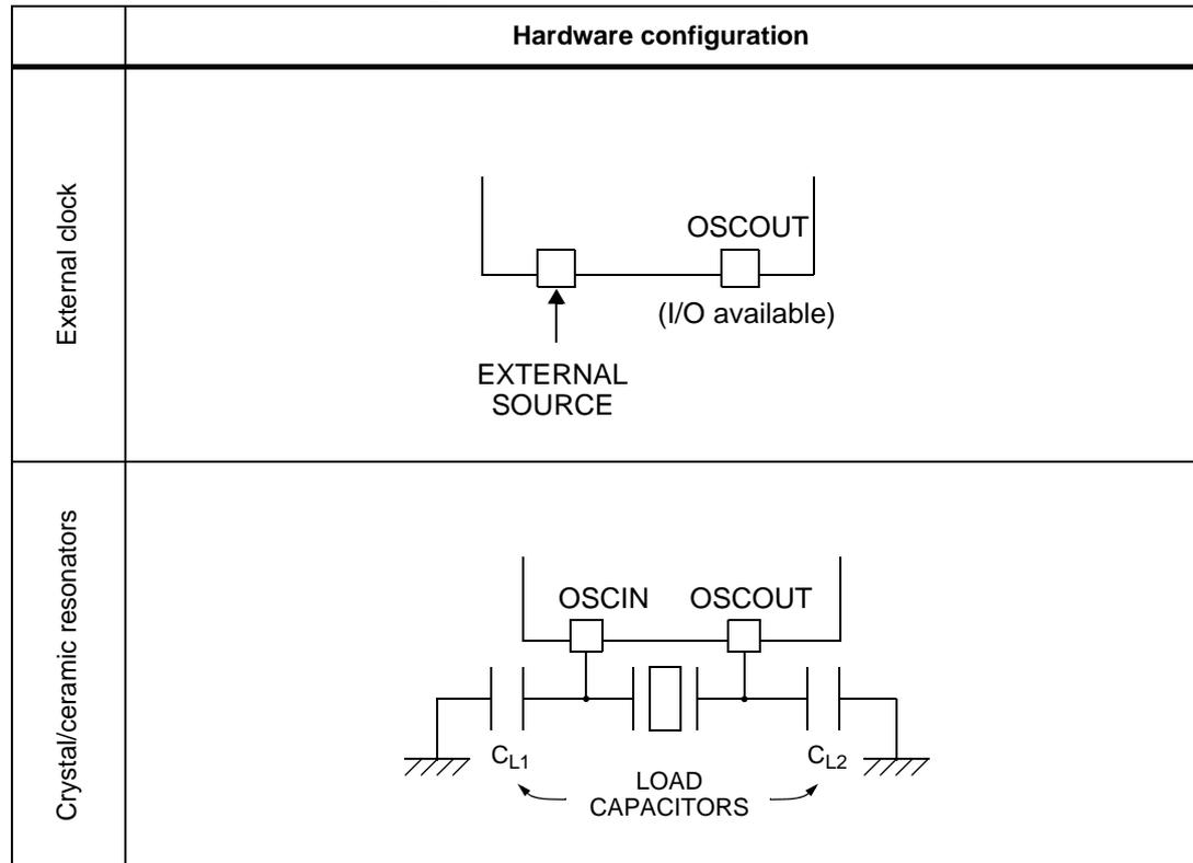
The resonator and the load capacitors have to be placed as close as possible to the oscillator pins in order to minimize output distortion and start-up stabilization time. The loading capacitance values must be adjusted according to the selected oscillator.
