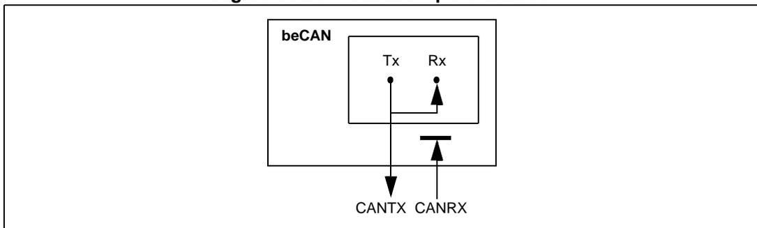
This mode is provided for self-test functions. To be independent of external events, the CAN Core ignores acknowledge errors (no dominant bit sampled in the acknowledge slot of a data / remote frame) in Loop Back Mode. In this mode, the beCAN performs an internal feedback from its Tx output to its Rx input. The actual value of the CANRX input pin is disregarded by the beCAN. The transmitted messages can be monitored on the CANTX pin.
