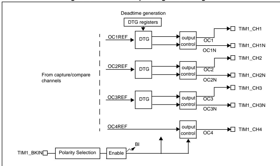
Figure 68. Detailed output stage of channel with complementary output (channel 1)
