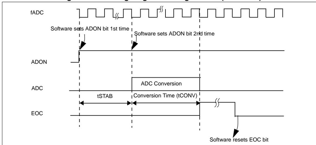
Figure 163. Timing diagram in continuous mode (CONT = 1)
