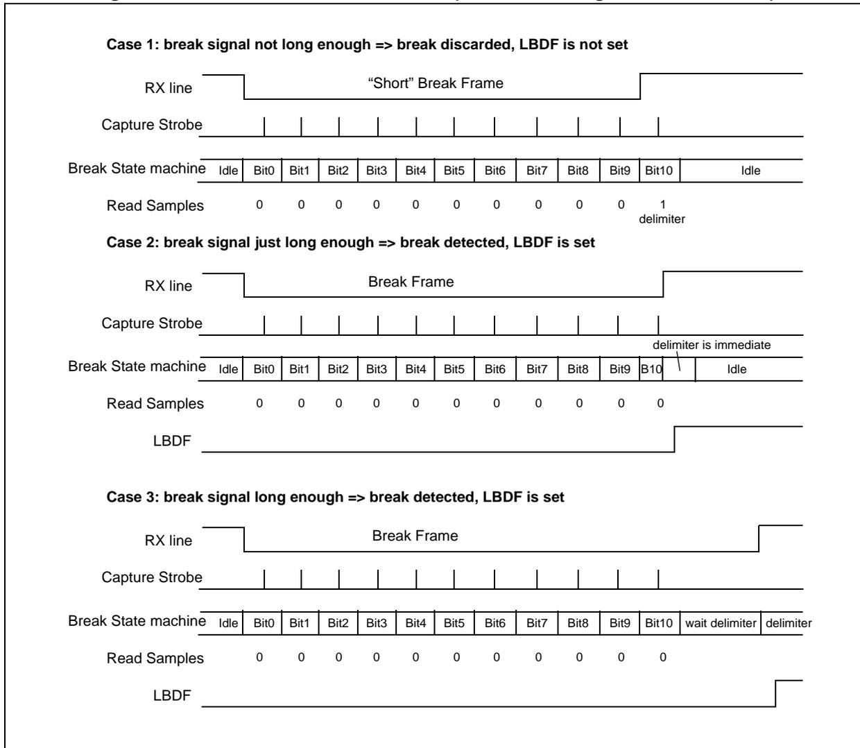
**Figure 131. Break detection in LIN mode vs framing error detection**
