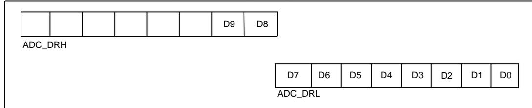
**Left Alignment:** 8 Most Significant bits are written in the ADC\_DH register, then the remaining Least Significant bits are written in the ADC\_DL register. The Most Significant Byte must be read first followed by the Least Significant Byte.
