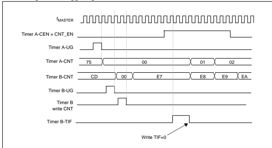
**Starting 2 timers synchronously in response to an external trigger**
