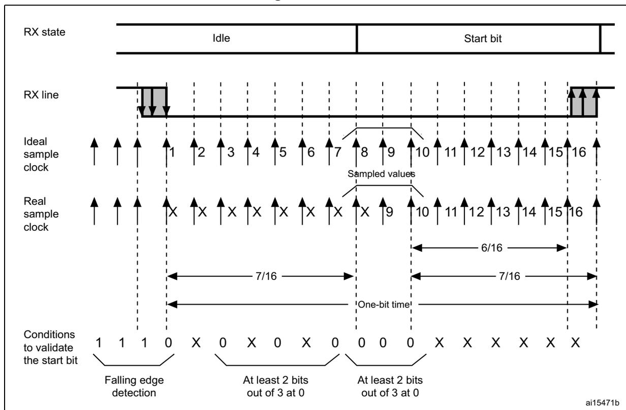
**Note:** If the sequence is not complete, the start bit detection aborts and the receiver returns to the idle state (no flag is set), where it waits for a falling edge.
