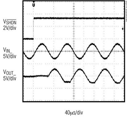
OUTPUT AT 2V<sub>RMS</sub> AT 1kHz
