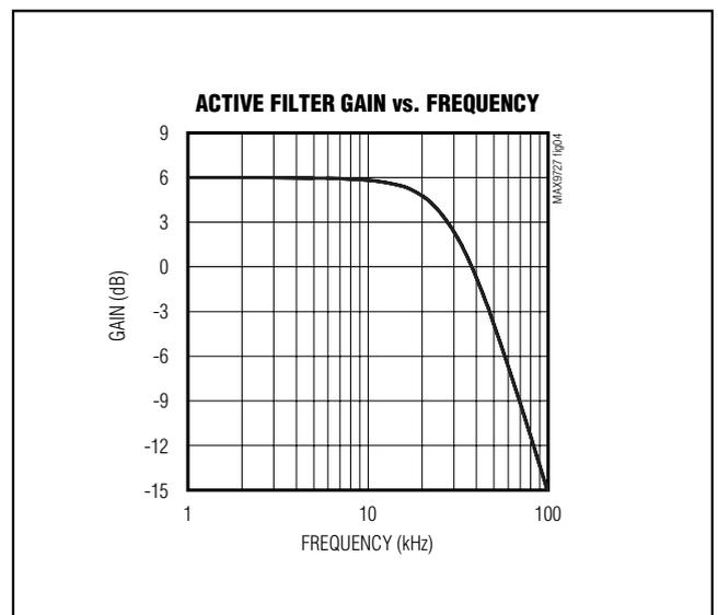
Figure 4. MAX9727 Active Filter Gain vs. Frequency
