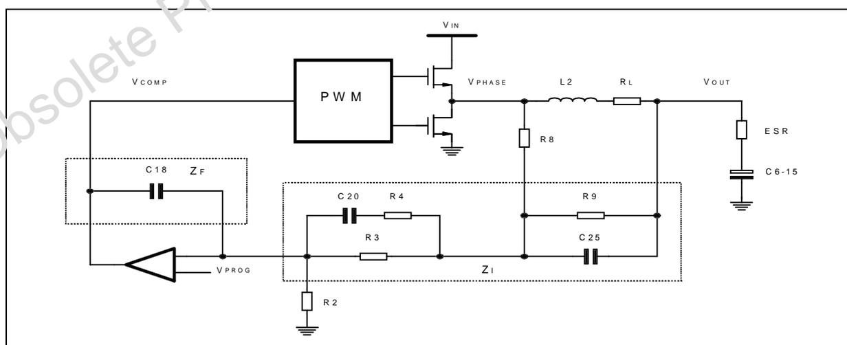
Considering the previous relationships  $R_2$ ,  $R_3$ ,  $R_8$  and  $R_9$  may be determined in order to obtain the desired droop effect as follow:
