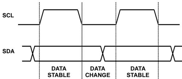
FIGURE 9. VALID DATA CHANGES ON I<sup>2</sup>C BUS
