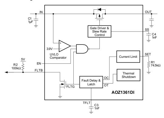
Figure 2. AOZ1361DI Functional Block Diagram
