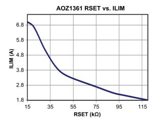
Figure 3. Current Limit vs. RSET ( $V_{IN} = 12V$ )
