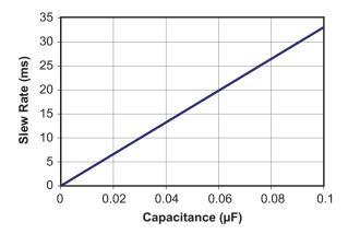
Figure 4. Output Slew Rate Adjustment vs. Capacitance
