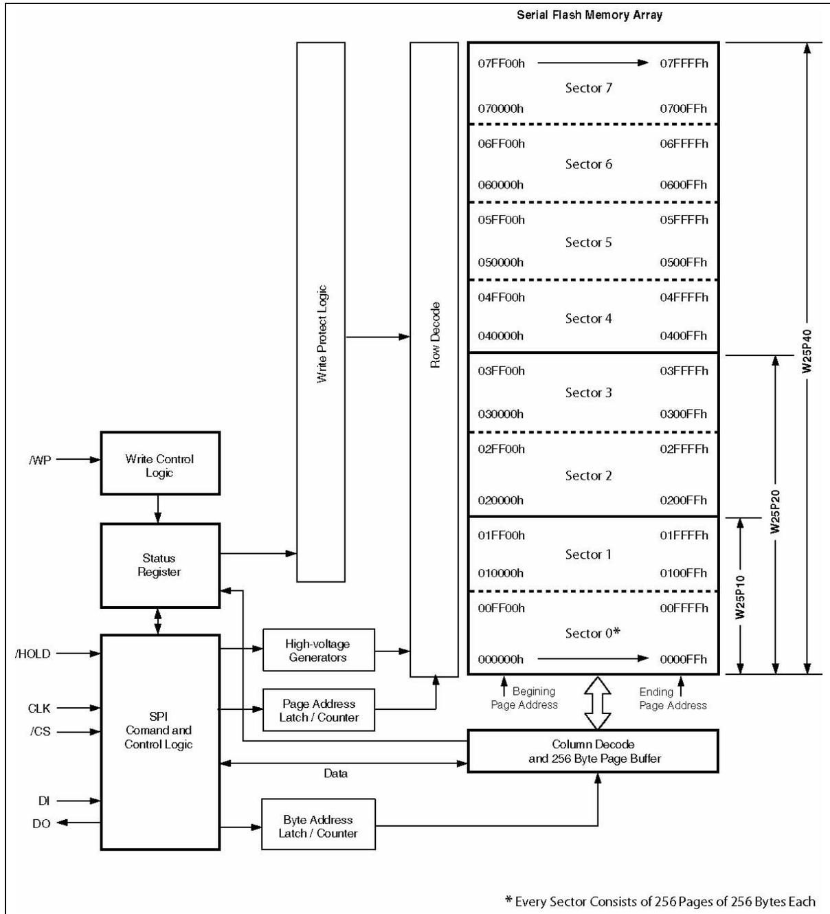
Figure 2. W25P10, W25P20 and W25P40 Block Diagram
