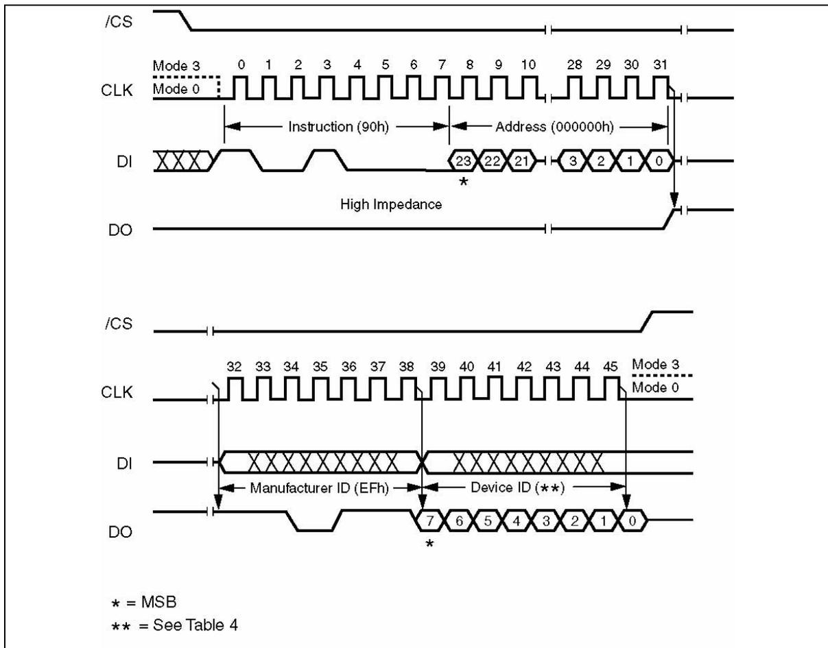
Figure 16. Read Manufacturer / Device ID Diagram
