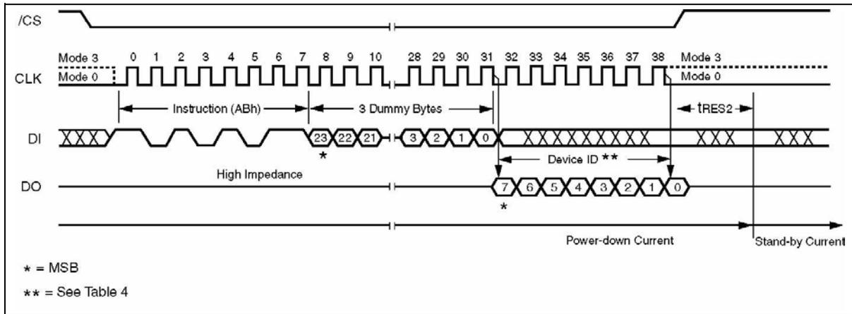
Figure 15. Release Power-down / Device ID Instruction Sequence Diagram
