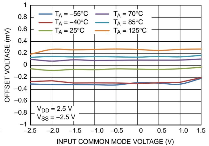
Figure 11.  $V_{OS}$  vs.  $V_{CM}$  ( $V_S = 5 V$ )
