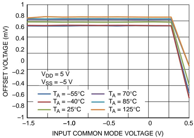
Figure 12.  $V_{OS}$  vs.  $V_{CM}$  ( $V_S = 10\text{ V}$ )
