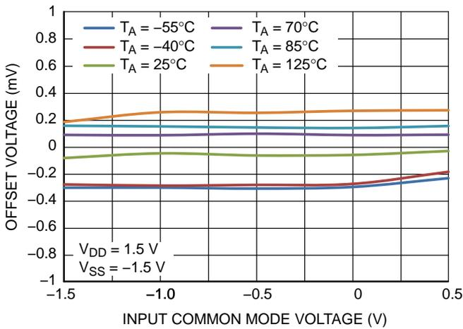
Figure 10.  $V_{OS}$  vs.  $V_{CM}$  ( $V_S = 3 V$ )
