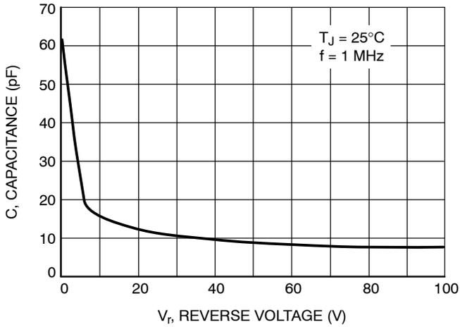
Figure 5. Typical Capacitance
