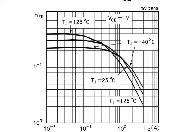
Figure 3. DC current gain ( $V_{CE} = 5\text{ V}$ )
