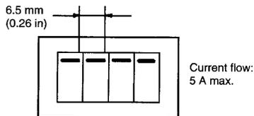
More than two relays can be closely mounted upside down as shown in the illustration below.
