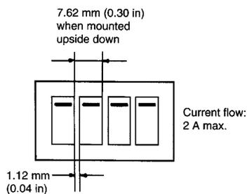
Note: The space between each relay required for heat radiation may vary with operating conditions.
