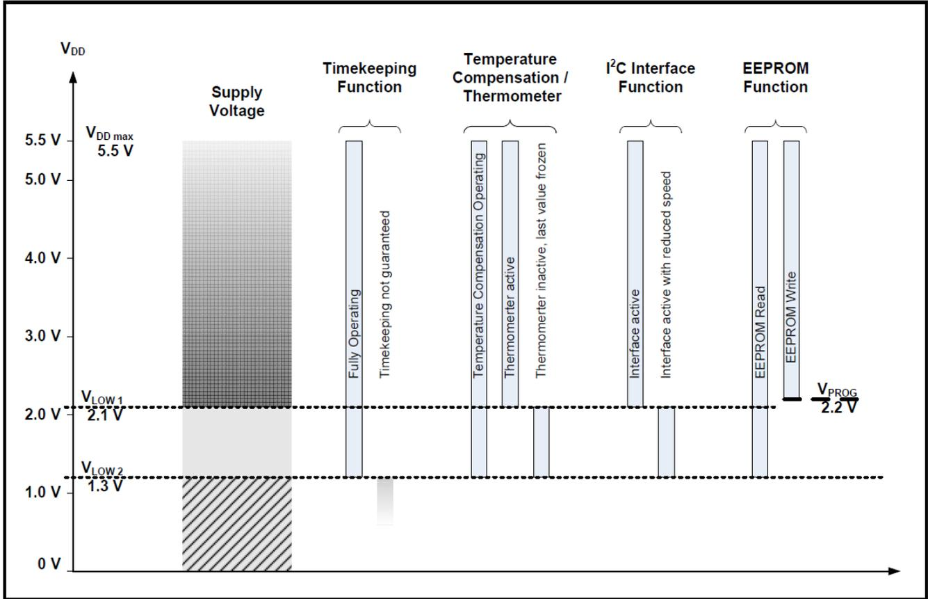
At first power-up, the supply voltage has to exceed  $V_{LOW1}$  threshold to enable and correctly setup all function of the device.
