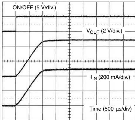
SiP4280-1 Turn-On ( $V_{IN} = 5\text{ V}$ ,  $R_{LOAD} = 10\ \Omega$ )
