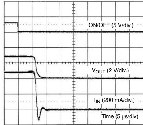
SiP4280-1 Turn-Off ( $V_{IN} = 3\text{ V}$ ,  $R_{LOAD} = 6\ \Omega$ )
