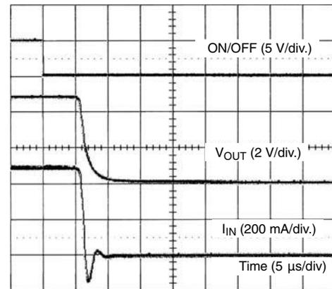
SiP4280-1 Turn-Off ( $V_{IN} = 5\text{ V}$ ,  $R_{LOAD} = 10\ \Omega$ )
