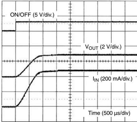
SiP4280-1 Turn-On ( $V_{IN} = 3\text{ V}$ ,  $R_{LOAD} = 6\ \Omega$ )
