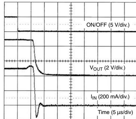
SiP4280-3 Turn-Off ( $V_{IN} = 5\text{ V}$ ,  $R_{LOAD} = 10\ \Omega$ )
