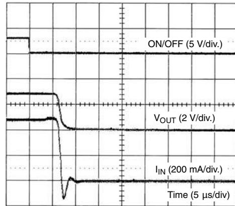
SiP4280-3 Turn-Off ( $V_{IN} = 3\text{ V}$ ,  $R_{LOAD} = 6\ \Omega$ )
