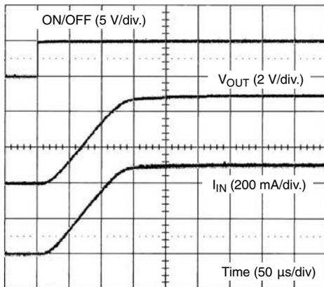
SiP4280-3 Turn-On ( $V_{IN} = 5\text{ V}$ ,  $R_{LOAD} = 10\ \Omega$ )
