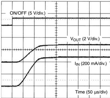
SiP4280-3 Turn-On ( $V_{IN} = 3\text{ V}$ ,  $R_{LOAD} = 6\ \Omega$ )
