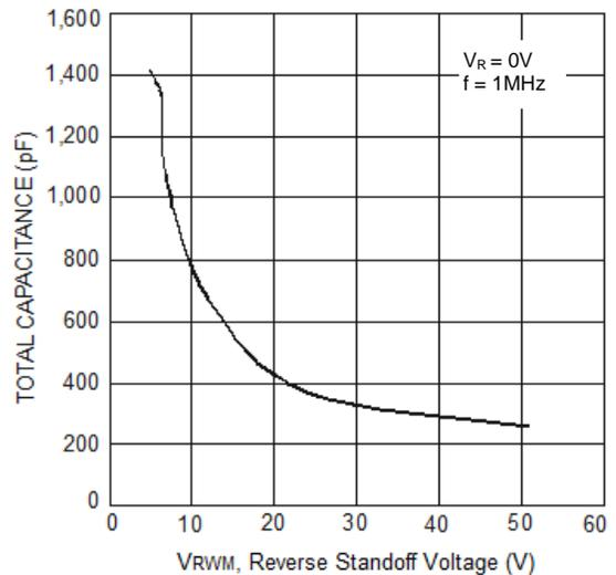
Fig. 6 Total Capacitance vs Reverse Standoff Voltage
