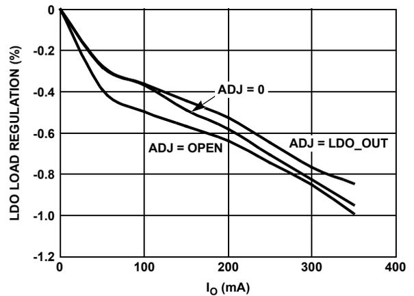
FIGURE 6. LDO LOAD REGULATION vs I<sub>O</sub>
