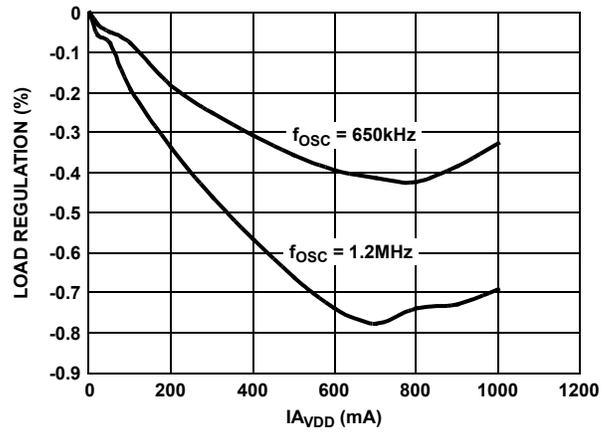
FIGURE 2. A<sub>VDD</sub> LOAD REGULATION vs I<sub>A\_VDD</sub>
