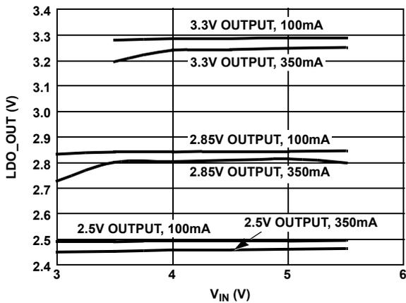
FIGURE 5. LINE REGULATION LDO\_OUT vs V<sub>IN</sub>
