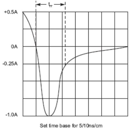
Fig. 5 Reverse Recovery Time Characteristic and Test Circuit
