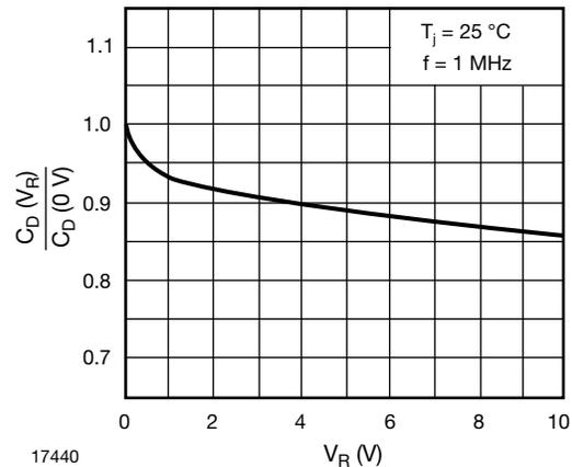
Fig. 4 - Relative Capacitance vs. Reverse Voltage
