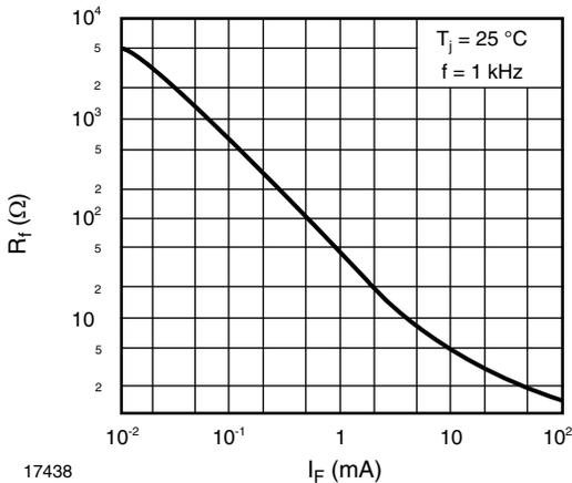
Fig. 2 - Dynamic Forward Resistance vs. Forward Current
