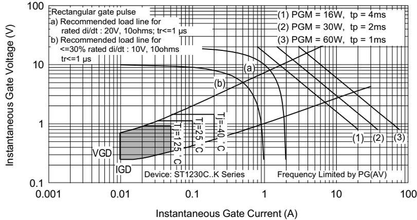
Fig. 11 - Gate Characteristics
