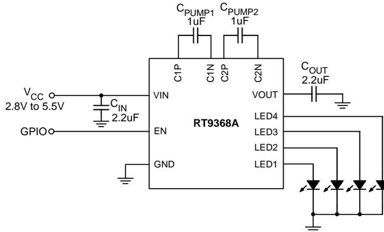
Figure 1. For 4-WLEDs Application Circuit
