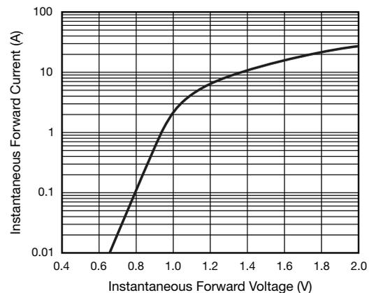
Fig. 2 - Typical Instantaneous Forward Characteristics Per Diode
