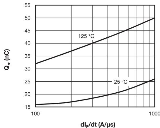
Fig. 7 - Typical Stored Charge vs.  $dI_F/dt$
