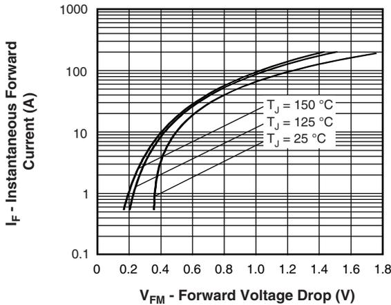
Fig. 1 - Maximum Forward Voltage Drop Characteristics
