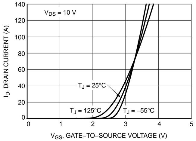
Figure 2. Transfer Characteristics
