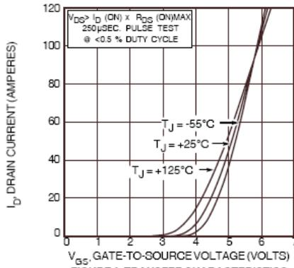
FIGURE 4. TRANSFER CHARACTERISTICS
