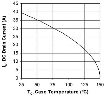
Figure 6, DC Drain Current vs Case Temperature
