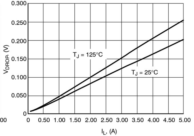
Figure 3.  $V_{DROP}$  vs.  $I_L$  @  $V_{IN} = 4.5$  V
