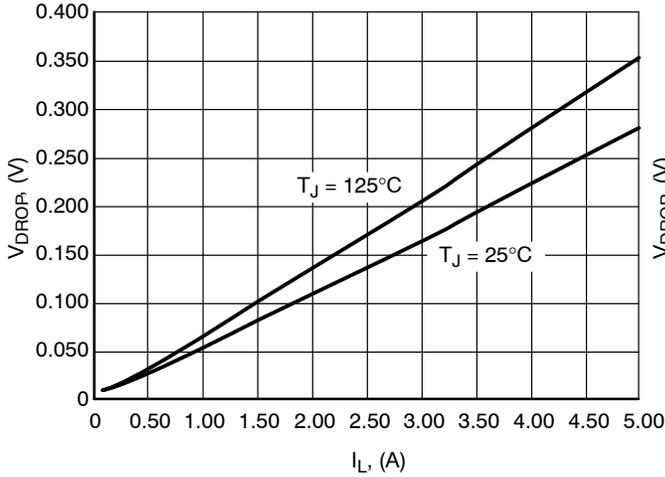
Figure 2.  $V_{DROP}$  vs.  $I_L$  @  $V_{IN} = 2.5$  V
