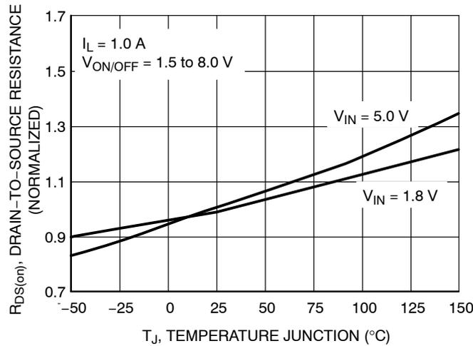
Figure 6. Normalized On Resistance Variation with Temperature
