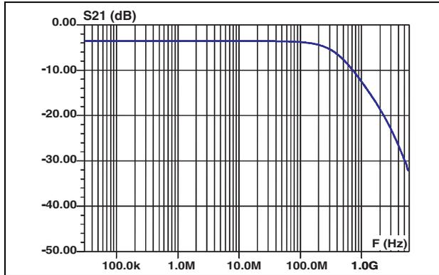
Figure 5. S21 (dB) analog crosstalk measurements C3 - A1
