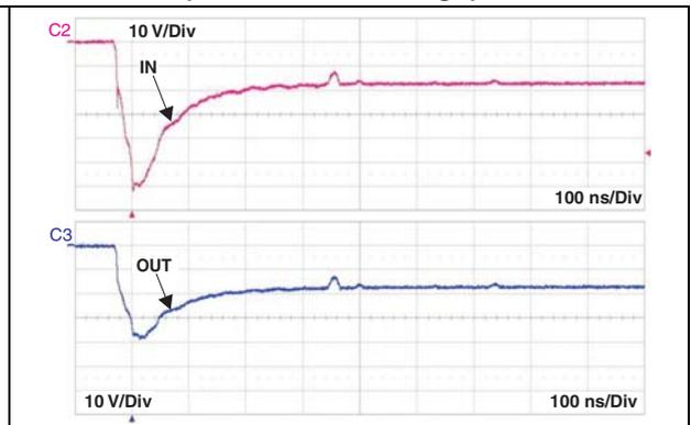
Figure 8. Digital crosstalk measurement
