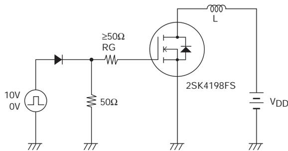
Fig.2 Switching Time Test Circuit
