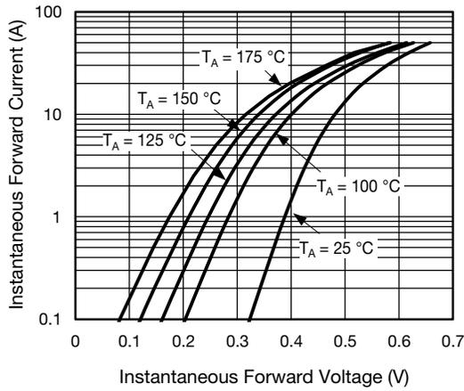
Fig. 3 - Typical Instantaneous Forward Characteristics Per Diode
