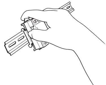
To remove the Relay from the DIN Track, pull down on the tab with a screwdriver in the direction of the arrow.
