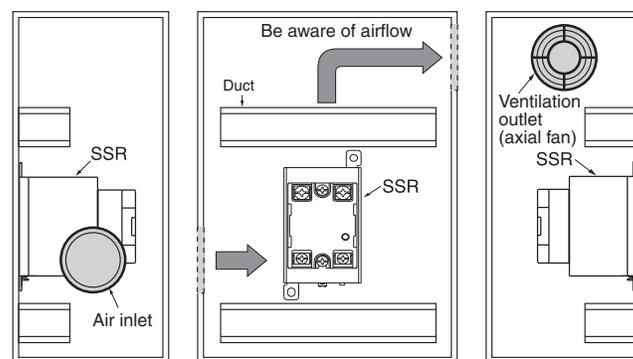
If the air inlet or air outlet has a filter, clean the filter regularly to prevent it from clogging to ensure an efficient flow of air.
