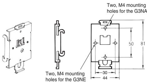
To mount the Relay to DIN Track, first mount it to the One-touch Mounting Plate and then attach it to the DIN Track as shown in the diagram.
