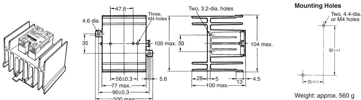
**Y92B-P250N (for max. 50 A load current)**
