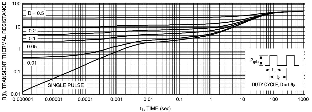
Figure 8. Thermal Response Junction-to-Ambient for MBR30H150CTG
