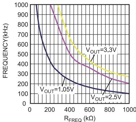
NB6381 is optimized to operate at high switching frequency with high efficiency. High switching frequency makes it possible to utilize small sized LC filter components to save system PCB space.
