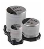
Type AVES Capacitors are rated for 1000 hours at 105 °C with low impedance characteristics. They are ideal for high density PC board packaging. The Type AVES offers a low in-place-cost for a high quality performer. The vertical cylindrical cases facilitate automatic mounting and reflow soldering into the same footprint of like-rated tantalum capacitors except without the need for voltage derating. Type AVES is RoHS compliant.
