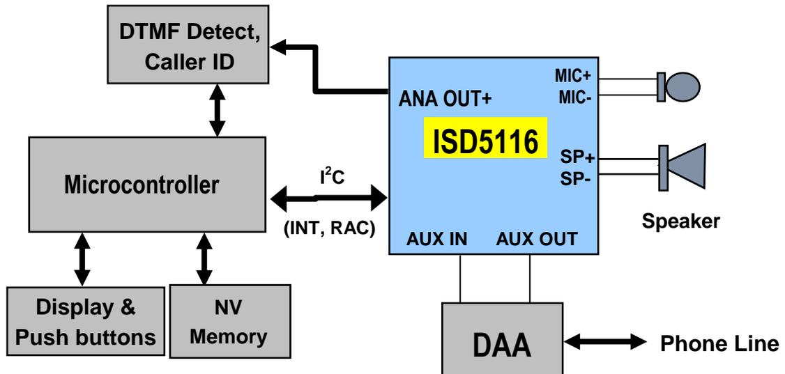
For duplex recording, speech from Mic inputs and message from received path can be directly recorded into the array simultaneously, then playback afterwards. In addition, for speaker phone
