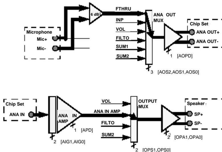
The figure above shows the part of the ISD5100 Series block diagram that is used in Feed Through Mode. The rest of the chip will be powered down to conserve power. The bold lines highlight the audio paths. Note that the Microphone to ANA OUT +/- path is differential.
