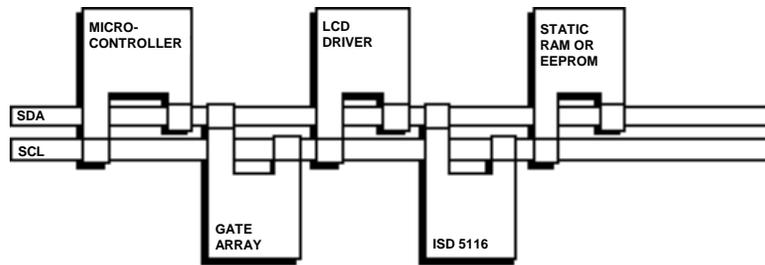
Example of an I<sup>2</sup>C-bus configuration using two microcontrollers
