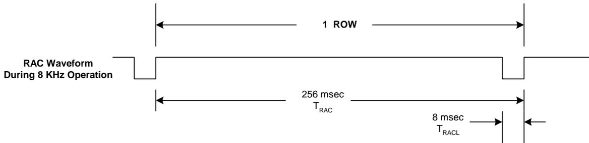
The RAC pin remains HIGH for 500 μsec and stays LOW for 15.6 μsec under the Message Cueing mode. See the [Timing Parameters table](#) on page 64 for RAC timing information at other sample rates. When a record command is first initiated, the RAC pin remains HIGH for an extra T<sub>RACML</sub> period, to load sample and hold circuits internal to the device. The RAC pin can be used for message management techniques.
