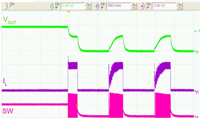
**Figure 35. Over-Current Fault Response,  $R_{LOAD} = 1\ \Omega$ ,  $50\ \mu\text{s/div.}$**
