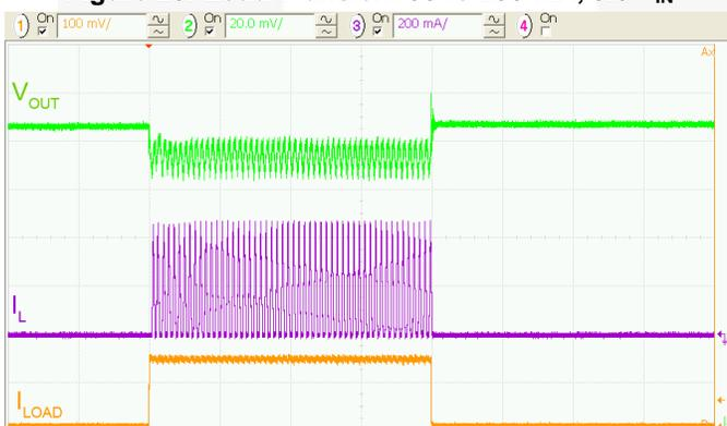
Figure 30. Load Transient 0 to 150 mA, 4.5  $V_{IN}$
