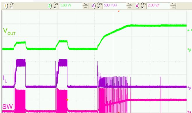
**Figure 37. Overload Recovery to Light Load,  $50\ \mu\text{s/div.}$**
