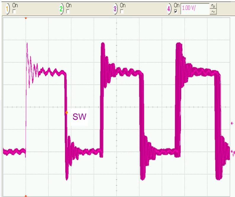
**Figure 39. SW-Node Jitter (Infinite Persistence),  $I_{LOAD} = 200\text{ mA}$ , 50 ns/div.**
