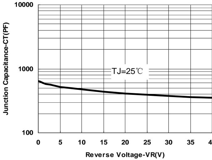
Fig.1-Typical Junction Capacitance
