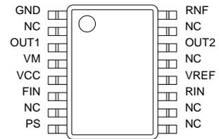
Fig.30 BA6285FS (SSOP-A16)
